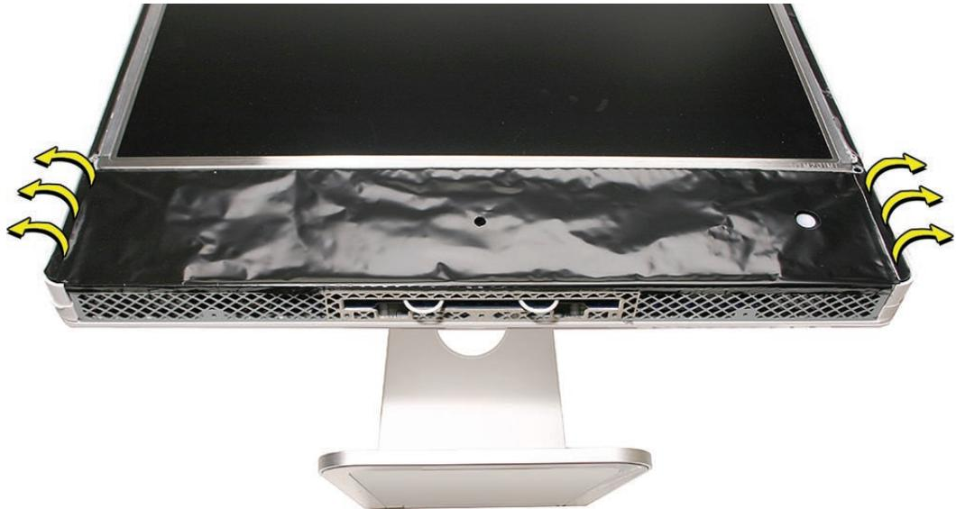
2. Peel the bottom of the EMI shield off the frame.
