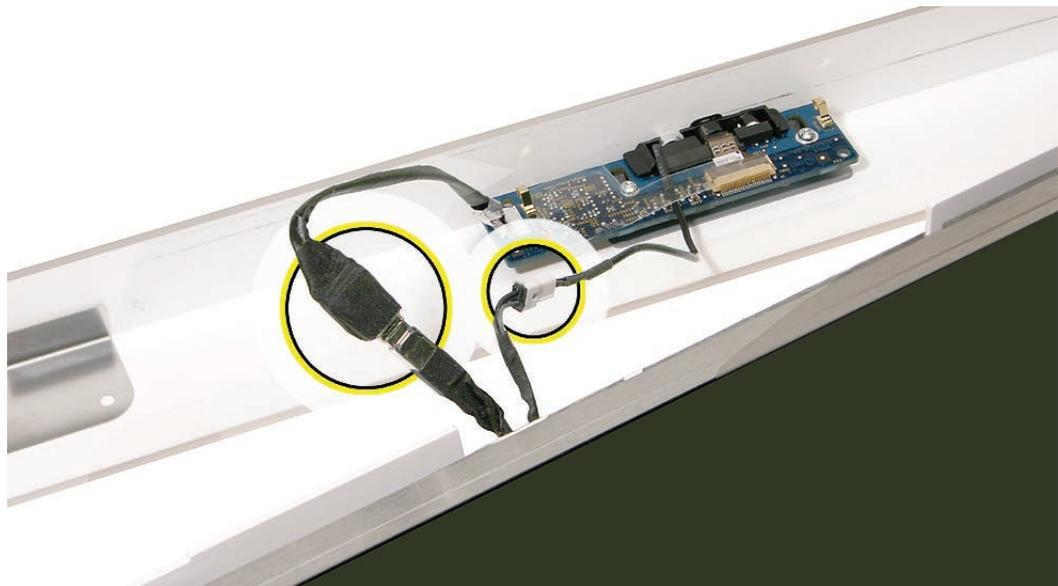
12. Lift the front bezel off the computer. **Note** the microphone is part of the front bezel assembly.
