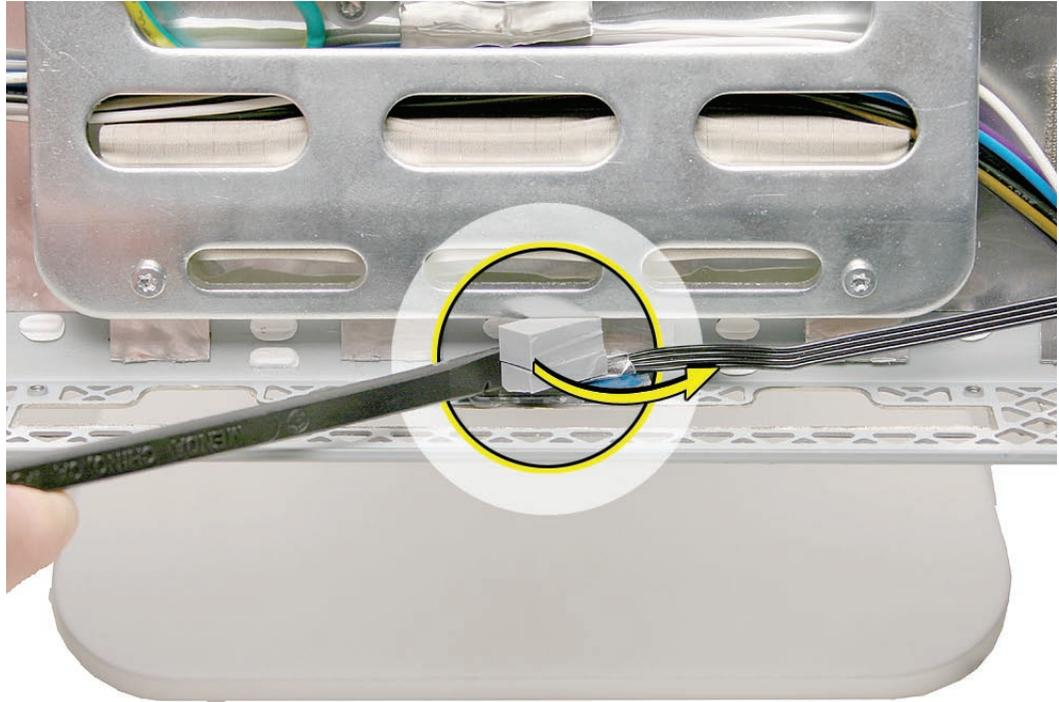
2. Using a black stick, pry the ambient light sensor off the inside of the rear housing. The sensor is stuck to the rear housing with double-stick tape. **Note:** never poke the ambient light or you could damage the sensor board.
