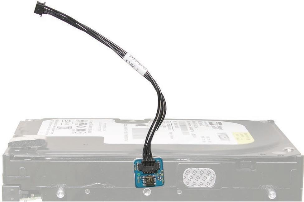
2. Attach the mounting bracket and pins if they were removed. Connect the hard drive data and power cables.
