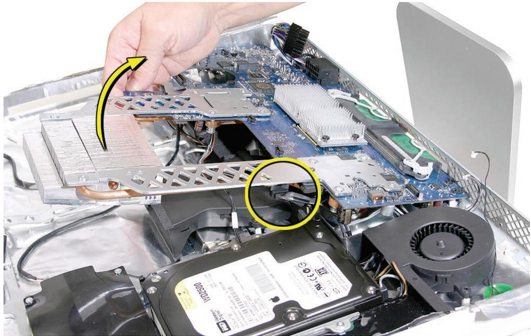
8. Holding the board by the sides, lift it up and toward the top of the computer. **Note:** Remove the memory module from the slot before returning the board to Apple.
