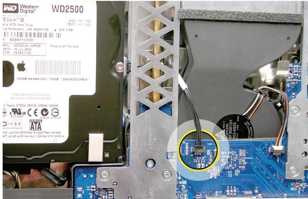
4. Insert the hard drive pins into the grommets. Lower the drive into the rear housing.
