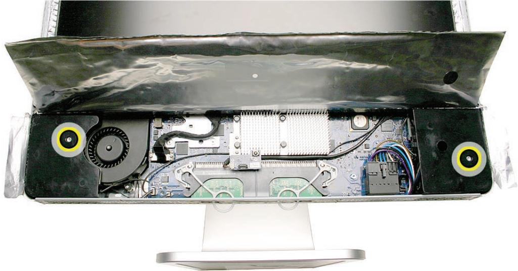
2. Using a T6 torx screwdriver, remove the screw that secures the IR board to the IR mounting bracket. Disconnect the IR cable from the IR board.
