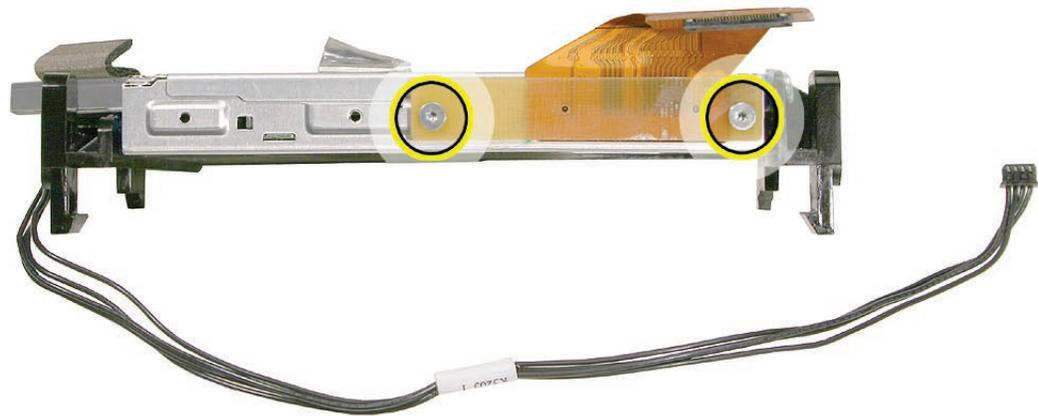
7. If replacing the optical drive, disconnect the sensor cable from the optical sensor located on the underside of the optical drive. Transfer the sensor cable to the replacement drive.
