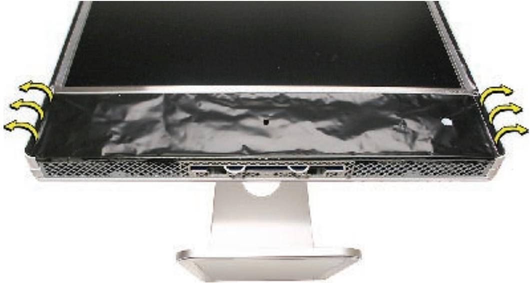
2. Carefully peel the lower EMI shield off the bottom edge of the rear housing. Use a black stick to help peel back the shield.
