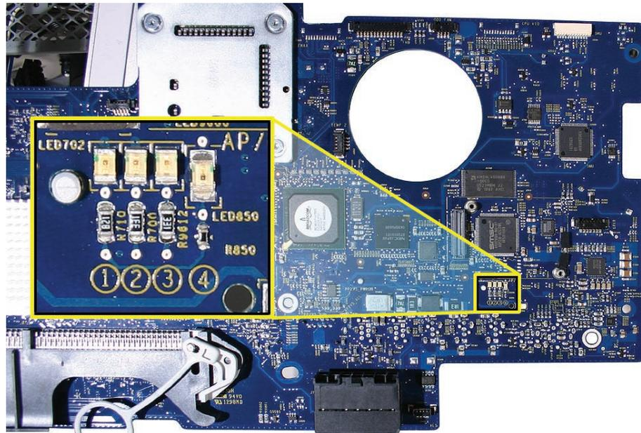
**LED #1 is On:** This indicates that the AC power inlet and AC-to-DC power supply is getting good power from the AC outlet, and the DC-to-DC board is receiving 12VDC. Go to step 8.
