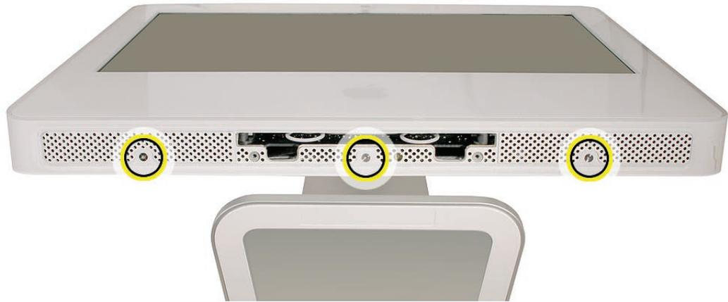
3. Slightly bending the upper quarter of the access tool card will help engage the latch more securely. Refer to the Access Tool Modification if the bezel is difficult to remove.
