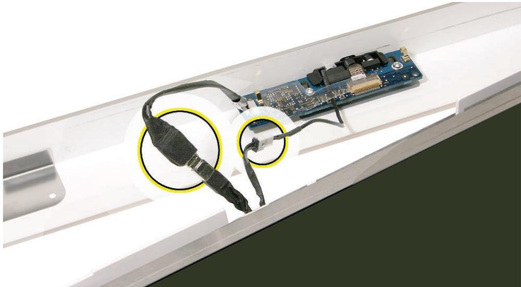
3. Remove the two T6 screws on the camera board.
