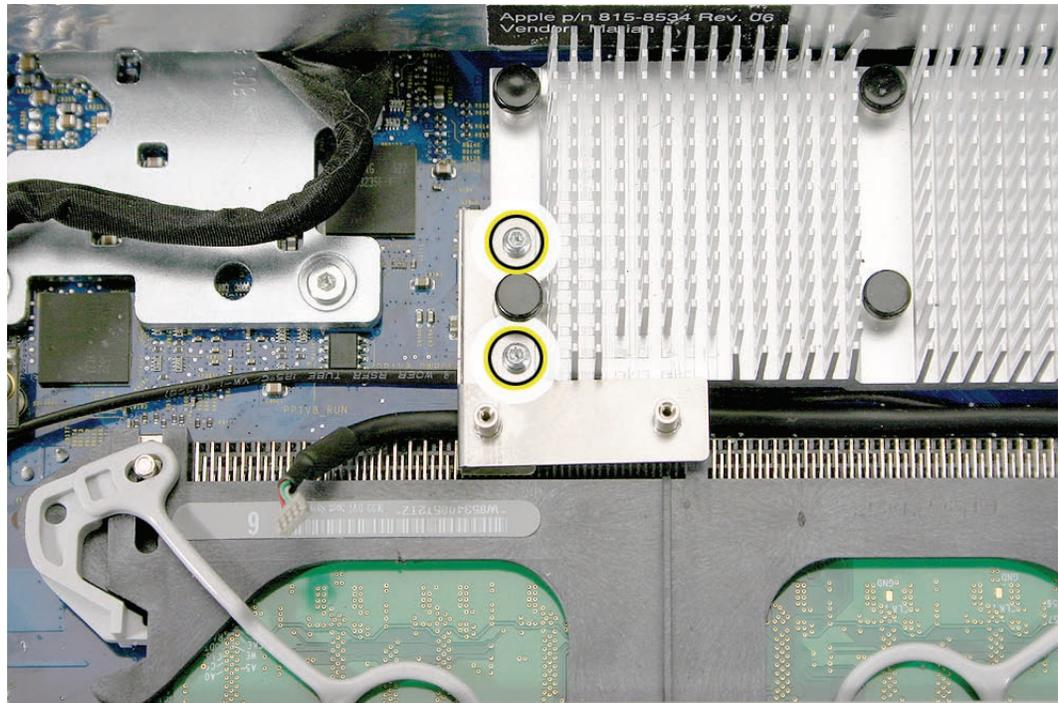
3. Replace the IR board onto the mounting bracket. Connect the cable and replace the two T6 screws.
