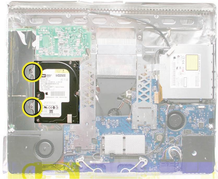
2. Disconnect the hard drive sensor cable from the connector on the logic board. **Note** the location of the sensor on the side of the hard drive and the routing of the cable.
