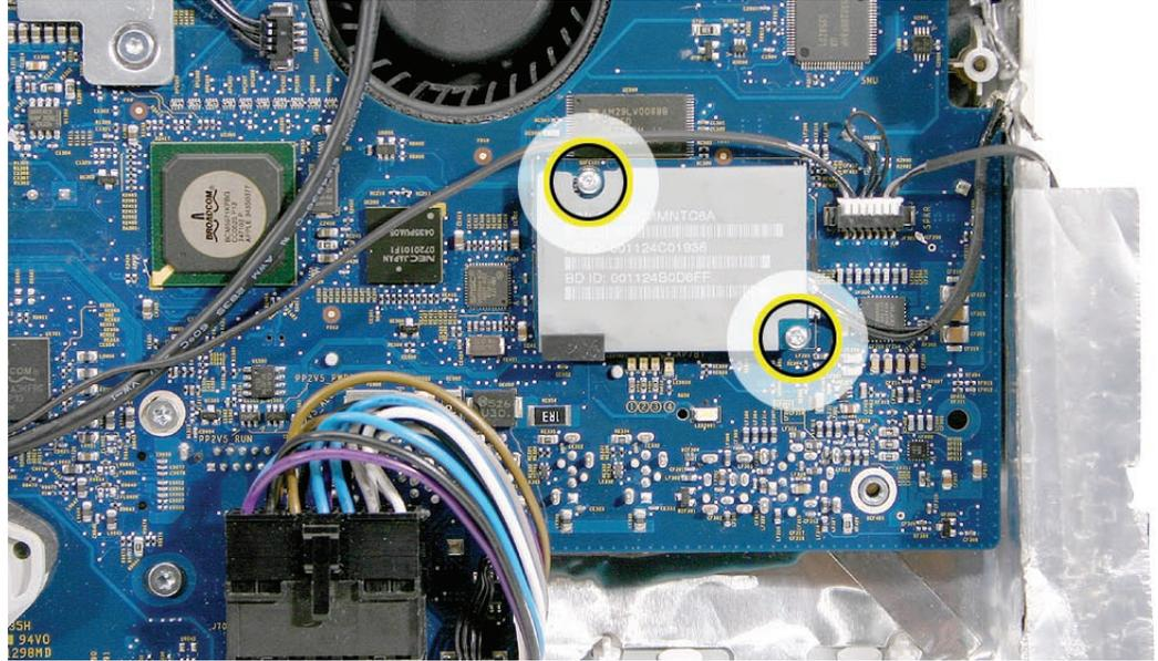
2. Disconnect the two antenna cables from the AirPort Extreme/Bluetooth card.
