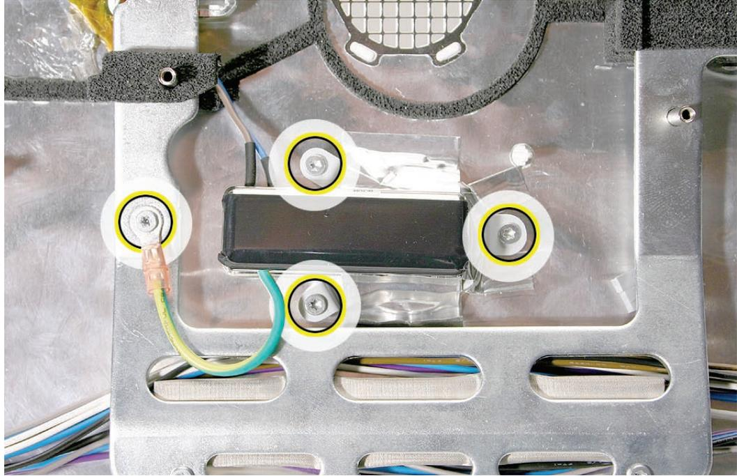
2. Carefully peel up the EMI tape on the AC filter; peel off both the large and small EMI pieces of tape. Set them aside.
