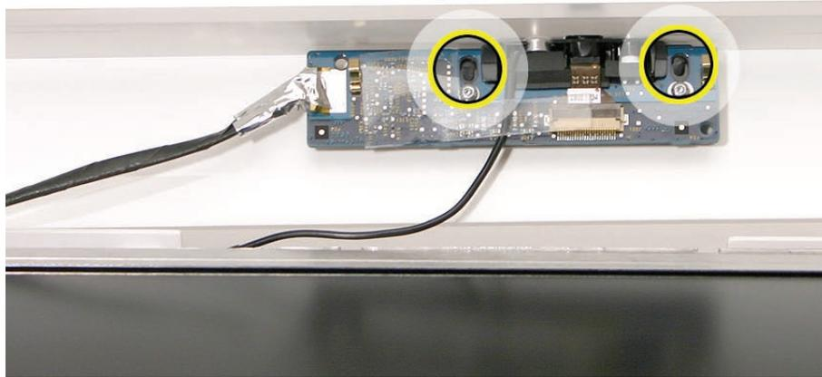
3. Connect the camera and microphone cables.
