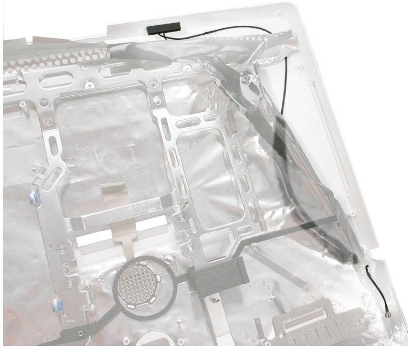
3. Route the antenna cable as shown above and insert the connector's end of the cable through the access hole in the Faraday shield. Leave about 2 inches of cable extending from the Faraday shield.
