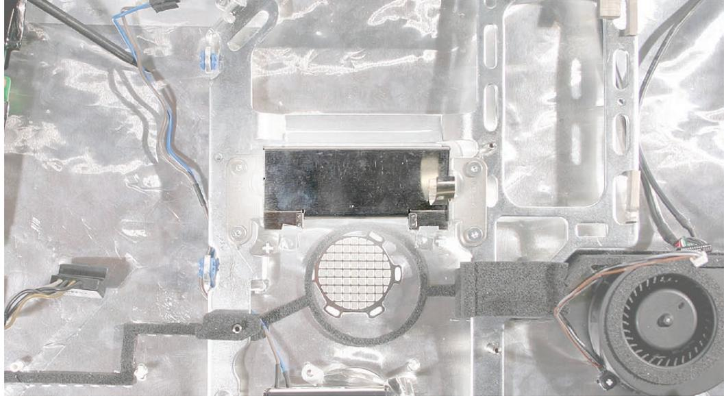
2. Peel back the EMI tape on top of the mechanism. Using a torx T10 screwdriver, remove the four clutch mounting screws.
