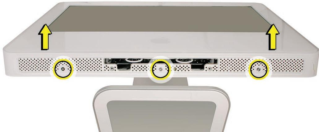
6. Stand up the unit. Using the plastic access card, unhook the bezel locking mechanism in one upper corner of the front bezel, and pull the bezel slightly away from the rear housing.
