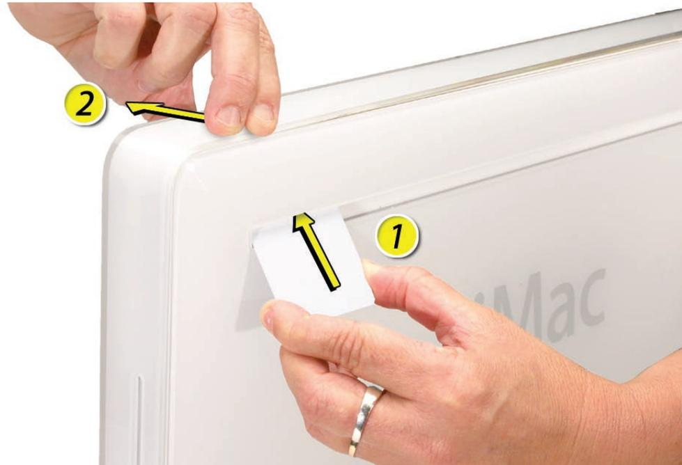
8. Lay the unit screen-up on an ESD mat, with the bottom facing toward you. Lift up the top of the bezel and pull it slightly toward you to separate it from the top of the rear housing.
