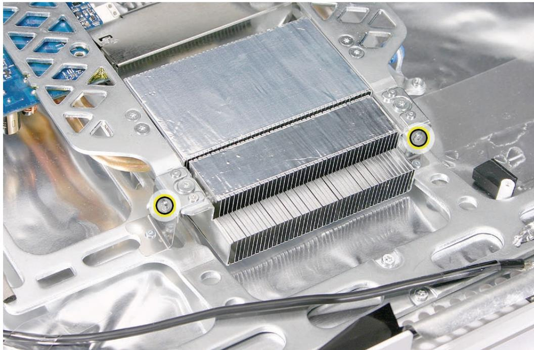
5. **Note:** If the replacement logic board doesn't have the support brackets (shown below) installed on the heatsink, transfer them to the replacement logic board. Remove the two T6 screws on the top of the brackets and the T7 screws from the side support bracket.
