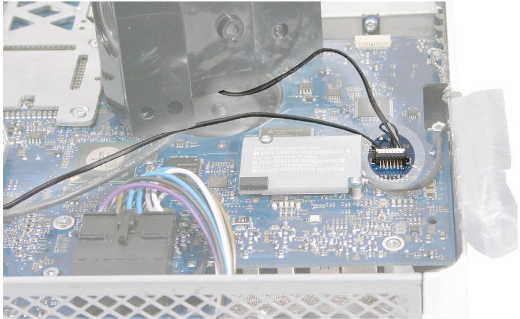
2. Install the speakers and route the speaker wire as shown below.
