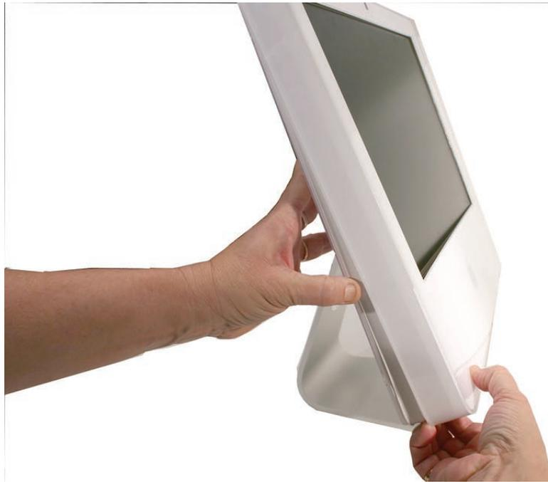
9. Once the access card has been removed, it is safe to open the bezel. Position the unit on an ESD mat, with the bottom facing toward you. Lift up the top of the bezel and pull it up and slightly toward you. **Caution:** Make sure the memory eject rings are not protruding from the access door when you lift the bezel or you could bend or damage the eject rings.
