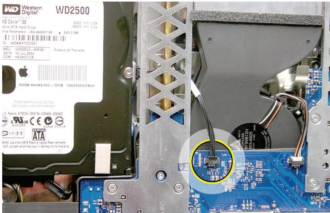
6. Replace the optical drive sensor cable, flex cable and screws, and the silver EMI tape.
