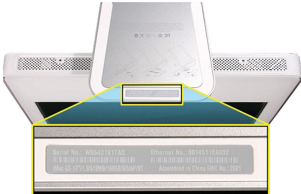
iMac G5 (iSight) serial numbers are located on the bottom of the computer stand.
