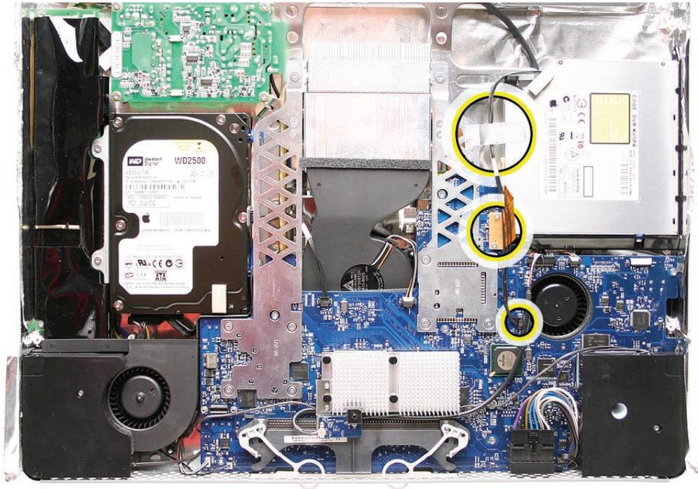
7. Using a T10 torx screwdriver, replace the seven screws on the board. Always install the machine screws (drawn in yellow/white circles) before installing the self-tapping screws (shown in orange).
