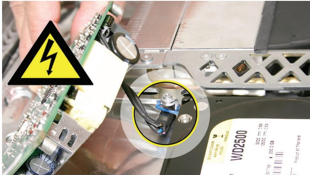
3. Disconnect the two power supply cables; the left cable connects to the DC/DC inverter board and the right cable connects to the AC filter board.
