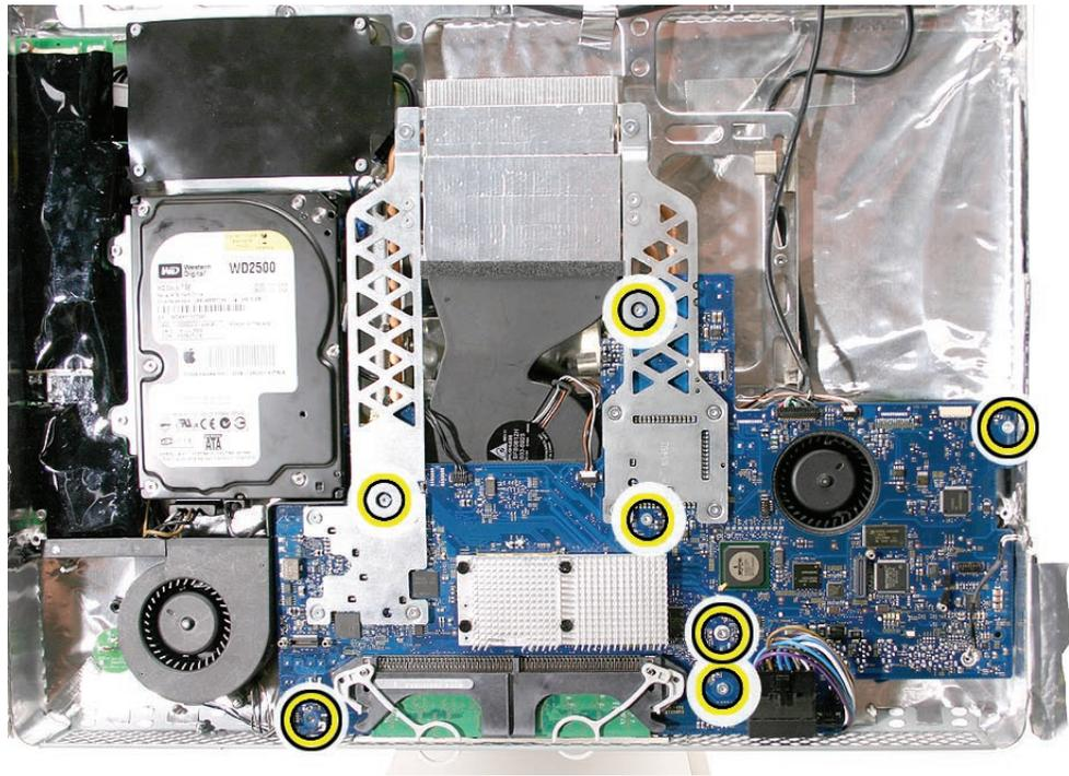
8. Connect the following cables to the connectors on the logic board. Connectors are shown starting in the lower left corner, proceeding clockwise **Note:** The hard drive sensor cable and the optical sensor cable were connected earlier in the procedure.
