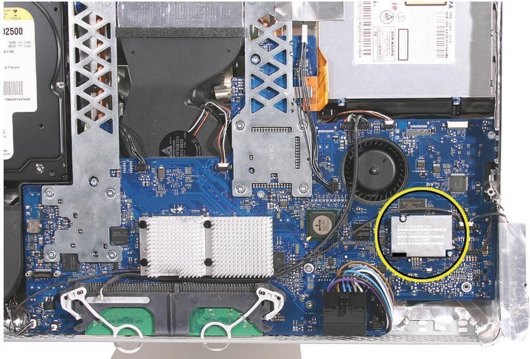
2. Disconnect the optical cable, flex cable, and peel back the silver EMI tape from the logic board frame.
