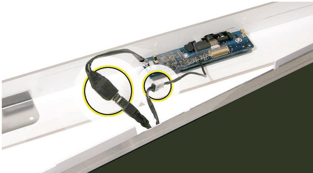
4. Tuck the camera board cables neatly into the channel on the rear housing.
