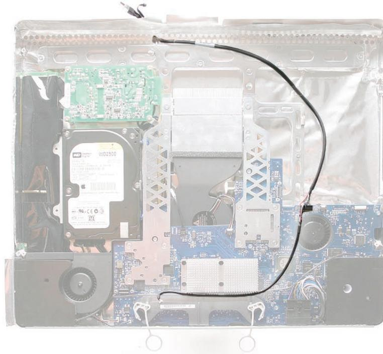
3. Replace the optical drive, flex drive cable and screws, and optical drive sensor cable.
