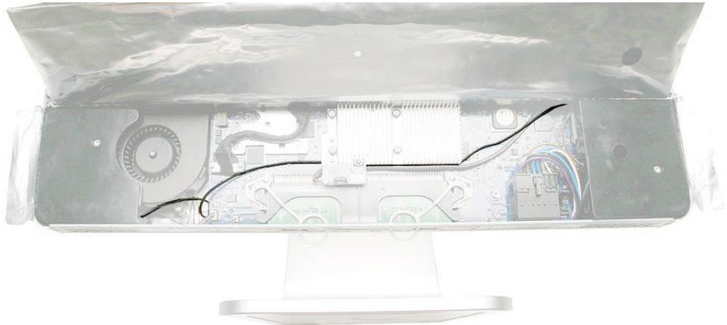
3. Secure the right speaker with the smaller of the two mounting screws.
