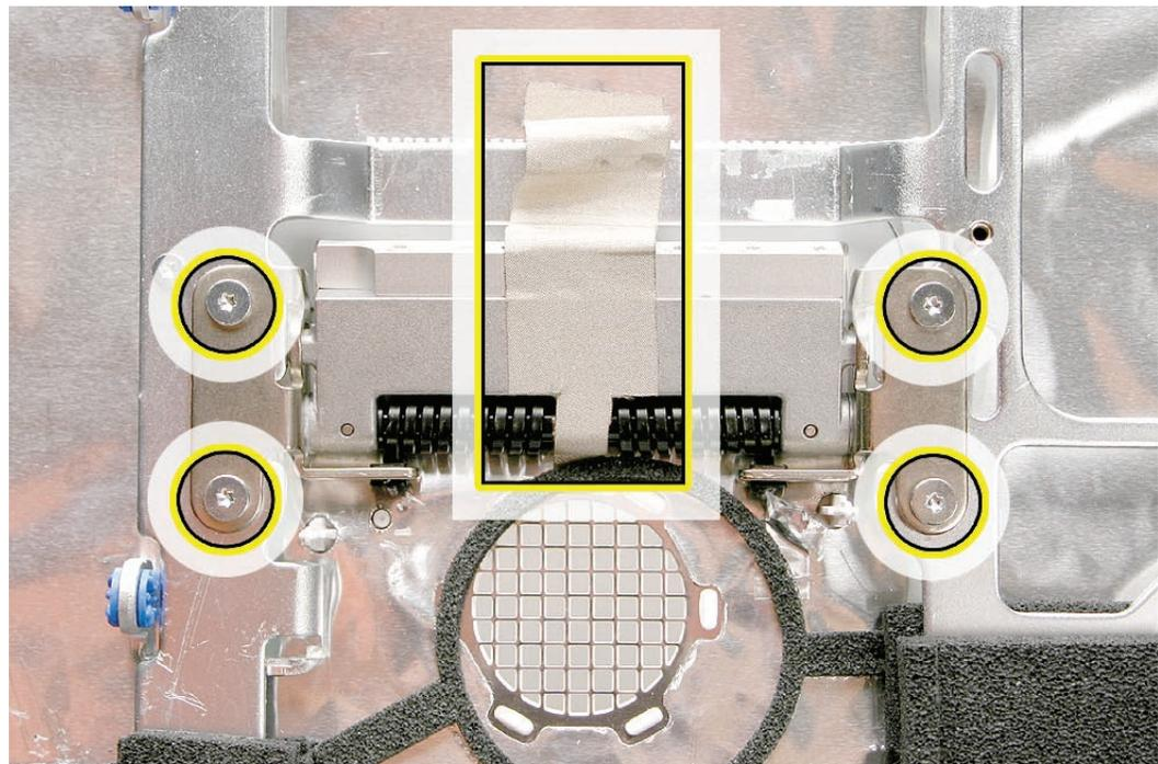
3. Stand up the unit, to access the clutch-to-stand mounting screws.
