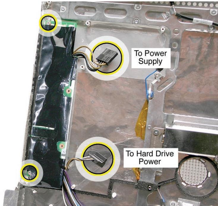
2. Remove just the circled chassis screws, one of which is the AC filter ground screw. Carefully lift the chassis frame just enough to pull the inverter cable from under the metal chassis.
