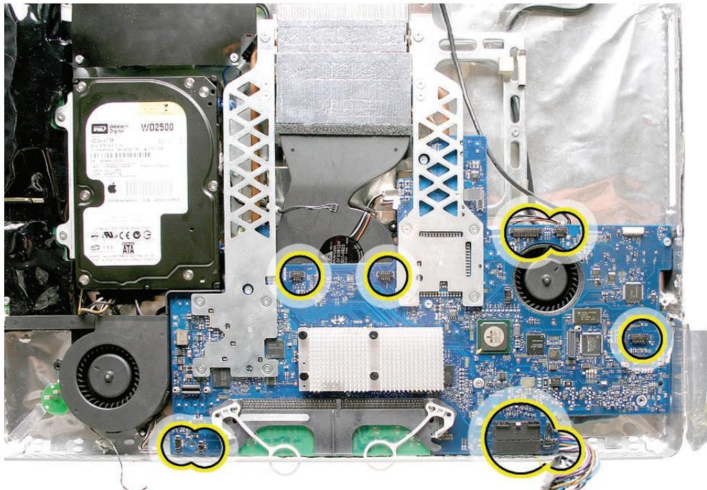
7. Lift the board enough to disconnect the hard drive data cable located on the underside of the metal railing, on the left.
