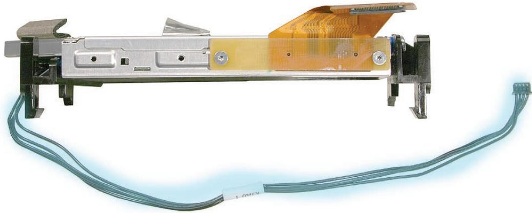
8. Note: The optical drive sensor can be identified by the presence of resistor R1701. The hard drive also has a sensor, but its resistor is R1700. **Note:** The optical drive sensor and mounting bracket will be attached to all replacement optical drives.
