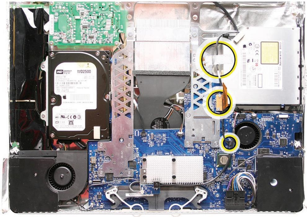
2. **Note:** Make sure to use a needlenose pliers with teeth to remove the optical drive. The pliers must have a textured surface to properly grasp the optical drive release tabs.
