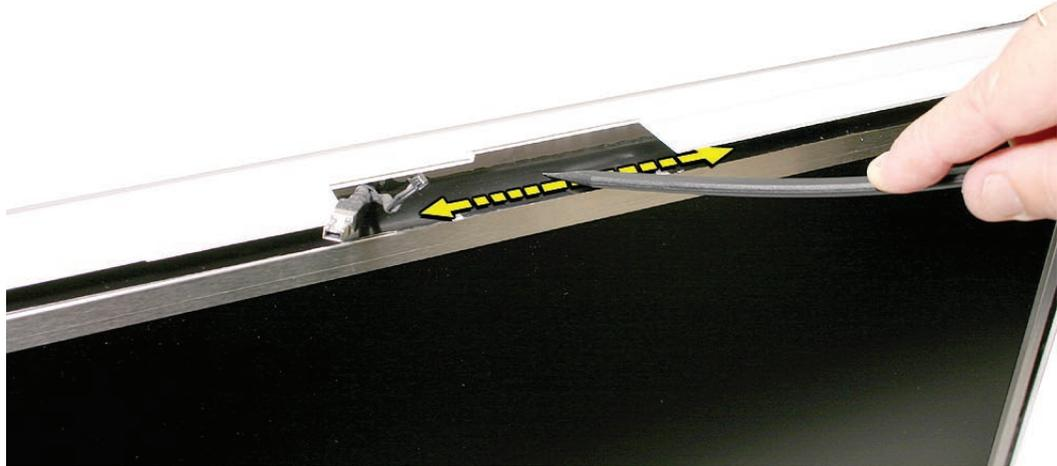
2. Connect the camera and microphone cables (on the camera board) to the cables sticking out of the top of the computer.
