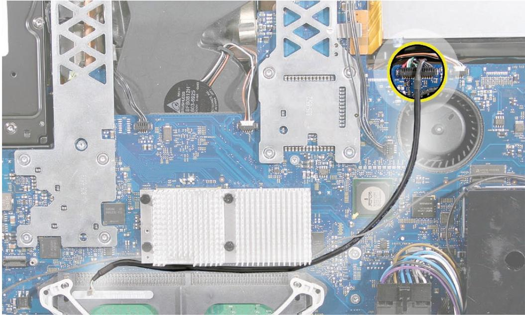
2. Install the IR board mounting bracket and screws.
