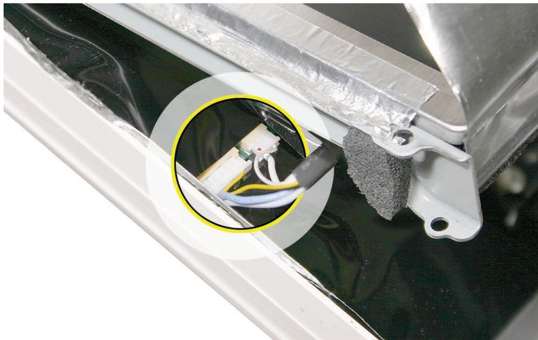
10. Raise the panel up the rest of the way to locate the two inverter cables on the top left side of the display. **Replacement Note:** The cable connectors are marked with dots to indicate “right-side up”.
