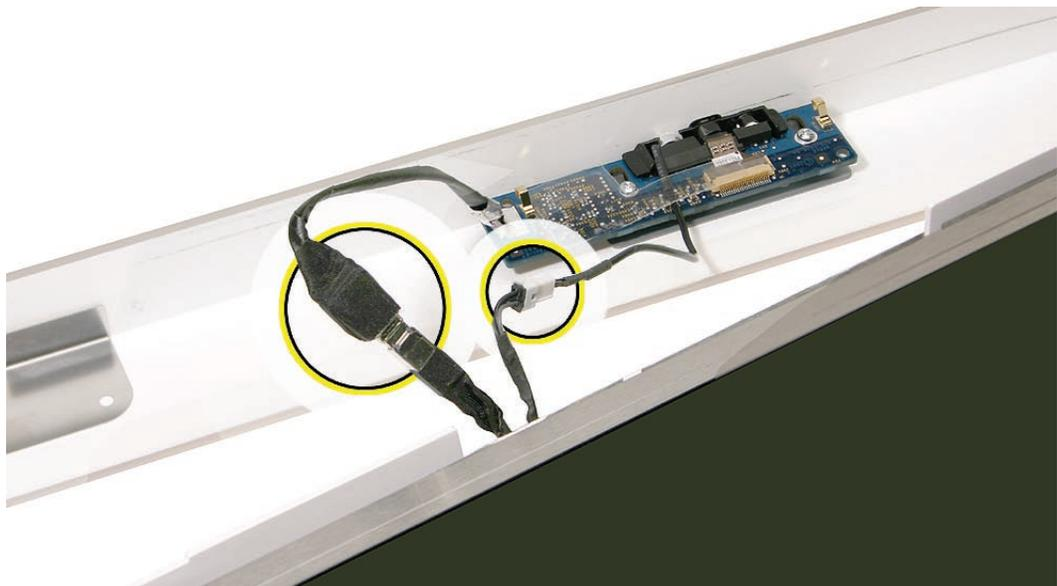
3. Tuck the cables neatly into the channel on the rear housing.
