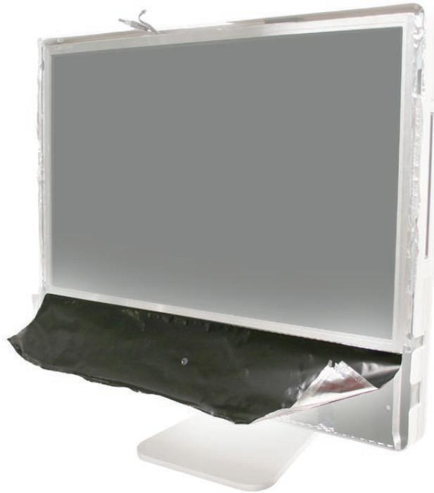
4. Using the access tool, a black stick, or your fingers, peel the black EMI tape off the right and left sides of the panel.
