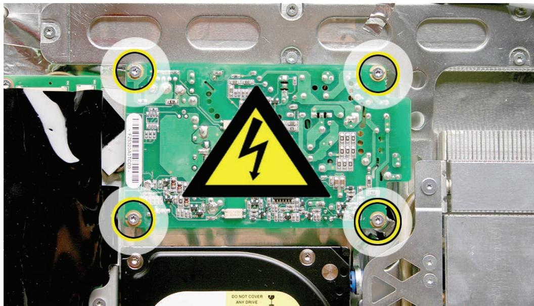
2. Lift the power supply up and remove the cable and connector from under the chassis. This cable connects to the AC filter board located under the logic board. Note the routing of the cable under the chassis.
