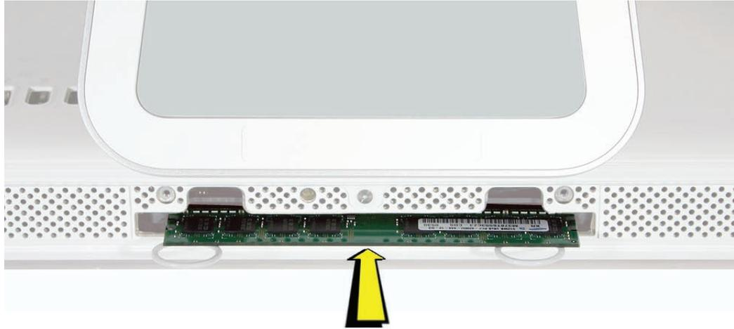
2. Replace the access door using it to push the rings into the memory compartment.
