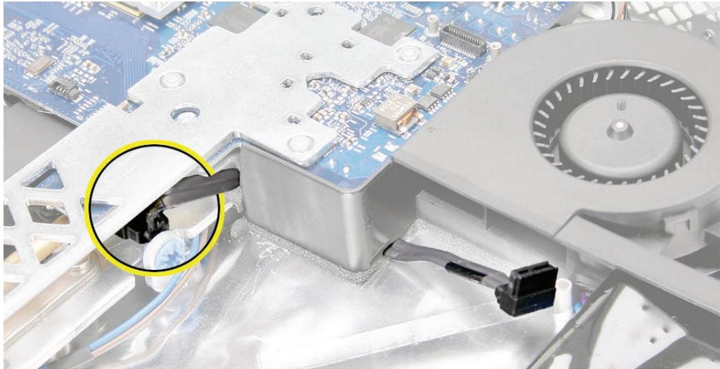
5. Make sure the hard drive sensor and the sensor cable are attached to the side of the hard drive. Route the sensor cable under the chassis and connect it to the logic board.
