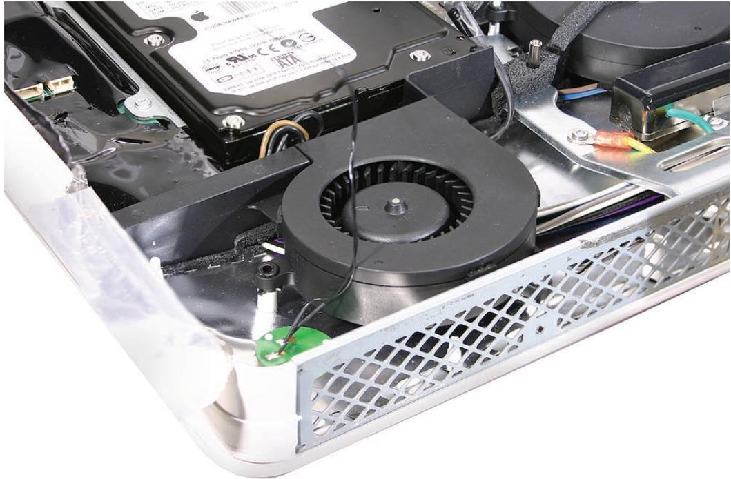
2. Make sure to route the hard drive data cable under the fan as shown in the photo. Connect the hard drive cable to the logic board if it was removed during the take apart.
