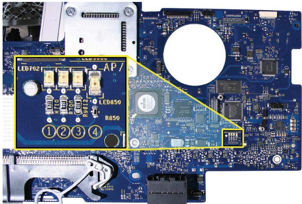
7. Plug the power cord into the iMac G5 and into the AC outlet. Check to see if diagnostic LED #1 is On or Off.
