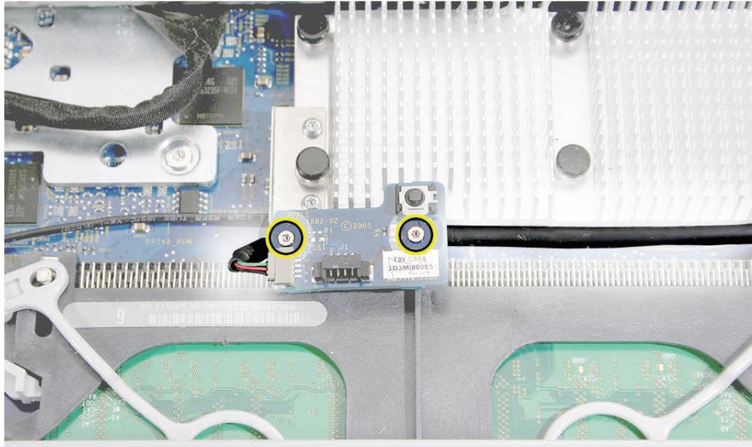
3. Using a Torx T6 screwdriver, remove the two IR board mounting screws. Remove the IR board mounting bracket from the logic board.
