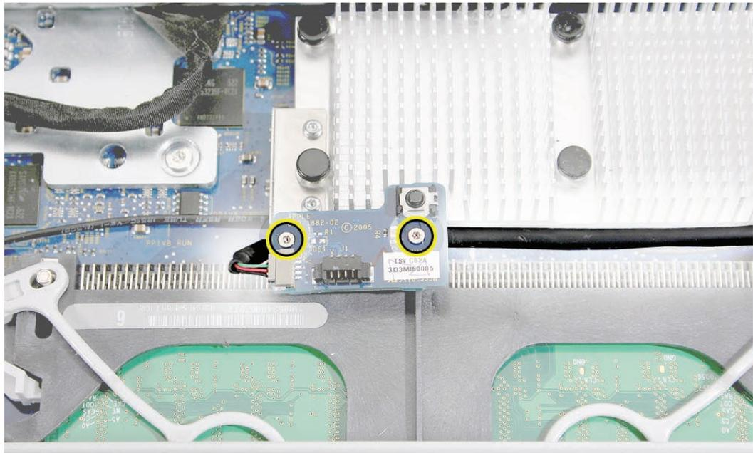
3. Remove the IR mounting bracket screws. Lift the bracket off the logic board to free the speaker cable.
