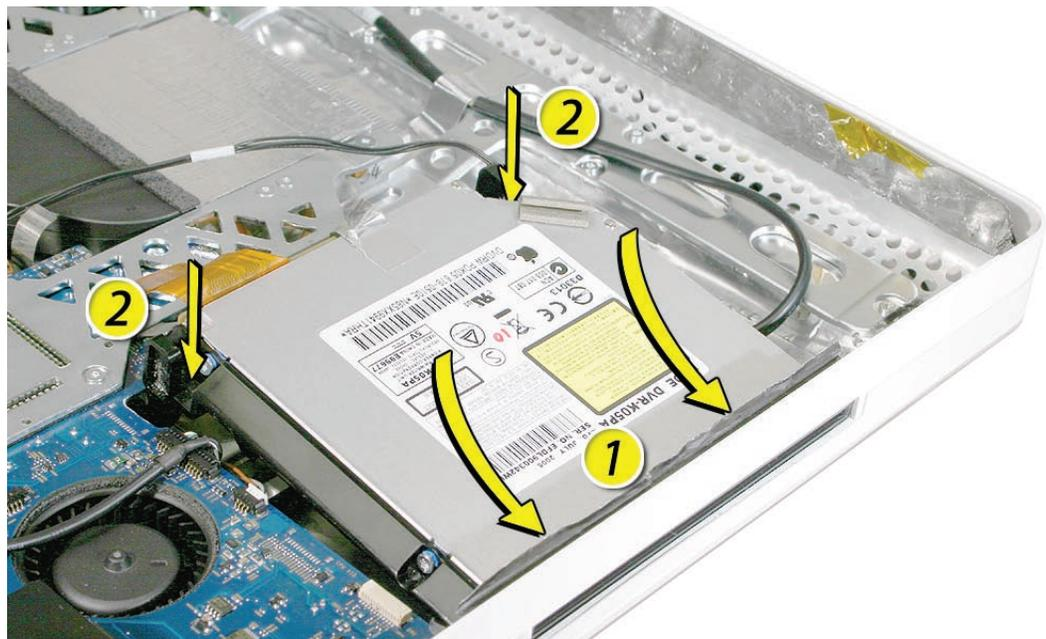
3. Connect the optical drive sensor to the logic board, attach the flex cable and secure it with the T6 screws, and reattach the silver EMI tape.
