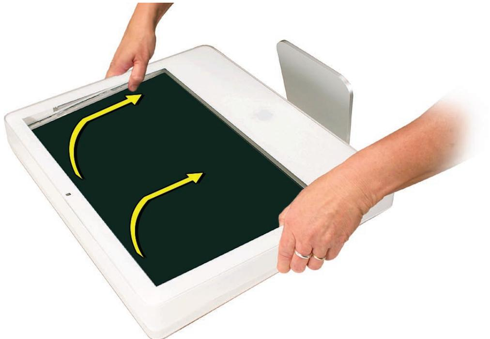
9. Lift the front bezel straight up to remove it. Then swing the bezel upright onto its top edge so you can disconnect two cables that tether the bezel to the rest of the unit.
