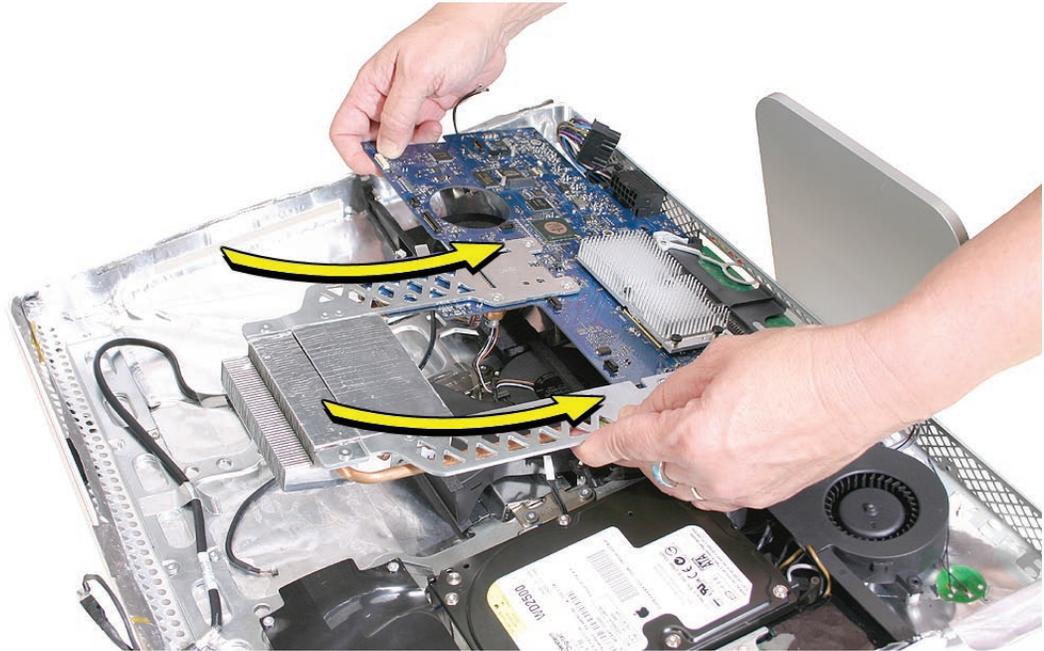
3. **Note:** If the replacement logic board doesn't have the support brackets (shown below) installed on the heatsink, transfer the brackets from the old board. Replace the two T6 screws on the top of the brackets and the T7 screws from the side support bracket.
