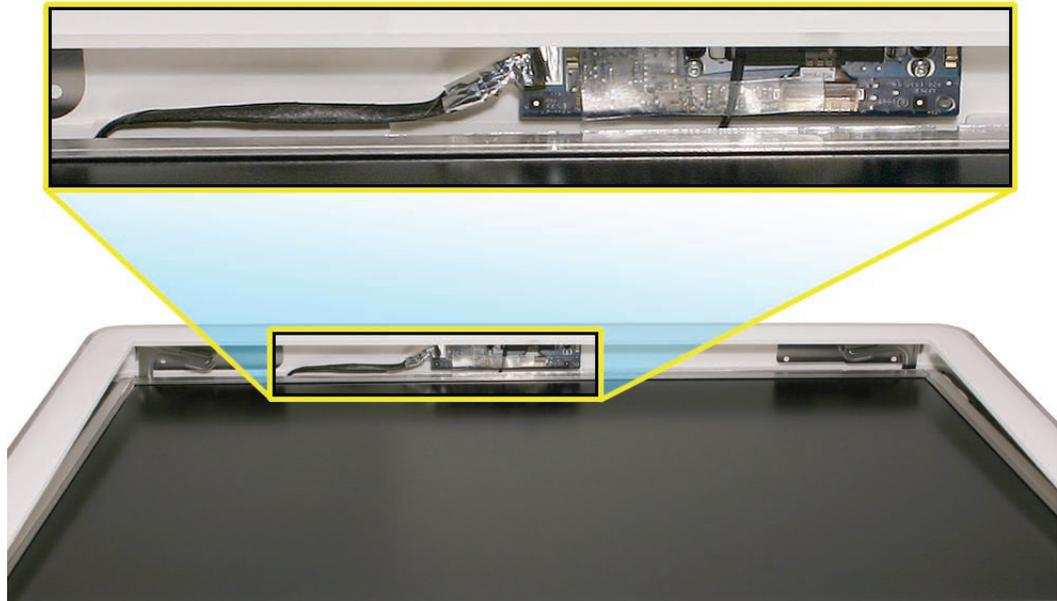
5. Continue to lower the front bezel down over the pull rings (in the memory compartment) and then lower the top corners of the front bezel so they connect with the magnetic latches.
