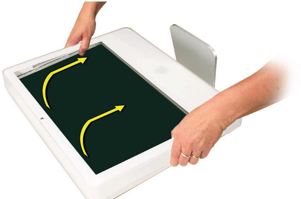
10. Swing the bezel up so you can disconnect two cables on the camera board at the top of the bezel.
