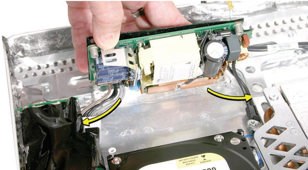
3. Replace the power supply screws. Install the machine screw (bottom right corner) first when installing the power supply.
