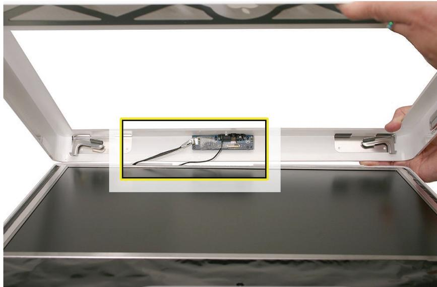
11. Disconnect the camera and microphone cables from the camera board.
