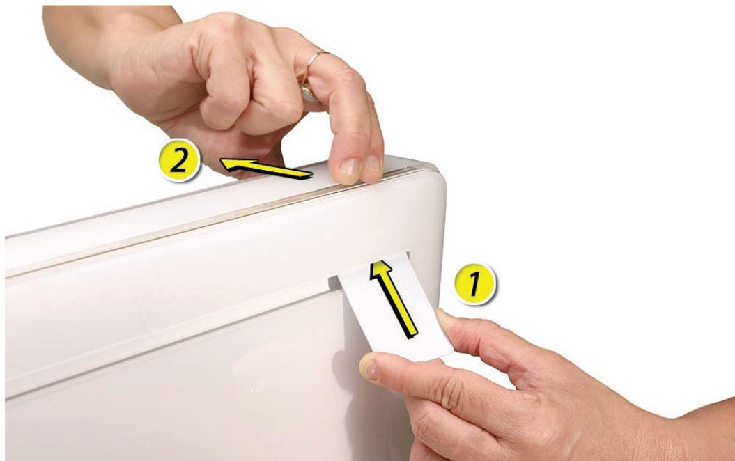
7. Repeat step 6 to release the locking mechanism in the opposite upper corner.
