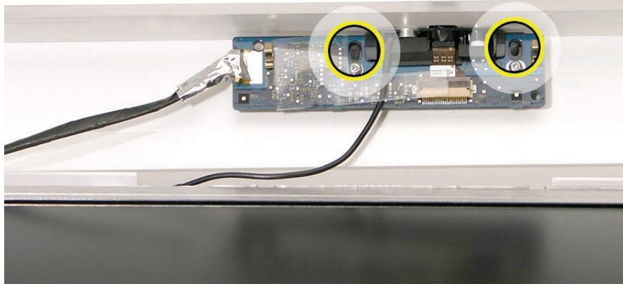
4. Peel back the clear mylar material to free the microphone cable from the camera board.
