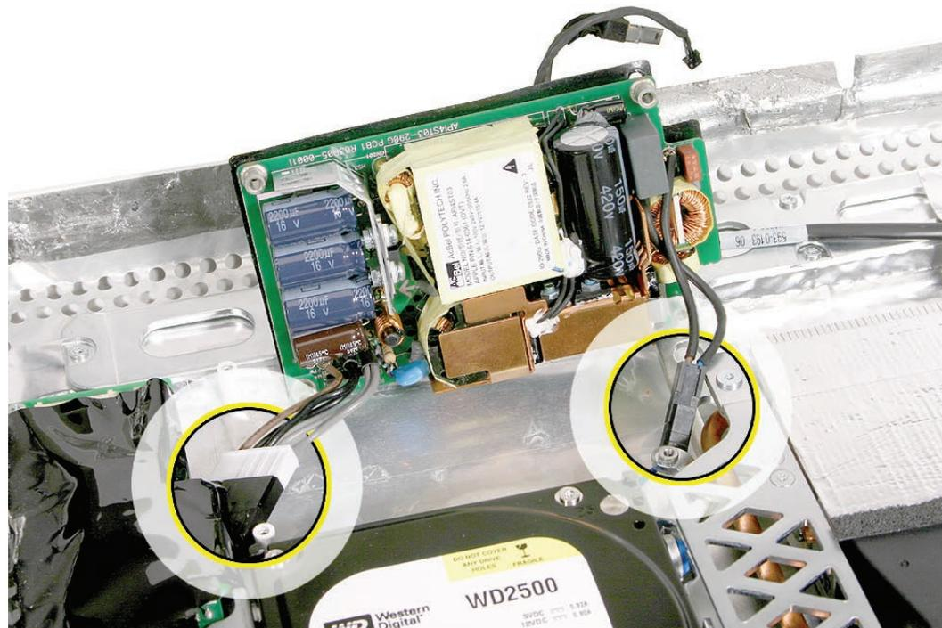
2. Tuck the cables under the DC/DC power supply/inverter and the metal chassis as shown.
