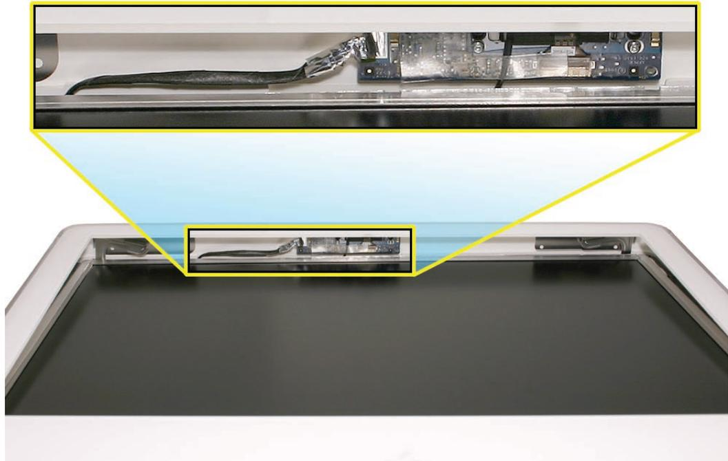
4. Continue to lower the front bezel down over the pull rings (in the memory compartment) and then press the top corners of the front bezel to connect the magnetic latches. **Note:** check that the latches are connected by lifting the front bezel at each corner.
