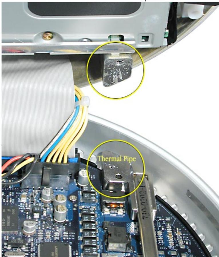
2. Squeeze a thin film of thermal paste onto the thermal pipe. Spread the paste evenly.
