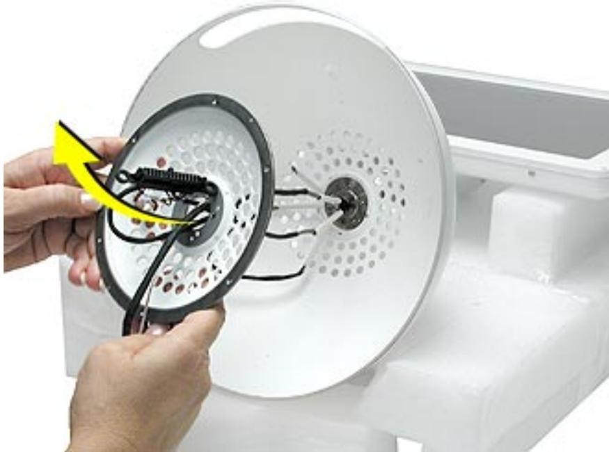
2. Next, carefully pull the neck cables through the hole in the plastic housing. **Note:** Turn the blind mate connector vertically to pull it through the hole.
