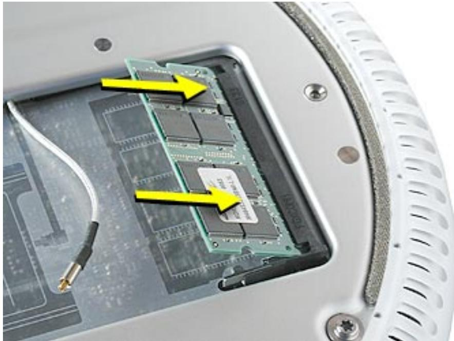
4. Press down gently on the memory until you hear it click into place under the two locking tabs (circled below) on the sides of the slot.
