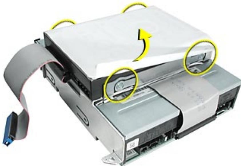
9. Remove the hard drive from the carrier.
