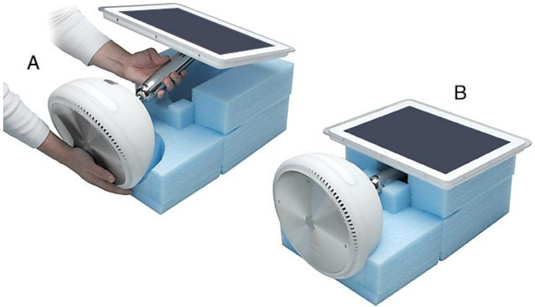
2. **Note:** The base of the computer can be rotated when servicing internal parts.
