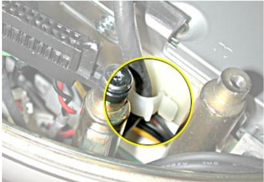
6. Grasp the carrier on both sides. Lift and pull the carrier in the direction of the arrow. Once the carrier is out, flip the carrier to the right to disconnect the power cables.
