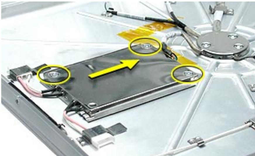
2. Turn the inverter over and disconnect the inverter neck cable.
