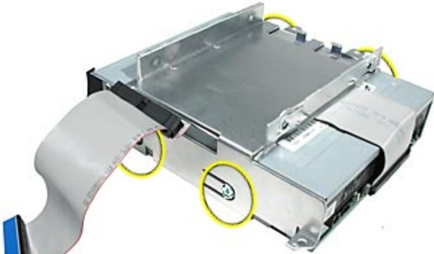
11. Slide the optical drive out of the carrier. Be careful of the black plastic dust filter on the carrier. It is very fragile and can rip easily if not handled properly. **Note:** The silver insulator is part of the carrier assembly.
