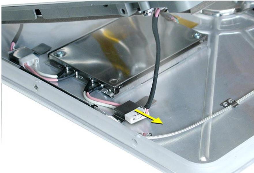
5. Raise the display to disconnect the circled items: the antenna, the inverter cable, the microphone, and the power on LED. Then, peel the tape away from the video connector and open the clip to release the video cable (see next page for a close up of the clip). **Note:** View this page at a larger size to enlarge the graphic.
