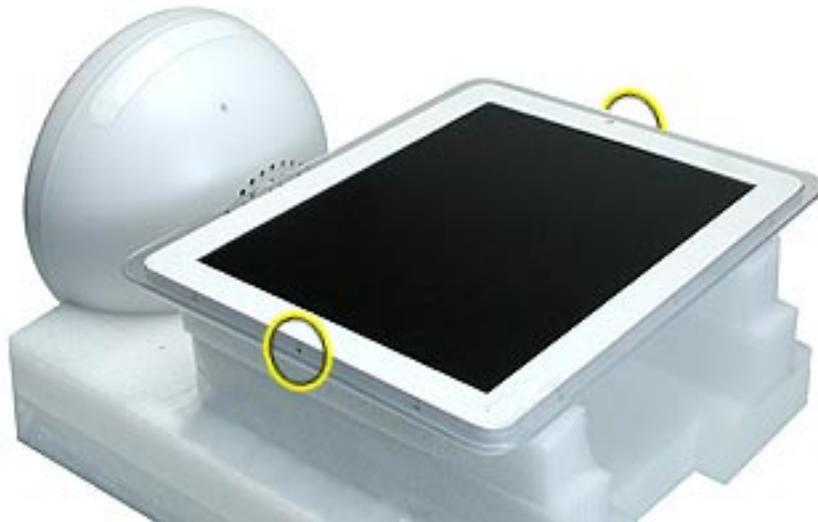
3. With a plastic tool, raise the display to access cables underneath the flat panel.
