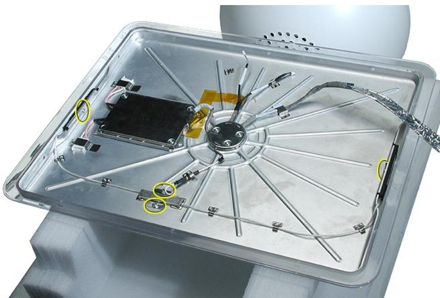
3. Remove the antenna from the metal clips on the panel shield. Lift the antenna from the panel shield.
