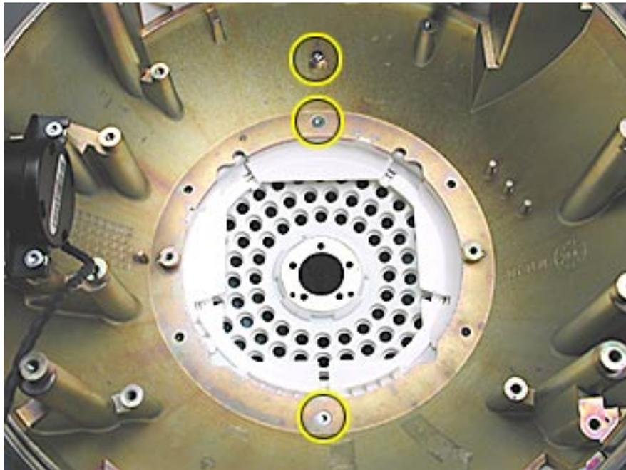
2. Separate and lift the Faraday cage away from the outer housing. Be careful not to scratch the white plastic housing. **Important:** The Faraday cage is very heavy and has sharp edges; handle with care.
