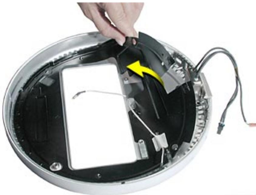
2. Remove two screws and lift the AC line filter from the bottom housing. **Note:** The AC line port cover plug may fall out of the bottom housing when you remove the AC line filter. Place the plug back into the bottom housing before reinstalling the AC line filter.
