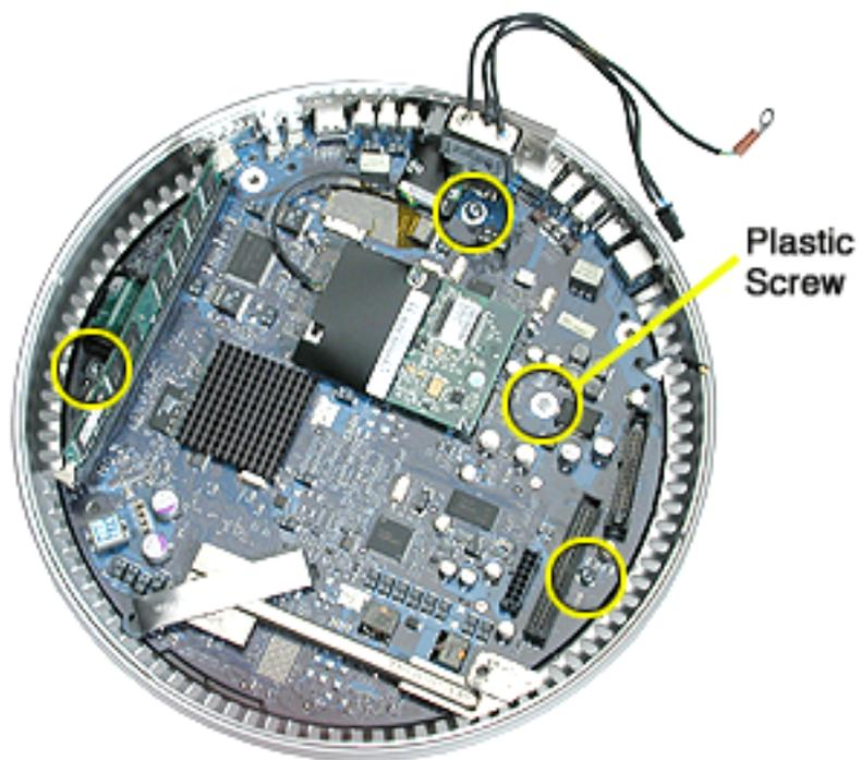
2. Grab the logic board by the battery retainer and the hard drive connector. Lift the board and pull back to release the board from the bottom housing and I/O ports. **Note:** The I/O port covers may come out with the logic board when it's removed.
