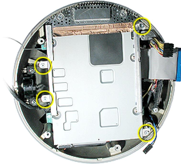
5. Remove the Airport antenna and the video cable from the plastic clip on the side of the hard drive.
