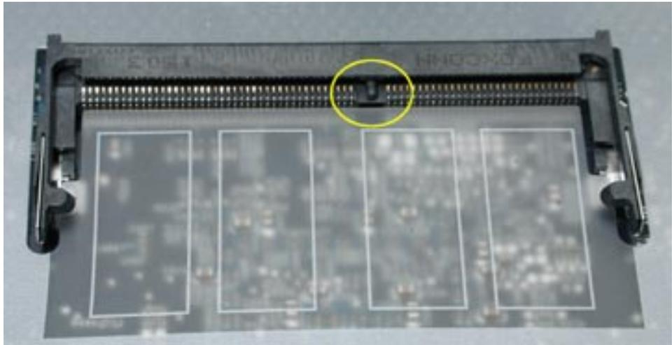
2. **Important:** Do not push the clips (circled below) when inserting memory. They are used to remove memory from the slot, not to insert memory. These clips are fragile and can break.
