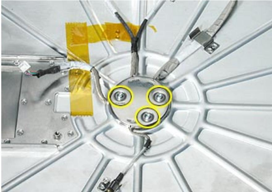
2. Remove the four T-10 screws on the panel shield. Next, release the cables from the metal clips on the panel shield. **Note:** View this page at a larger size to enlarge this graphic.
