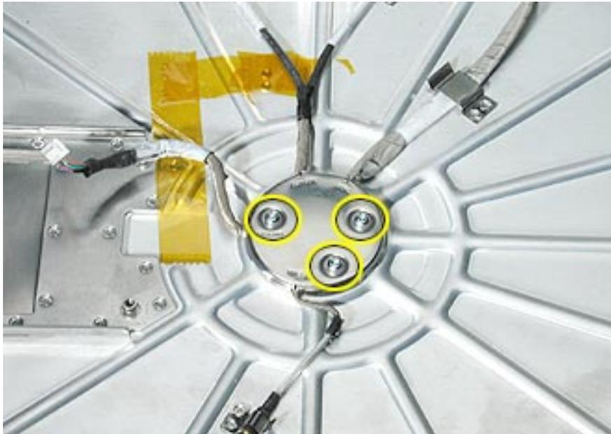
3. Loosen the four screws (shown below) that hold the panel shield to the neck assembly, and tilt the screen the opposite direction of the tilt.
