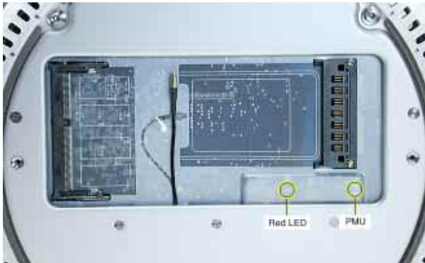
4. Disconnect the A/C power cord. Place the unit in the service stand and remove the user access plate. Press the PMU reset button on the logic board. Refer to “Resetting the PMU on the Logic Board” mentioned earlier in this chapter.
