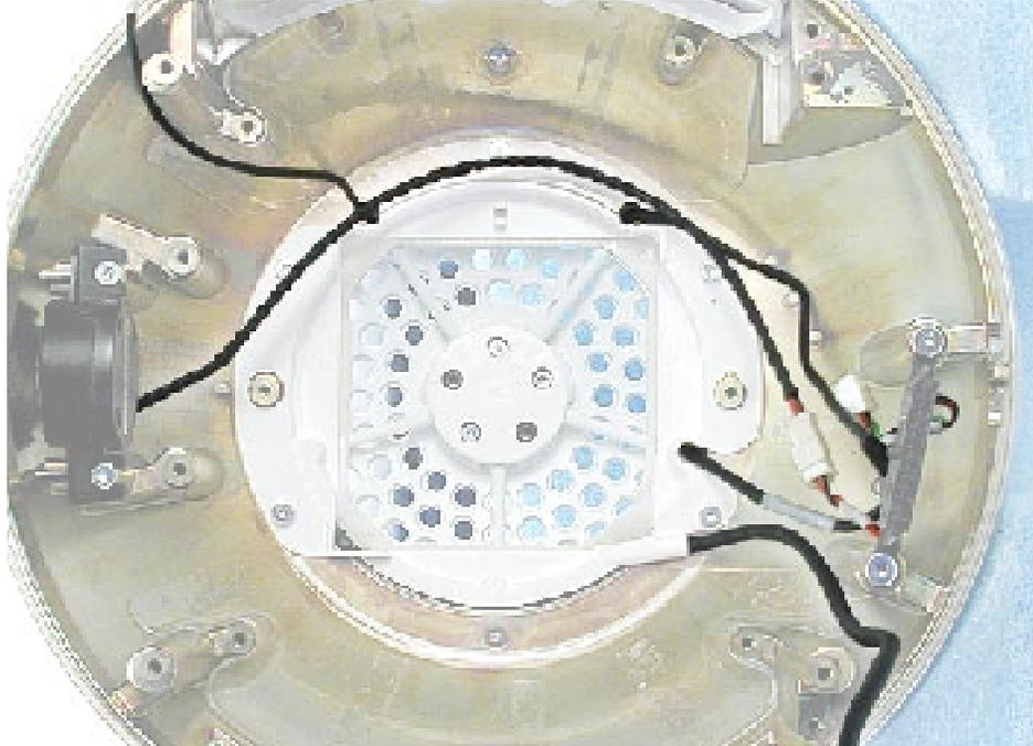
2. There are five screws on the neck cap, however; only the three silver screws need to be removed. The remaining two black screws keep the neck attached to the base.
