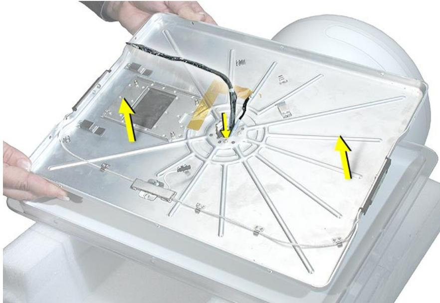
5. This is a close-up of the video cable going through the hole in the panel shield.
