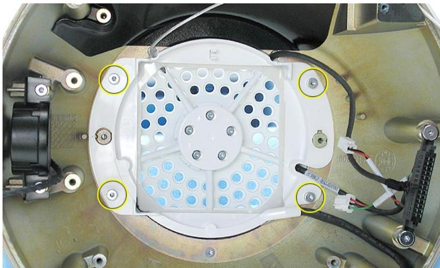
2. Lift the plastic cable retainer from the chassis. **Note:** The fan gasket is stuck to the back side of the plastic cable retainer.
