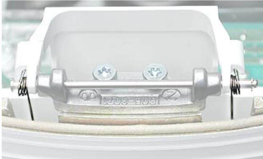
4. Remove the door hinge screws.
