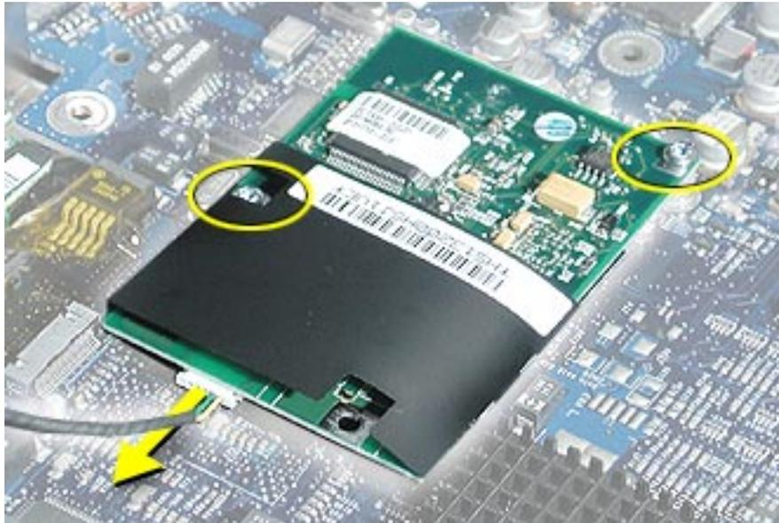
2. Lift the modem from the connector on the logic board.
