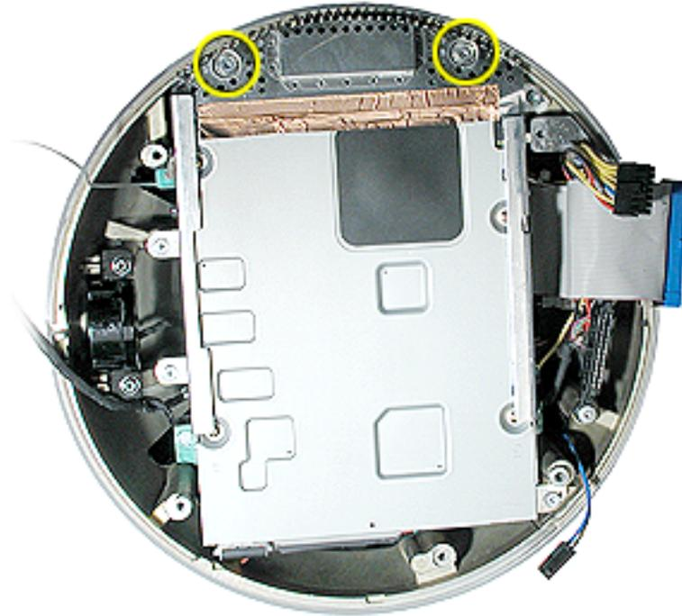
3. **Note:** The copper tape is stuck to the EMI shield and the optical drive. Carefully peel the copper tape off the drive to remove the EMI shield.
