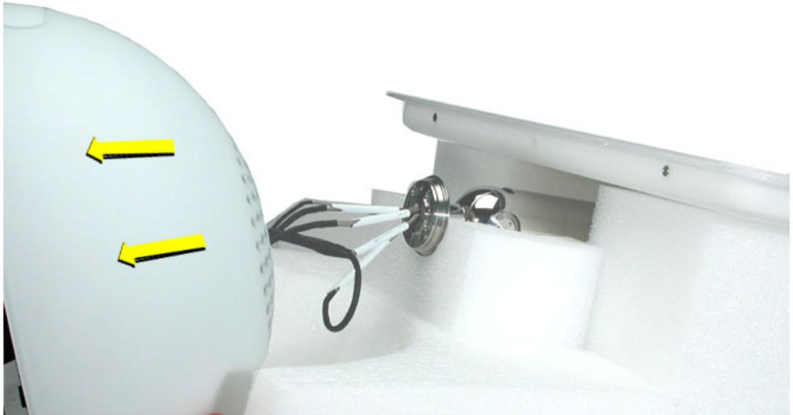
5. **Note:** Perform this step only if you are replacing the outer shell. Remove the three screws in the base of the Faraday cage to separate the shell from the Faraday cage.
