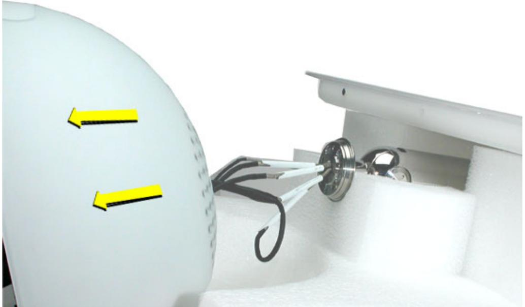
5. Replace the two black neck cap screws to connect the neck to the chassis.
