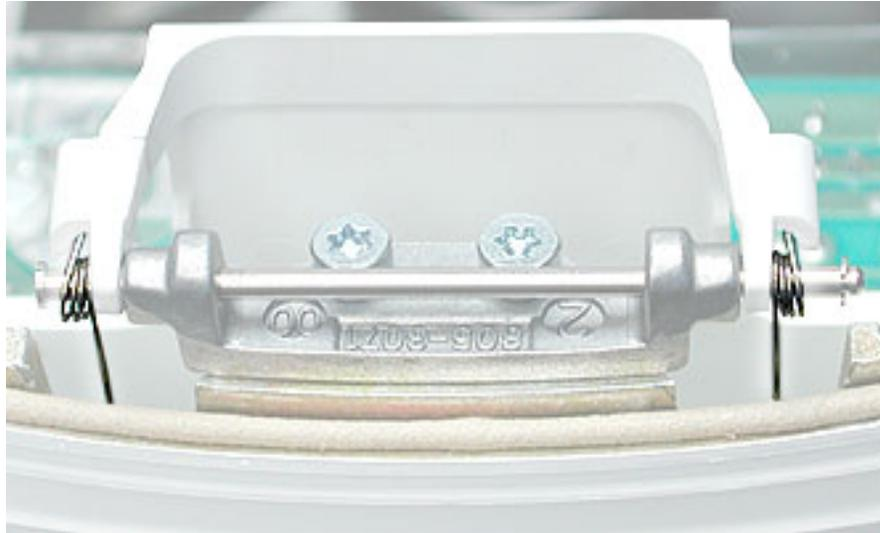
4. Remove the door hinge screws.
