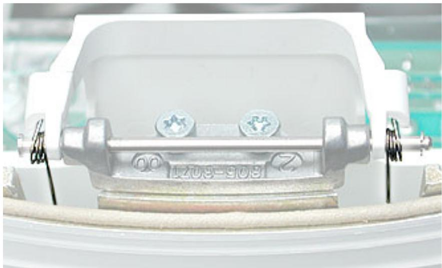
15. Rotate the base so the optical door is on the right. Replace the power supply and the six screws. Remember, the two smaller screw locations are hidden under the optical door flap.
