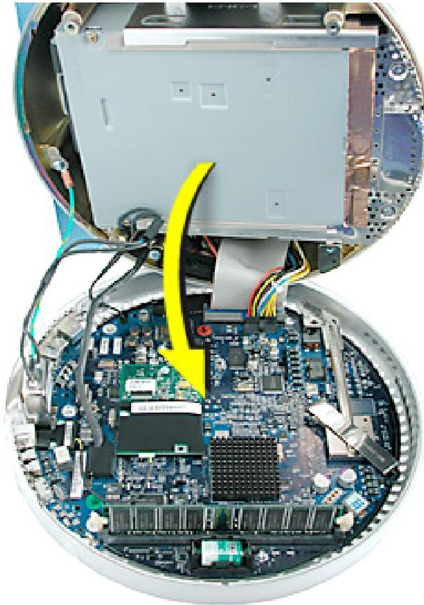
**Important:** Diagnostic service cables allow the unit to run while the bottom housing is open (as shown above). However, the computer cannot run for more than five minutes with the bottom housing open. If it is open longer, the CPU may overheat and become damaged.
