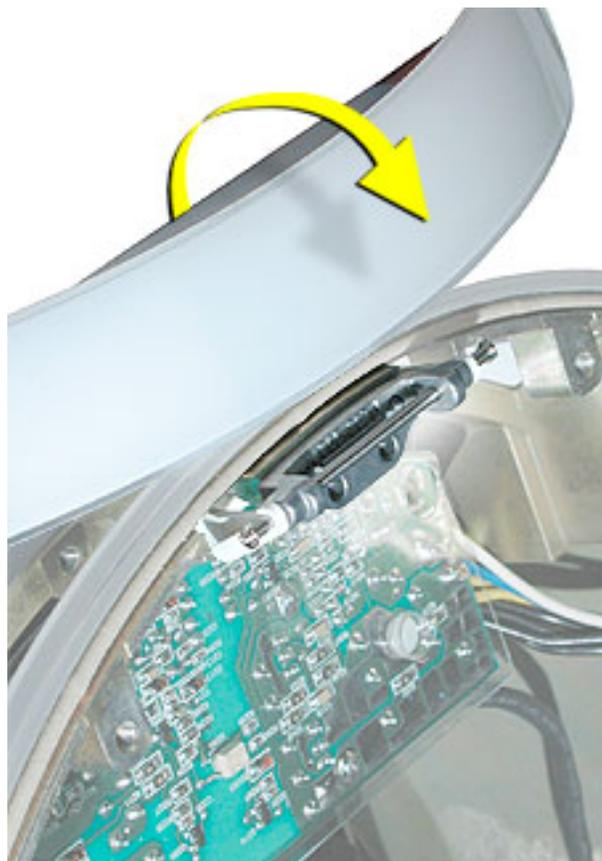
6. Slide the door and hinge off the frame. Remove the door from the base.
