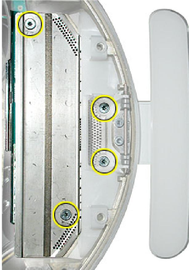
3. Remove the power supply from the chassis, keeping the two halves connected.
