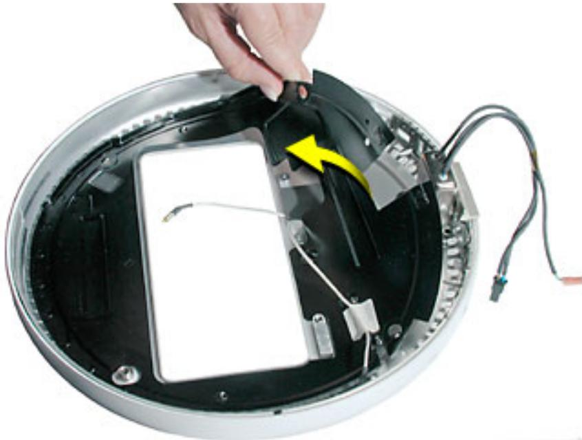
23. Replace the modem filter board into the opening in the bottom housing. Replace the modem and modem filter board screws. Connect the cable to the modem.
