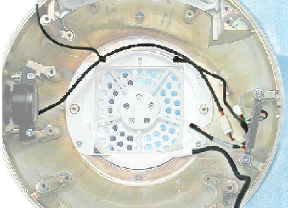
2. Loosen the three silver screws (circled below) to remove the neck cap. Lift the cap off the spokes. **Note:** The two black screws keep the neck attached to the base.
