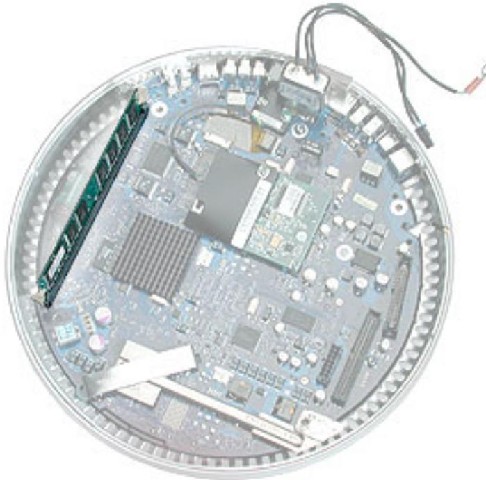
**Note:** The factory-installed memory slot is identified as Slot J13 by Apple Hardware Test and Apple System Profiler.
