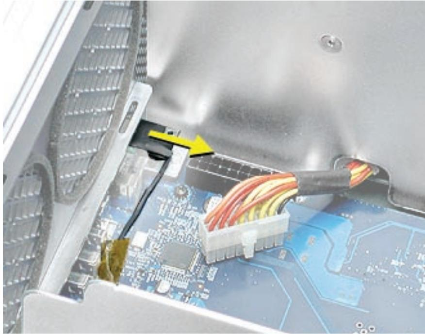
**Replacement Note:** When re-installing the modem filter board in its mounting bracket, be careful to engage the slots in the board with the edges of the bracket.
