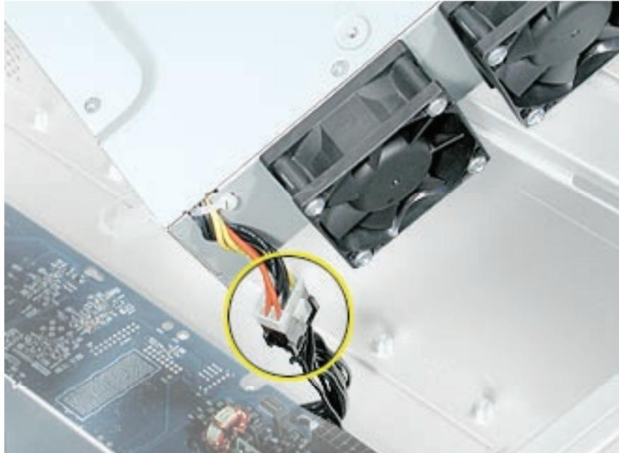
8. Remove the power supply from the enclosure.
