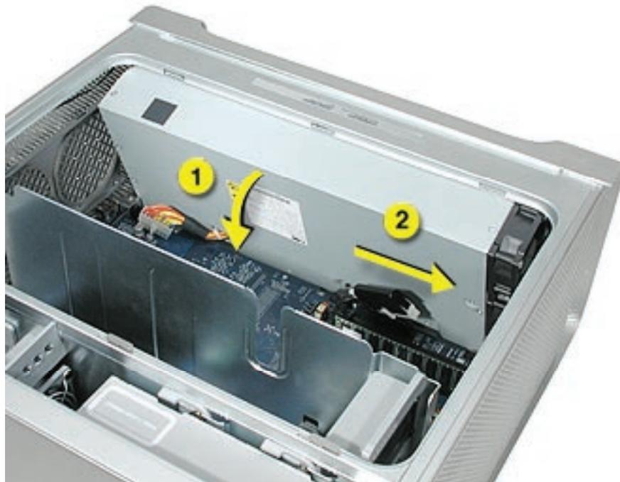
7. Disconnect the power harness cable from the power supply.
