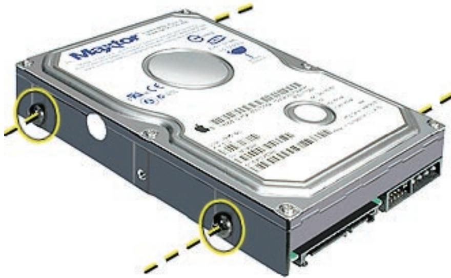
**Replacement Note:** When replacing the top drive, make sure the guide screws align with the middle slot of the drive bay, and then gently push the drive into the bay until it snaps into place.
