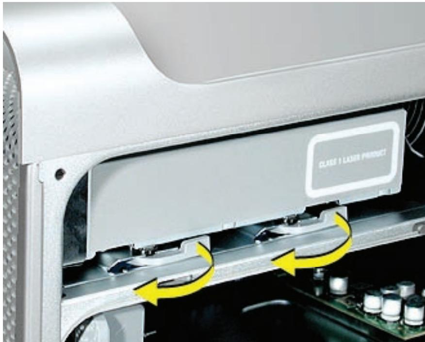
3. Place the fingers on one hand inside the opening for the optical drive cable and push the edge of the drive forward. The drive will move part way out of the media shelf.
