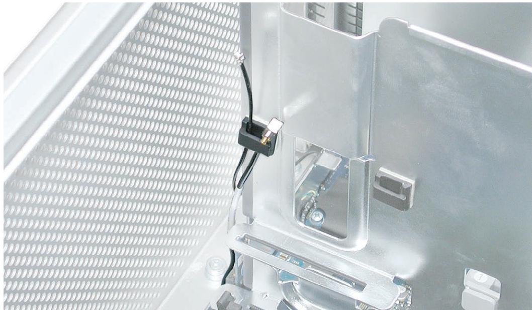
2. Remove the two antenna board mounting screws. Remove the board with the cables.
