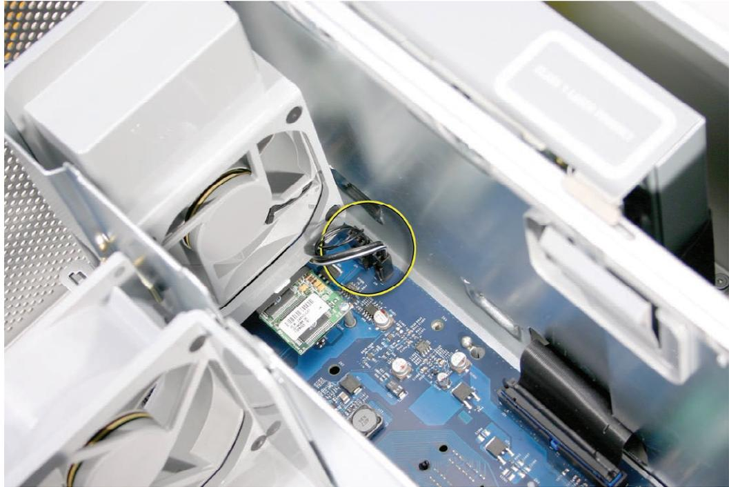
3. If you are replacing the speaker, remove the two screws and remove the speaker from the speaker/fan bracket.
