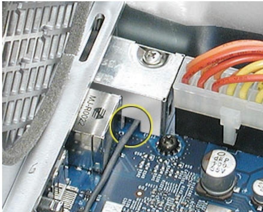
**Replacement Note:** Be careful when rerouting the modem filter cable that it routes under the black connector for the front inlet fan and out through the correct opening in the PCI divider. Make sure the cable is in place behind all cable guides.
