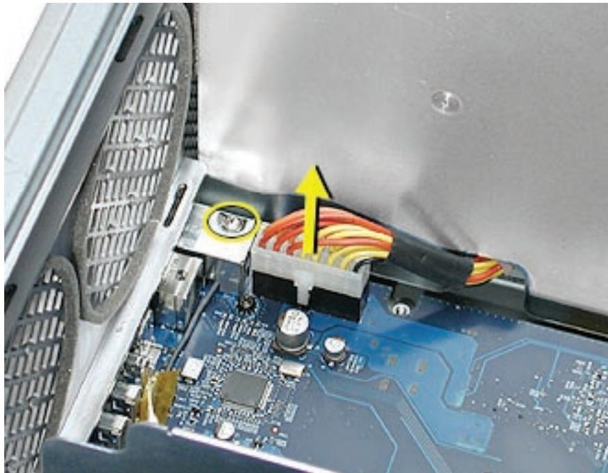
5. Slide the modem filter board back to disengage it from its mounting bracket, and remove the board and cable from the logic board.
