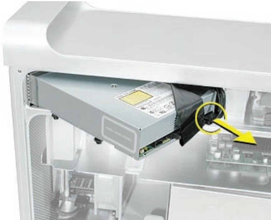
5. Route the drive ribbon cable out through the opening in the media shelf and remove the drive and ribbon cable from the computer.
