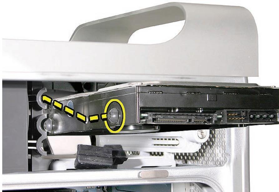
When installing a bottom drive, align the guide screws with the bottom slot of the drive bay and slide the drive in until it snaps into place.
