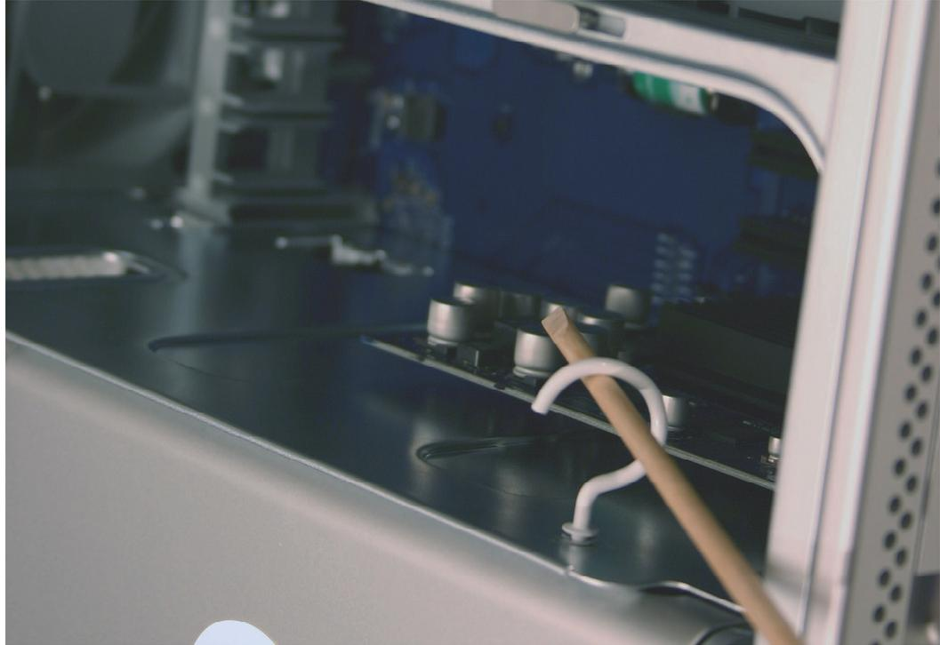
4. Slide the cover to the left to unlatch the four metal latches under the cover. Lift the cover up and off the heatsink.
