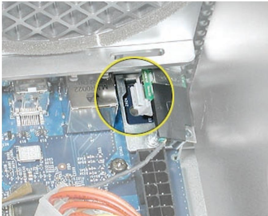
**Replacement Note:** Make sure the modem filter cable routes out through the opening in the side of the modem filter cap before securing the cap to the modem filter board.
