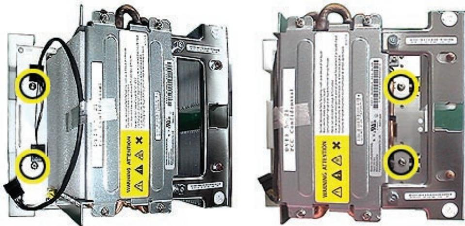
3. Check to make sure the top edges of both processors align.
