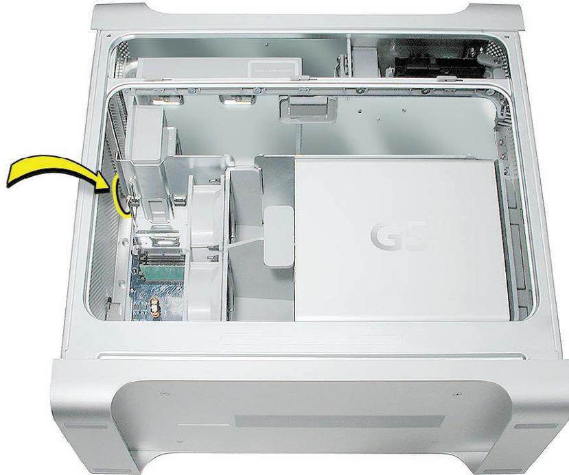
2. Lift the speaker/fan assembly straight up to disengage the large tab (circled) on the side of the bracket from the channel in the sheet metal.
