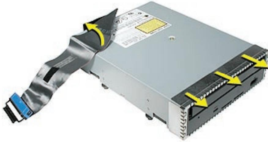
8. Carefully remove the EMI shield from the front of the original drive and transfer it to the front of the replacement drive.
