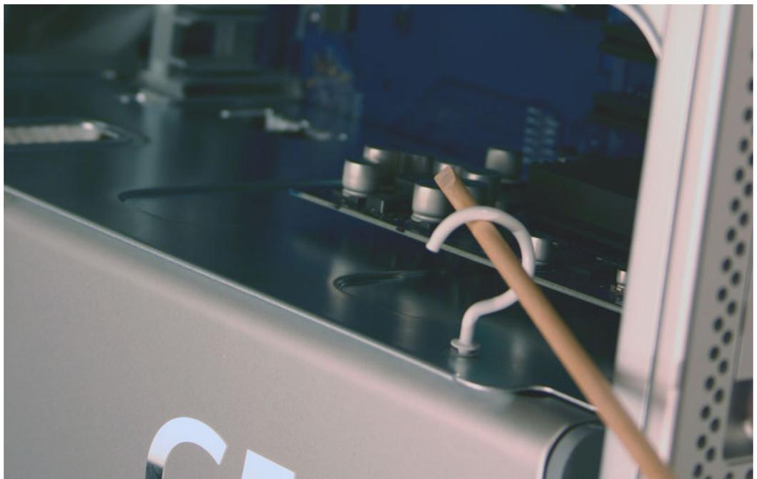
**Note:** The heatsink cover is secured to the computer by three latches below the left side of the cover. The following two steps release the cover from these latches.
