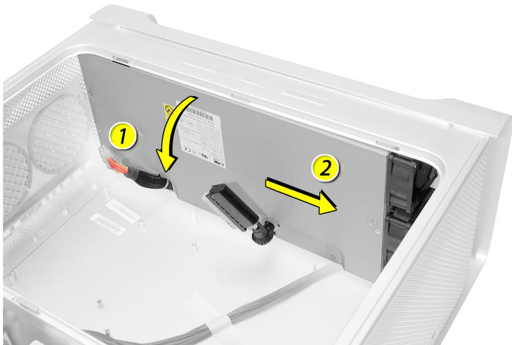
4. Disconnect the power harness cable from the power supply.
