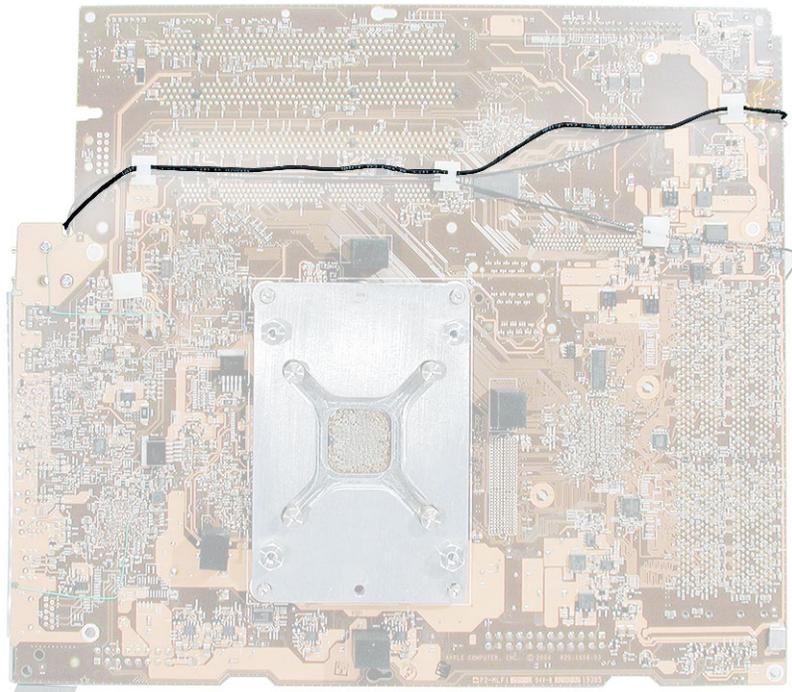
2. Remove the two screws that secure the antenna board, lift the board, and remove the modem cable from underneath the board.
