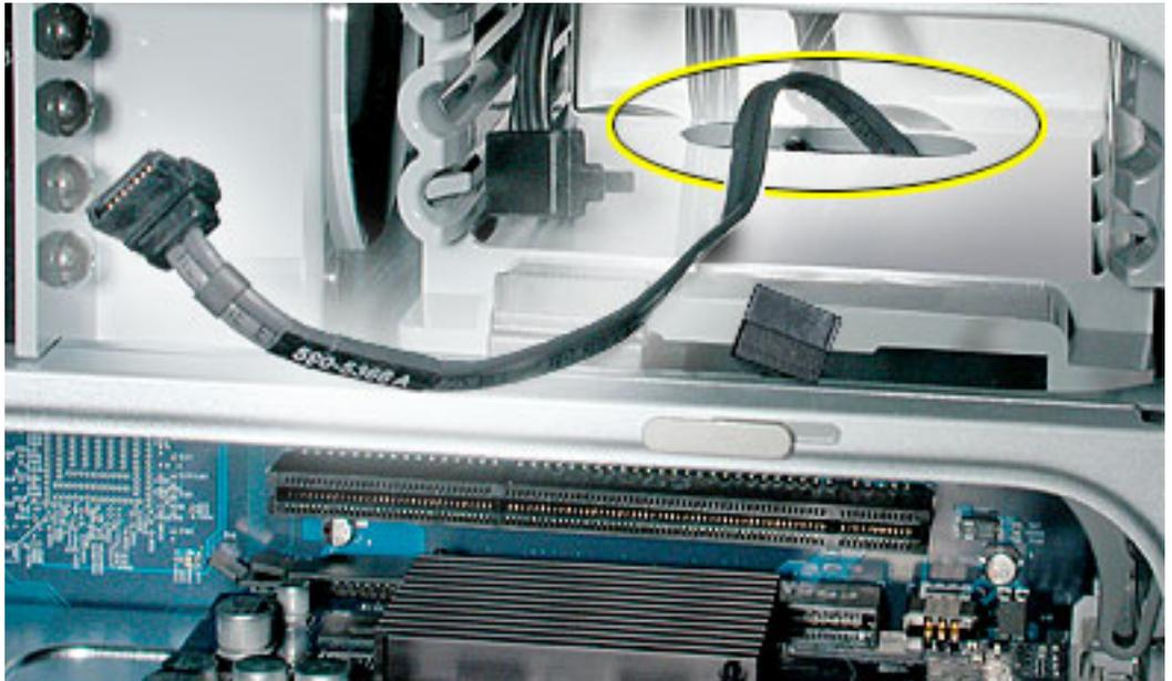
Then install the upper hard drive with the cable routed below the drive, and connect the cable to the drive as illustrated.
