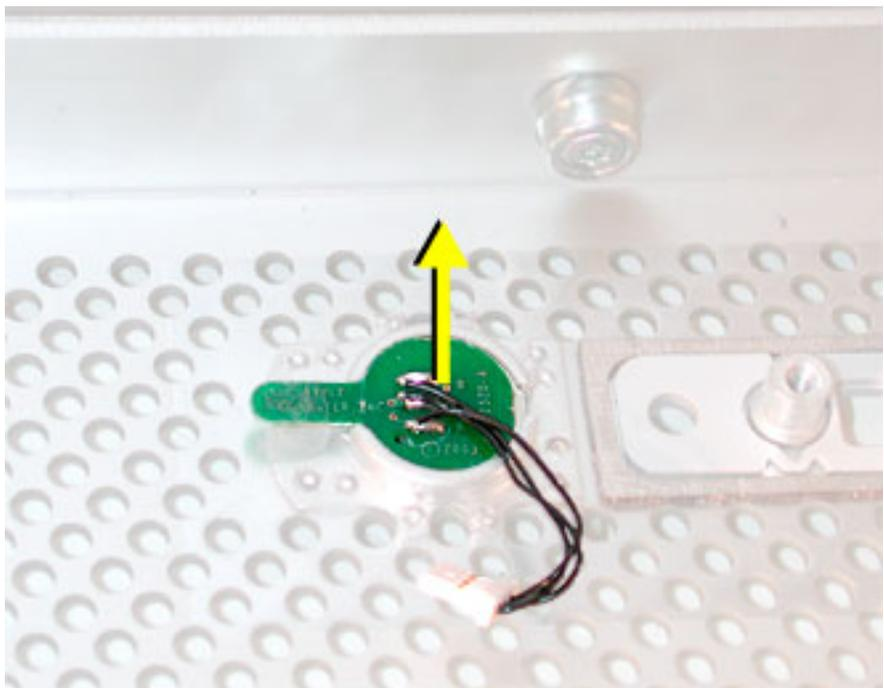
5. Remove the metal activation ring that lies below the power button board.
