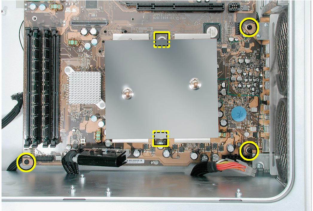
5. Slide the logic board to the left and then lift a short distance straight up to disengage the board from its three mounting posts. Slide and lift the logic board by holding onto the board's edges, never the processor.
