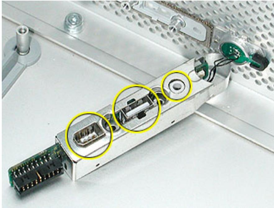
4. Install the front panel board and EMI shield on the inside front of the enclosure and replace the two mounting screws.
