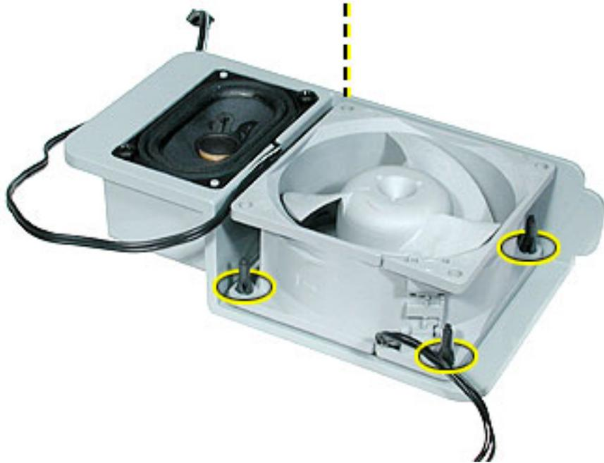
**Replacement Note:** When reinstalling the speaker/fan bracket in the enclosure, make sure the large tab on the side of bracket engages with the channel in the PCI divider.
