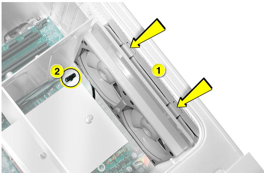
4. If you are replacing the fans, use needlenose pliers to pull each fan off the four grommets that mount it to the bracket, and remove the fans and cable from the bracket.
