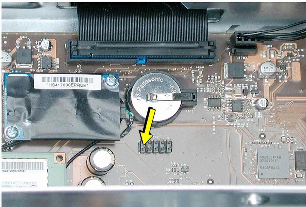
**Replacement Note:** Insert the new battery under the battery holder clip, making sure the side of the battery with the positive symbol faces up and touches the clip.
