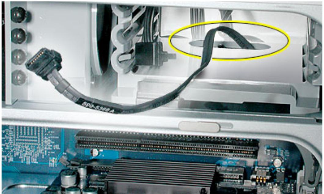
Then install the lower hard drive with the cable routed above the drive, and connect the cable to the drive as illustrated.
