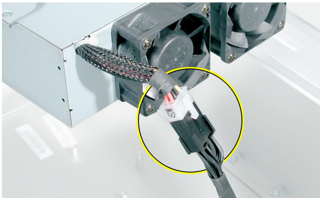
5. Remove the power supply from the enclosure.
