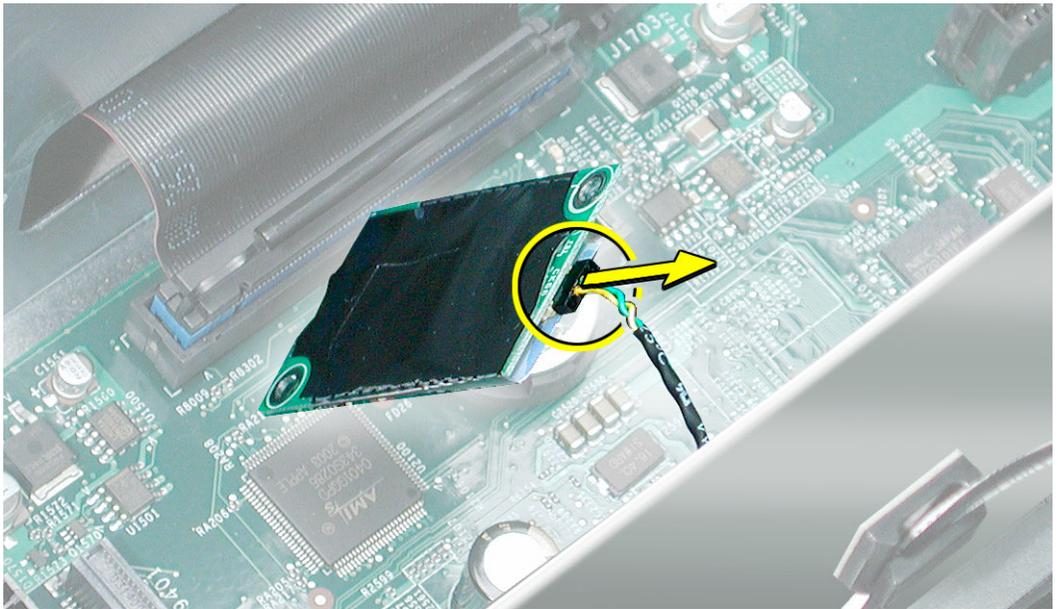
3. Remove the modem from the enclosure.
