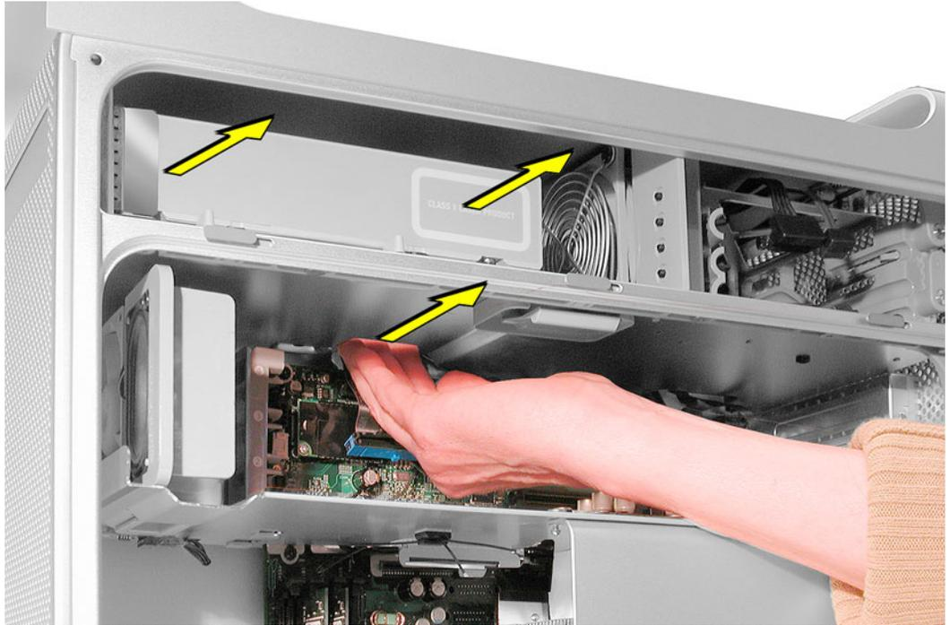
4. Disconnect the power cable from the drive.
