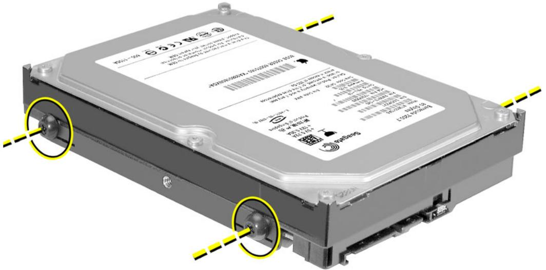
**Replacement Note:** When replacing the top drive, make sure the guide screws align with the middle slot of the drive bay, and then gently push the drive into the bay until it snaps into place in the top position.
