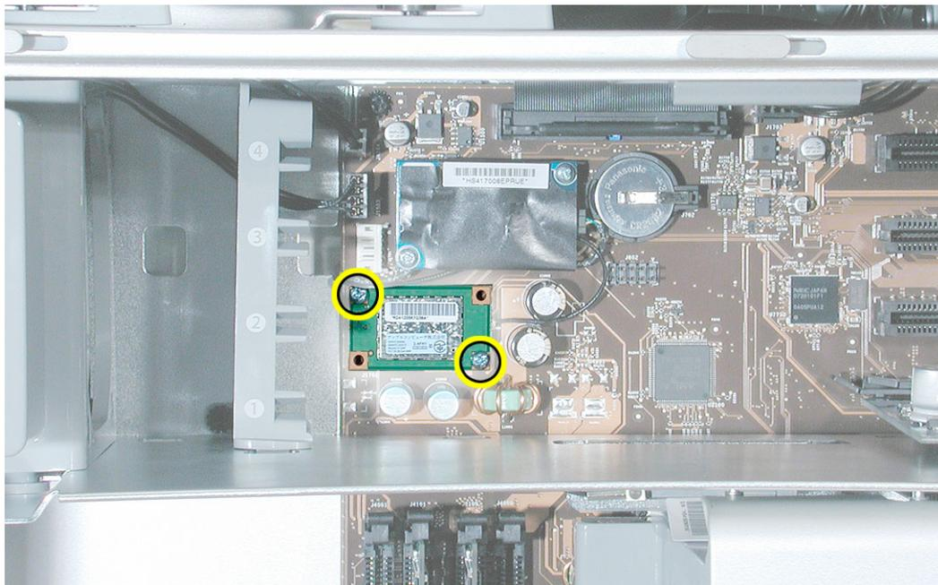
2. Lift the Bluetooth card straight up a short distance to disconnect it from the logic board. Then turn the card over, and disconnect the Bluetooth antenna cable from the underside of the card.
