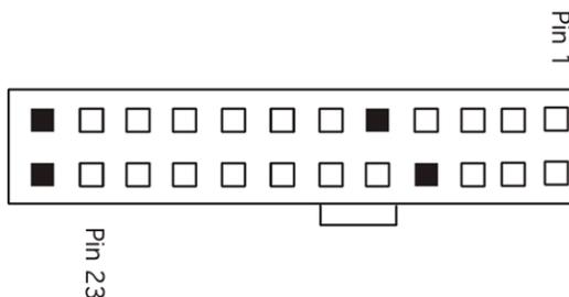
The volt meter should measure approximately +5V. If you do not get a reading of +5V, recheck the volt meter connections and measure the voltage again. If the voltage is still not present, replace the power supply.
