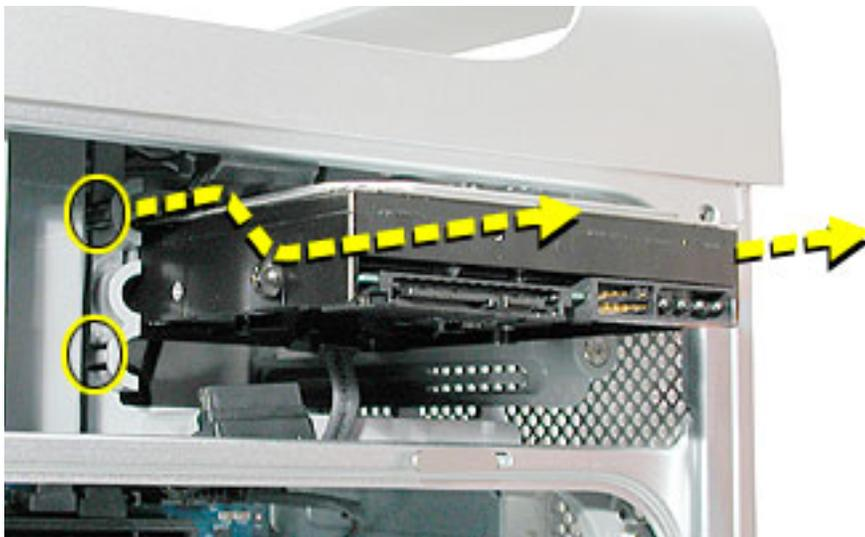
**Important:** If the printed circuit board (PCB) is exposed on the bottom of the hard drive, hold the drive by its sides. To avoid damaging the replacement drive, take care not to touch the PCB during installation.
