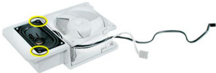
4. If you are replacing the fan, use needlenose pliers to pull the fan off the four grommet fasteners. Then remove the fan from the bracket.
