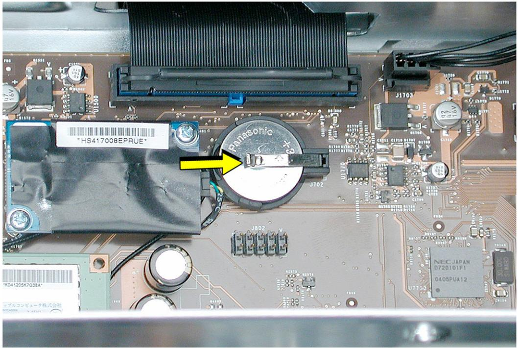
**Warning:** Installing the battery incorrectly may cause an explosion. Be sure the battery's positive symbol faces up in the holder. Use only the same type of battery or an equivalent recommended by the manufacturer of the original.
