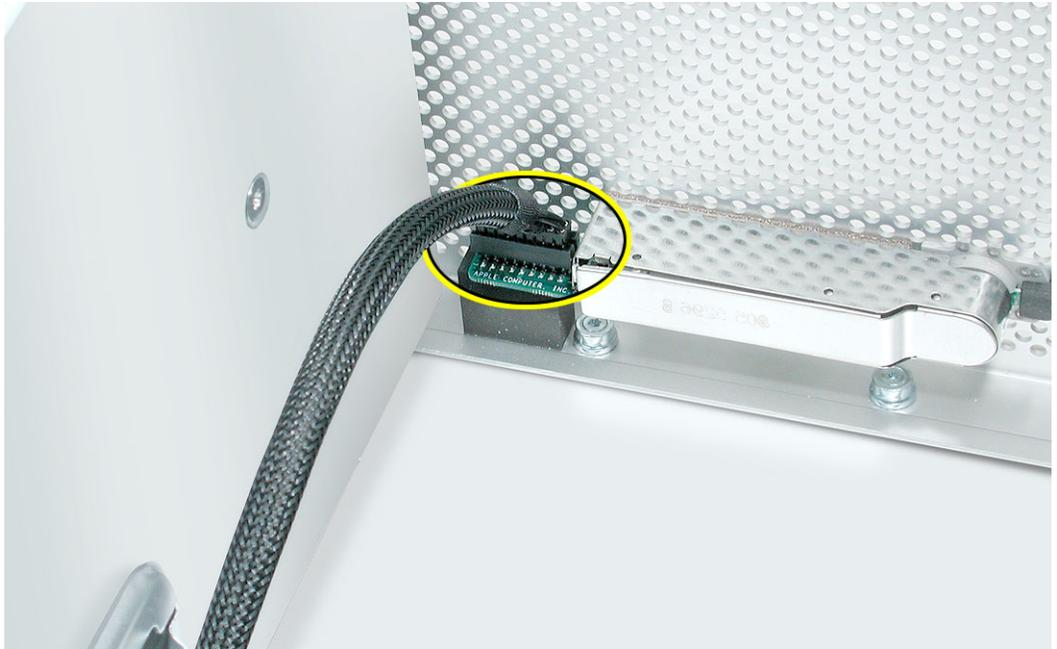
3. Using a jeweler's flatblade screwdriver, pry up the metal cap covering the front panel board EMI shield.
