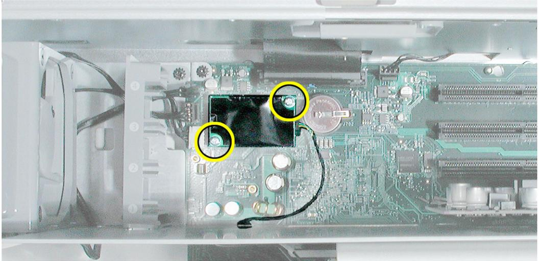
2. Lift the board slightly and disconnect the modem filter cable from the modem board.
