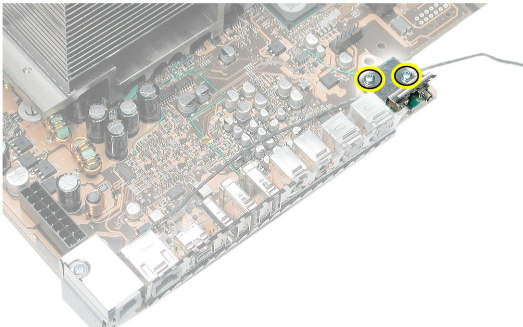
3. Remove the mounting screw on the modem filter board cap and remove the cap.
