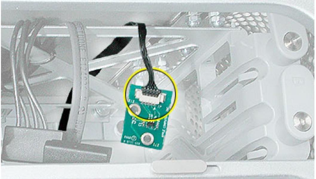
**Replacement Note:** Before installing the replacement board, apply the double-stick tape included in the sensor board kit to the back of the board. Then reconnect the media sensor board cable and press the board to the frame in the location illustrated below.
