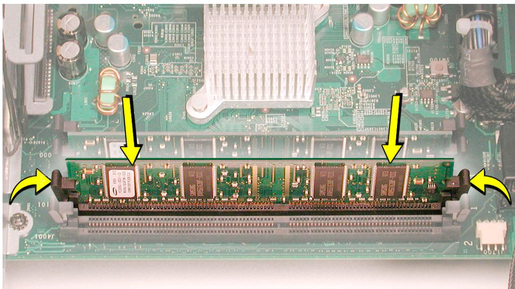
**Important:** Do not touch the DIMM connectors. Handle the DIMM only by the edges.
