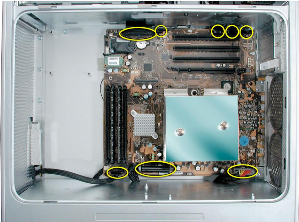
3. Move the cables at the top of the logic board out of the way by temporarily tucking them into the openings in the media bay shelf.
