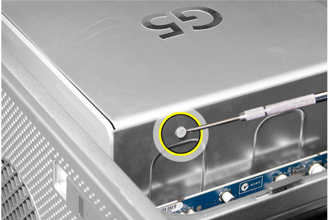
**Replacement Note:** You do not need to replace the rivet after you have replaced the heatsink cover.
