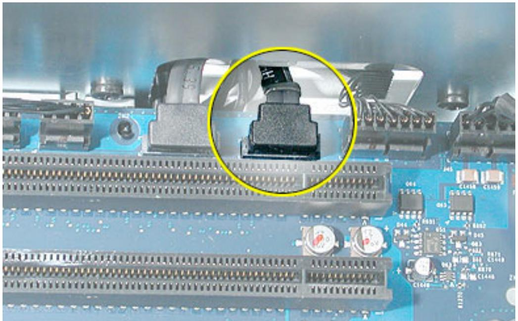
**Replacement Note:** When installing the replacement upper hard drive cable, first route the cable through the opening in the hard drive bay.
