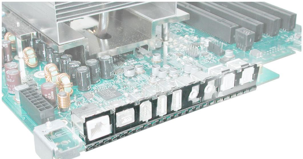
**Replacement Note:** When installing the logic board into the computer, make sure the antenna board shield is not bent back away from the case. The shield should touch the case when the logic board is fully installed.
