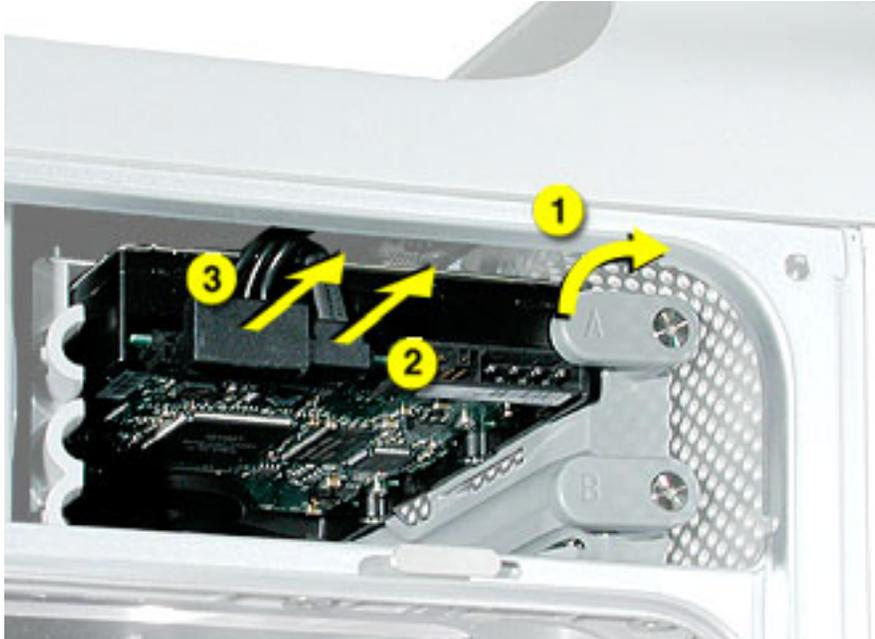
3. Pull the drive out of the drive bay, being careful not to touch the bottom of the drive.
