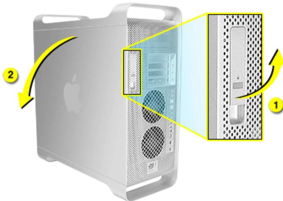
**Replacement Note:** Make sure the latch is in the up position before replacing the access panel. If the latch is down, the access panel will not seat correctly in the enclosure.
