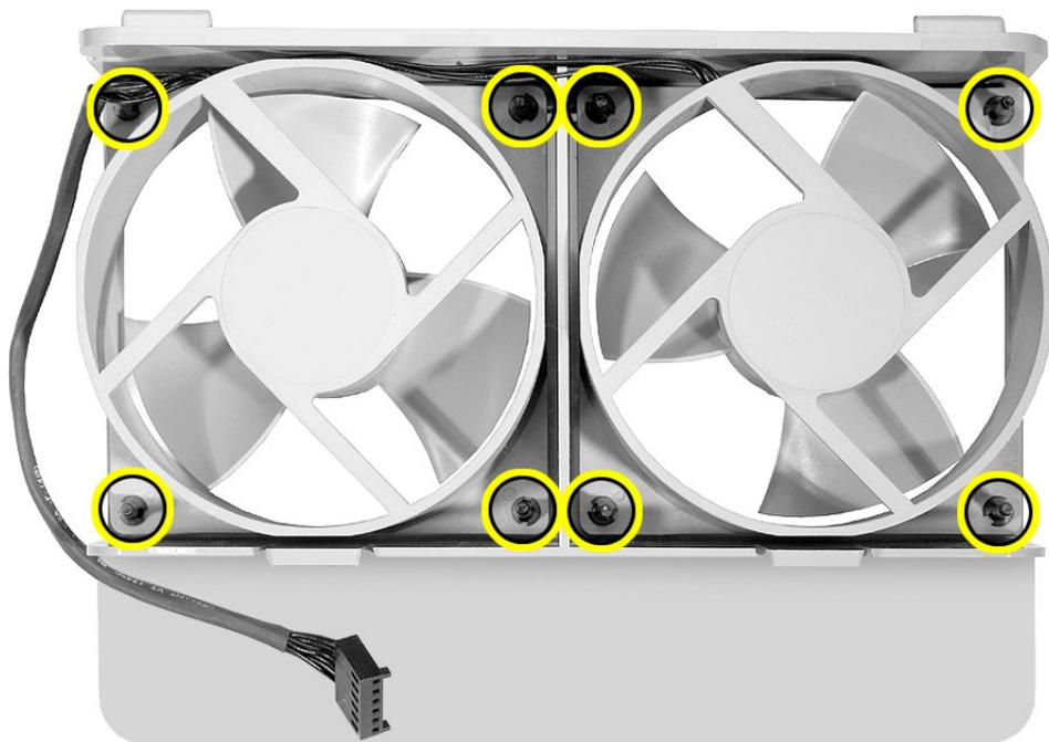
**Replacement Note:** When reinstalling the fan bracket in the enclosure, first connect the fan cable to the logic board. Next, insert the two tabs on the bottom of the bracket into the slots in the enclosure's fan guide.
