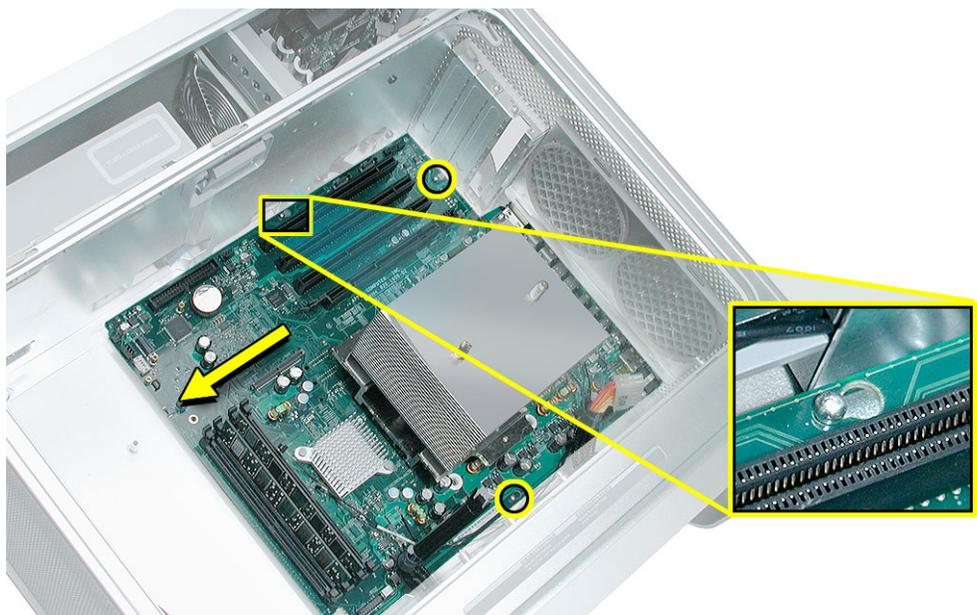
6. Carefully tilt the front edge of the logic board up and maneuver the board out of the enclosure. Place the board on an ESD-safe surface with the processor facing up.
