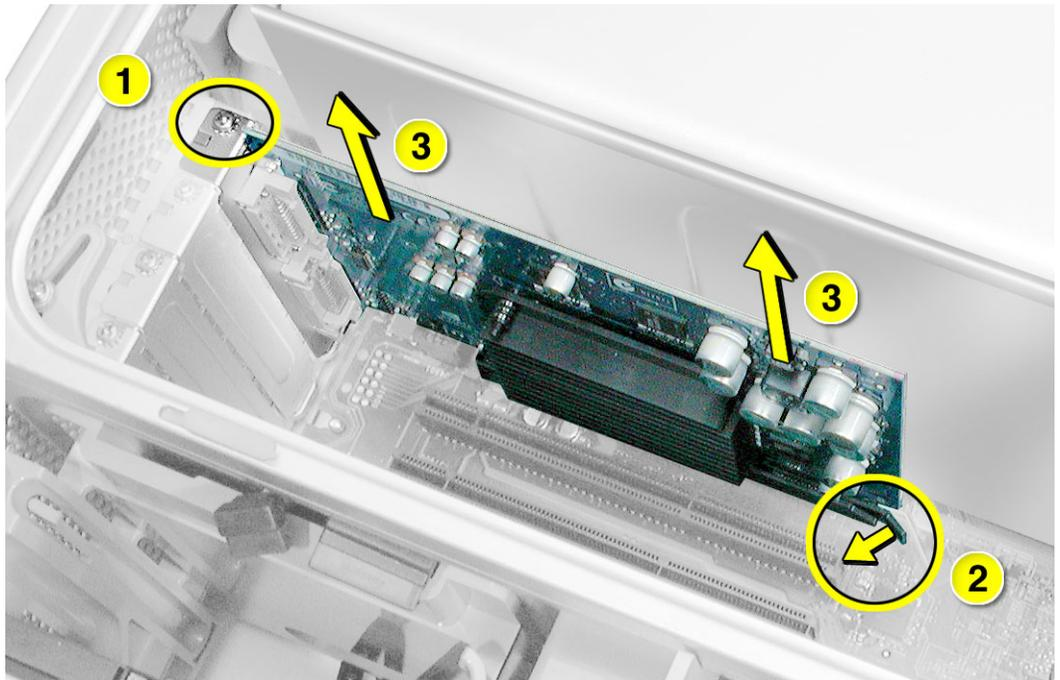
**Replacement Note:** Align the card's connector with the expansion slot and press until the connector is inserted all the way into the slot. If you're installing a 12-inch card, make sure the card engages the appropriate slot in the PCI card guide.
