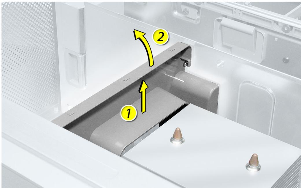
**Replacement Note:** Make sure the inlet frame engages with the mounting pegs on the PCI divider and press down.
