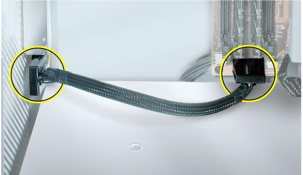
2. Disconnect the cable from the logic board.
