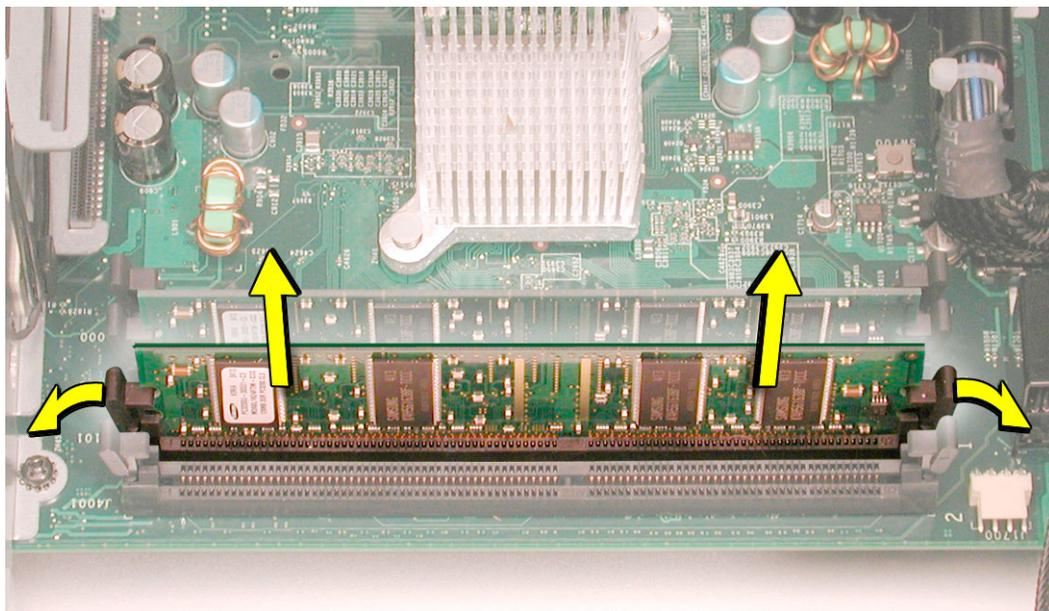
**Replacement Note:** Align the DIMM in the slot and push both ends of the DIMM down until the tabs are vertical and the ejectors snap into place.
