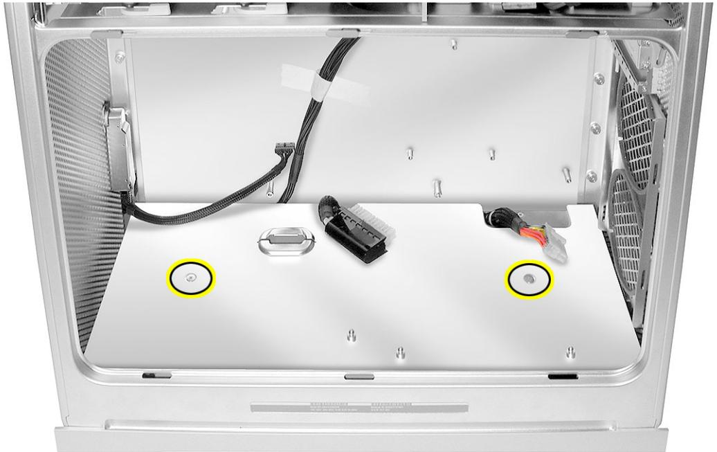
Remove the four power supply mounting screws on the bottom of the enclosure.
