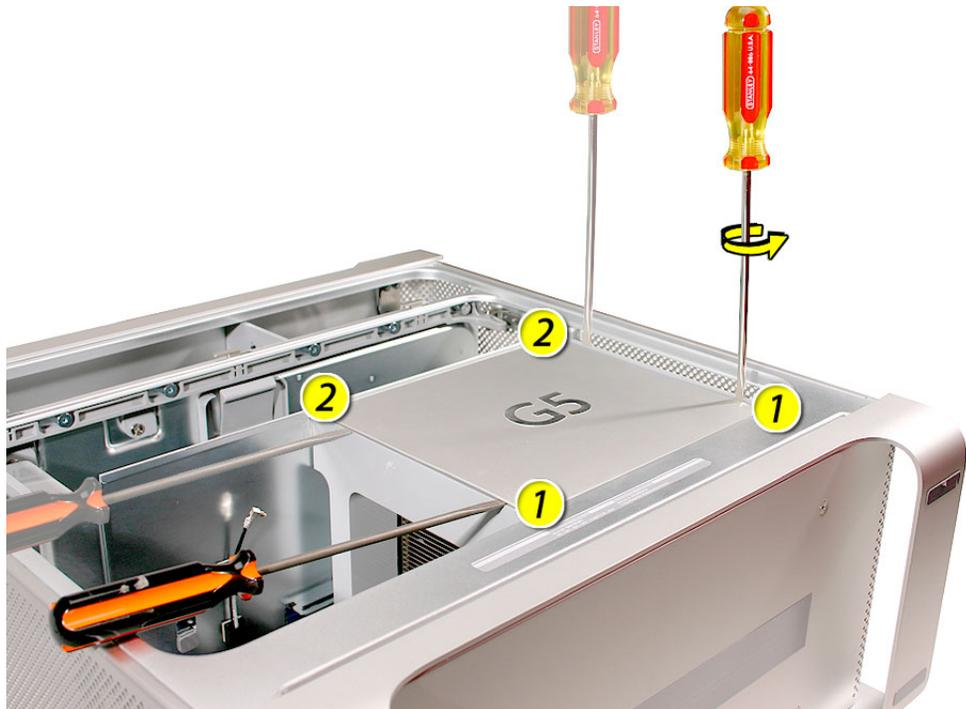
6. Once you feel the latches release, slide the cover to the left a short distance to release it from four metal mounting pegs located under the cover.
