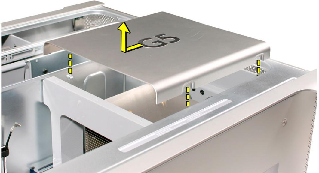
**Replacement Note:** Place the notches in the underside of the cover directly over the four mounting pegs. Slide the cover toward the back of the computer and then press down firmly until you feel the cover lock into place.
