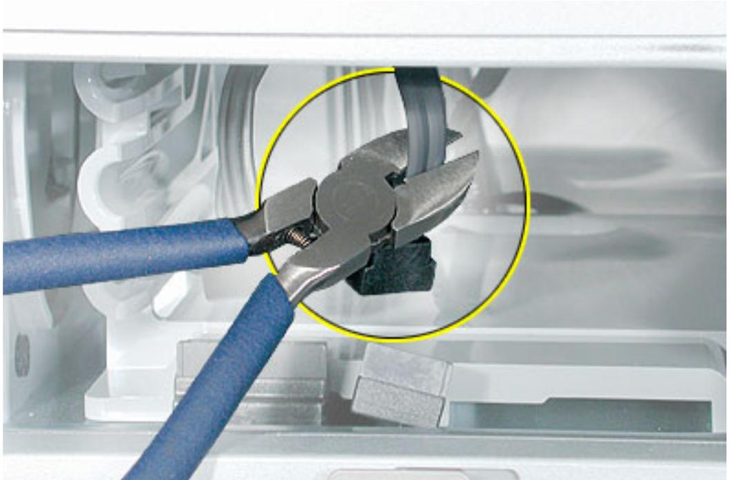
2. Disconnect the cable from the logic board, pull the cable out of the hard drive bay, and remove the cable from the enclosure.
