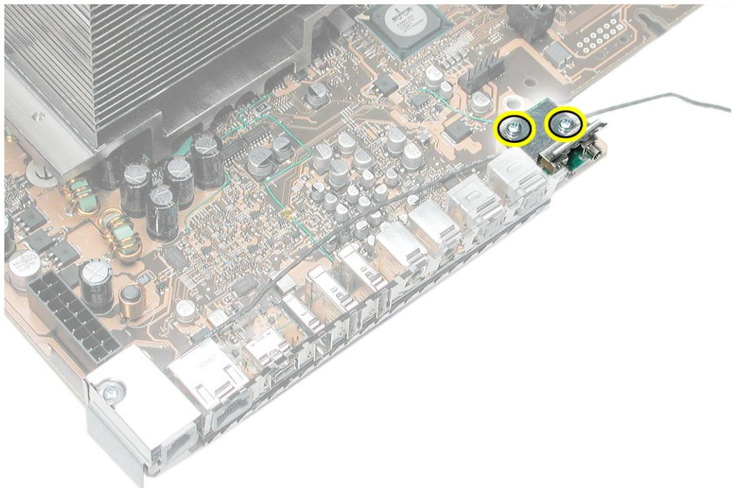
2. Remove the Bluetooth cable (gray) and AirPort cable (black) from the clips on the underside of the logic board.
