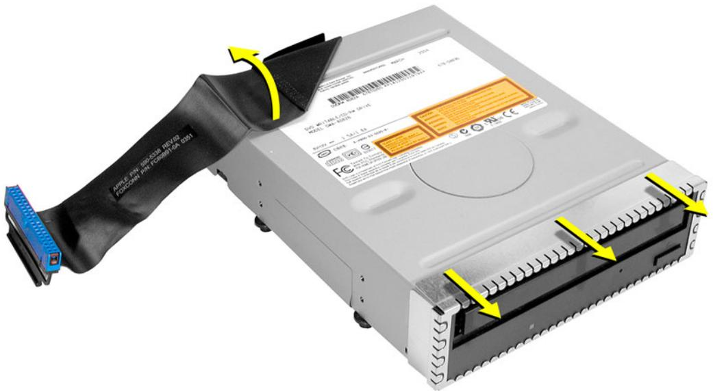
8. Carefully remove the EMI shield from the front of the original drive and transfer it to the front of the replacement drive.
