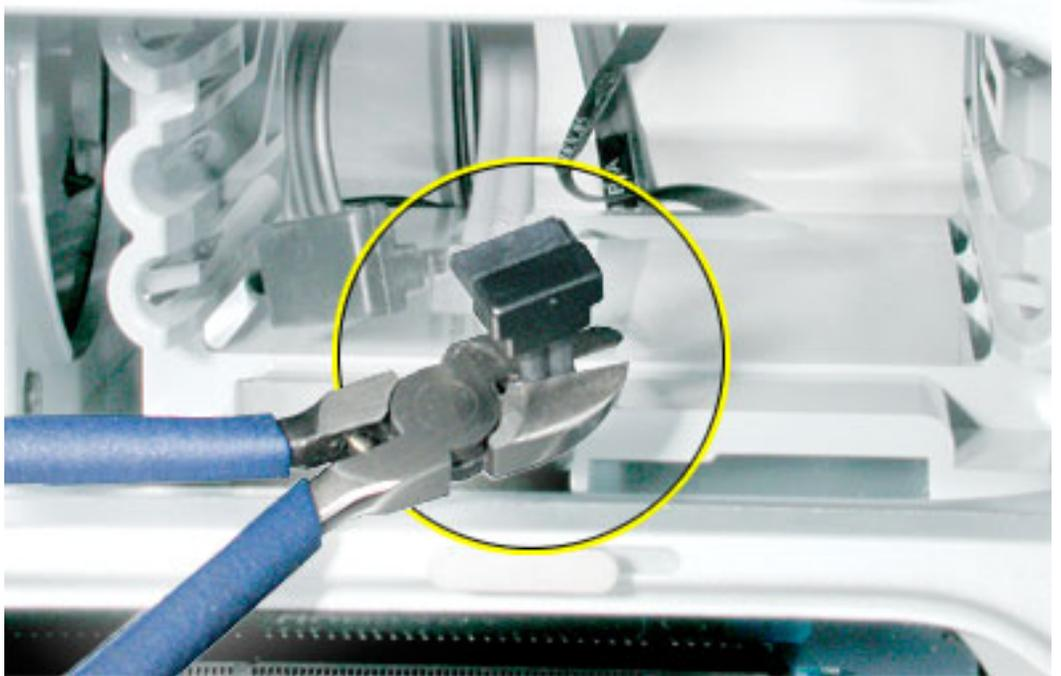
2. Disconnect the cable from the logic board, pull the cable out of the hard drive bay, and remove the cable from the enclosure.
