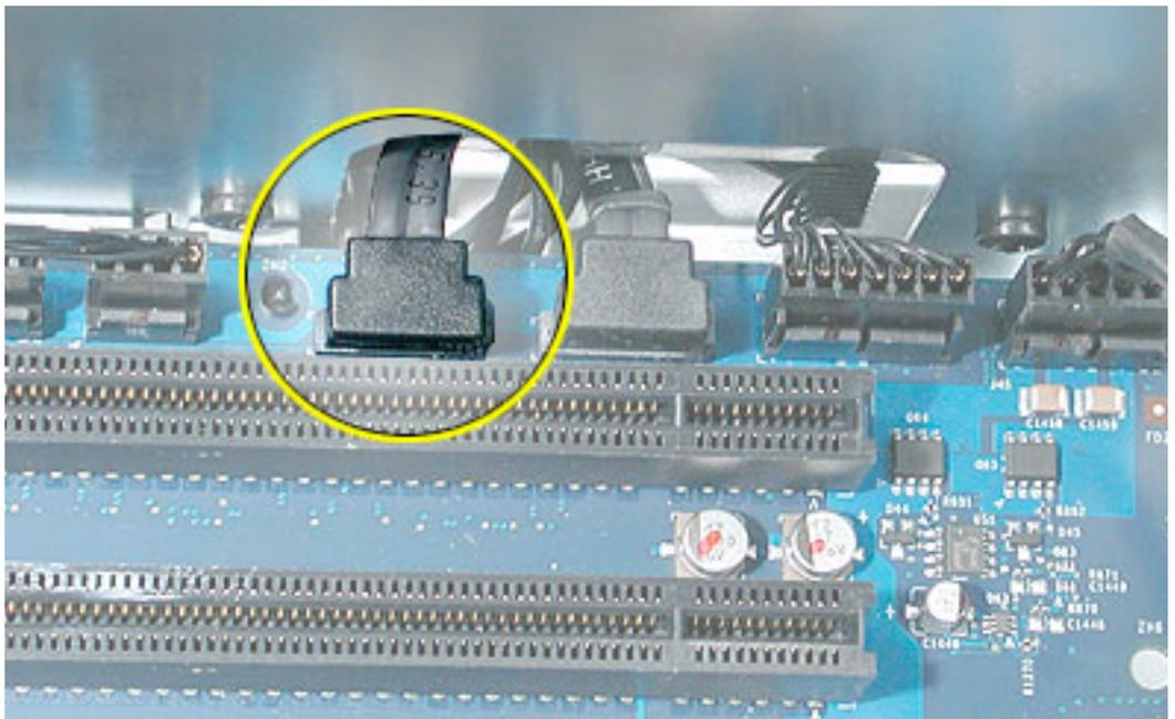
**Replacement Note:** When installing the replacement lower hard drive cable, first route the cable through the opening in the hard drive bay.
