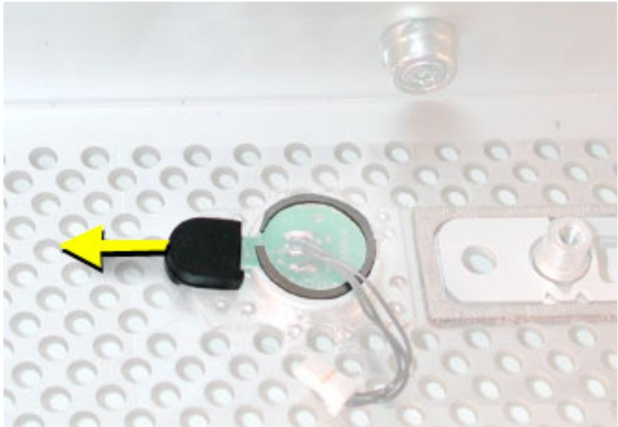
4. Lift up and remove the power button board.
