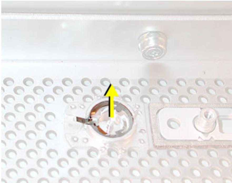
6. Remove the power button from the enclosure.
