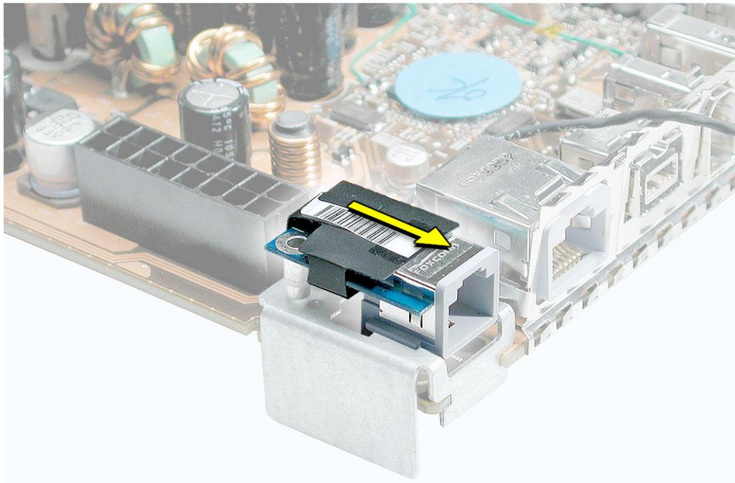
**Replacement Note:** Make sure the modem filter cable routes out through the opening in the side of the modem filter cap before securing the cap to the modem filter board.
