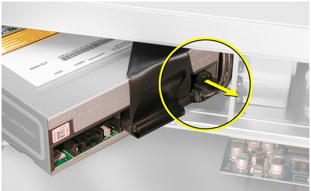
5. Route the drive ribbon cable out through the opening in the media shelf and remove the drive and ribbon cable from the computer.
