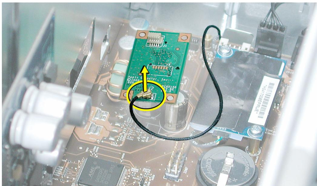
**Replacement Note:** Be very careful connecting the antenna cable to the Bluetooth card. The connector is fragile and can easily be bent.
