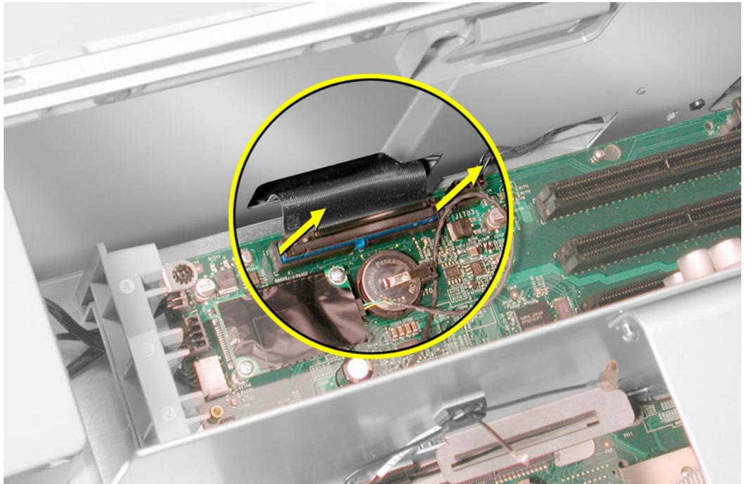
2. Push the optical drive levers out to release the drive.
