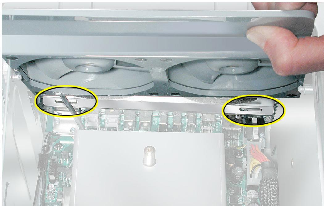
Then rotate the fan back flush with the rear panel, making sure the two latches on the top of the bracket engage with the two slots on the top of the fan guide.
