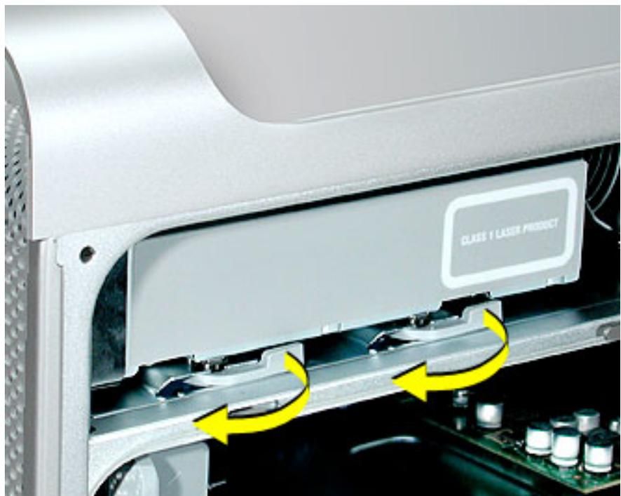
3. Place the fingers on one hand inside the opening for the optical drive cable and push the edge of the drive forward. The drive will move part way out of the media shelf.
