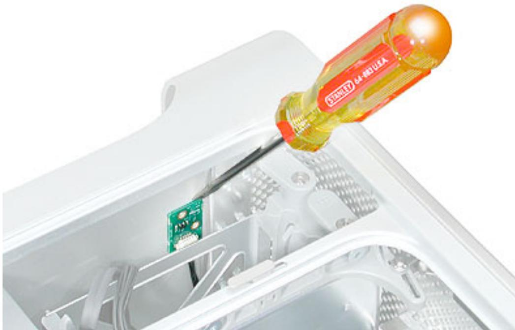
2. Pull the board forward slightly so that you can reach the cable connector.
