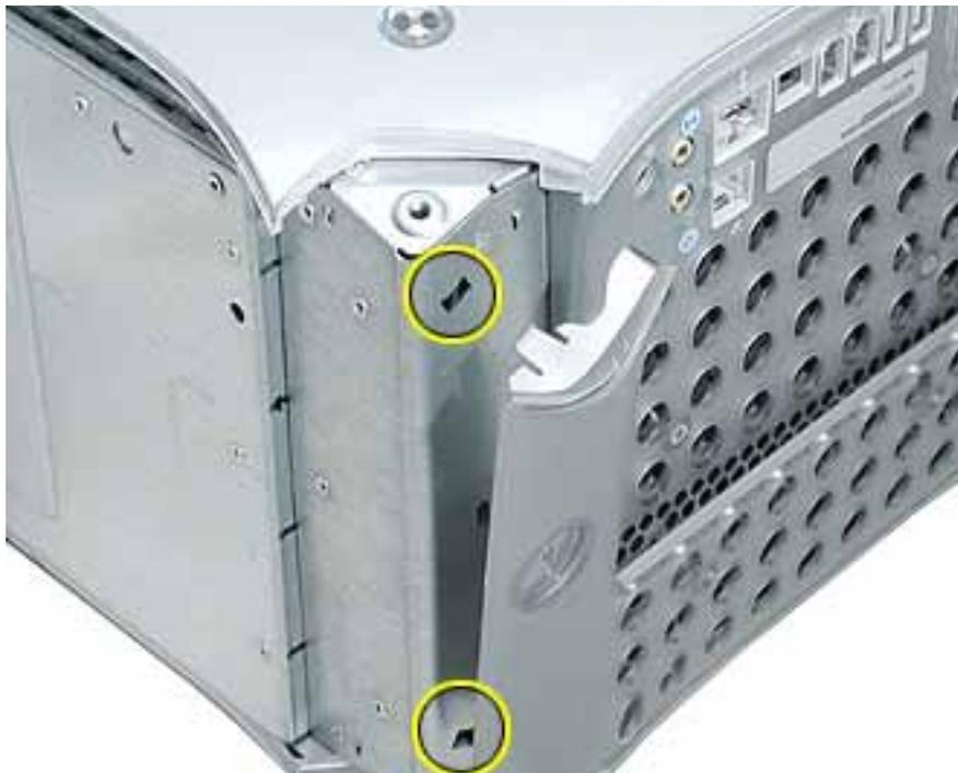
3. Grasp the rear vented panel on both sides of the lockable cover latch, and forcefully pull off the rear vented panel.
