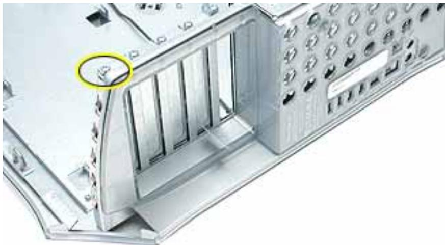
3. Use a flat-blade screwdriver to pry up the hooked tabs from the slots in the chassis. Pull that end of the I/O panel forward.
