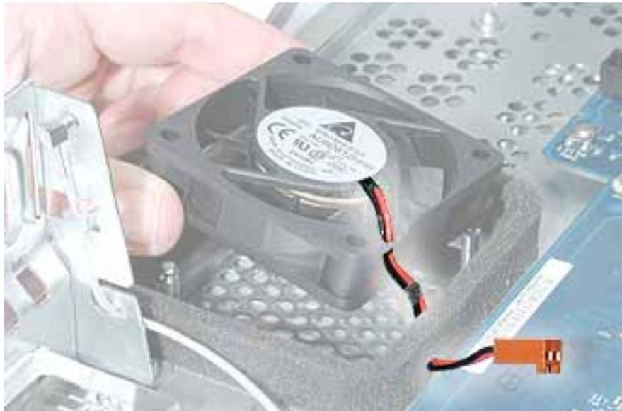
**Replacement Note:** If the foam wall is damaged, replace it by peeling off the old foam and cleaning the chassis surface with an alcohol wipe. Then apply the new foam wall to the chassis.
