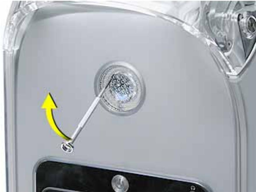
**Replacement Note:** Press the replacement speaker grill into the speaker opening.
