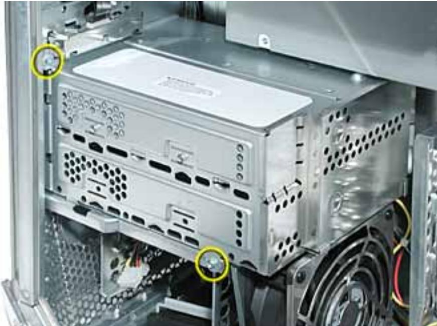
3. Slide the back panel off the carrier.
