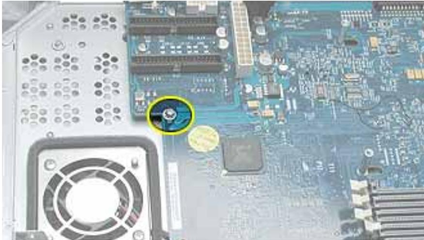
3. Slide the logic board toward the front of the computer to clear the chassis hooks.
