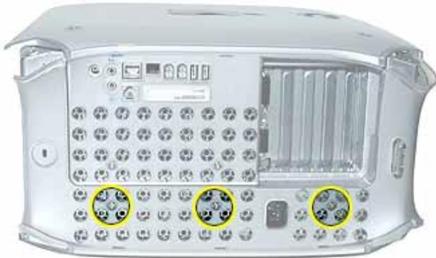
2. Use a flat-blade screwdriver to pry out the tabs from the lower chassis.
