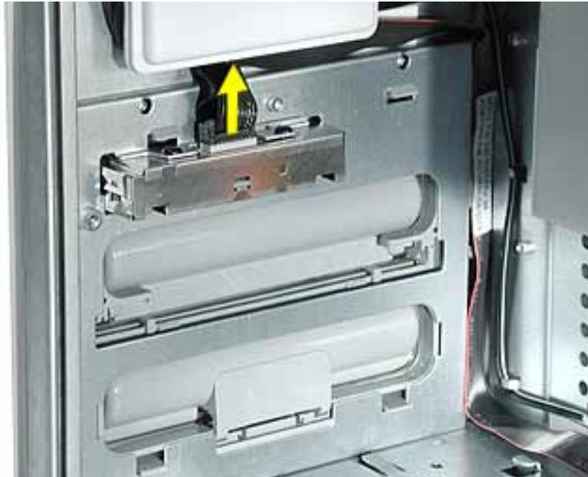
2. Peel the front panel board cable from the recessed channel in the side chassis and route the cable through the opening in the optical drive shelf.
