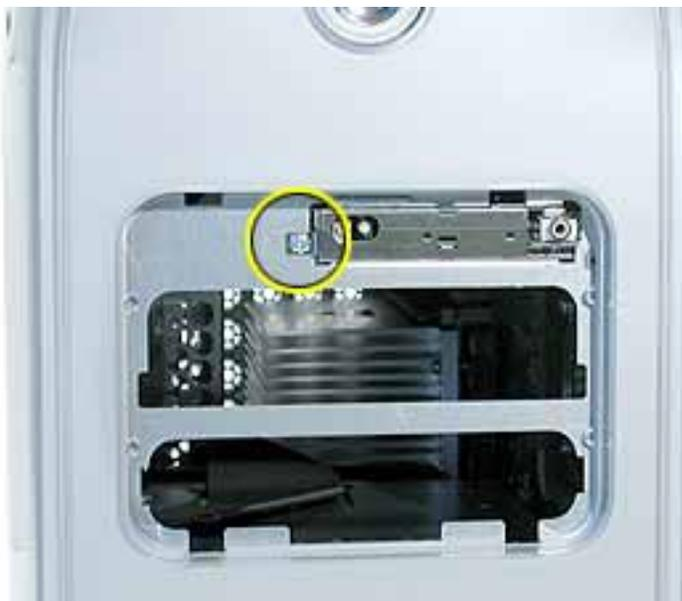
4. Remove the front panel board through the front opening in the computer.
