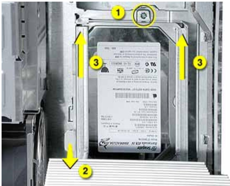
3. Rotate the carrier back from the chassis far enough to reach the drive cables. Disconnect the hard drive data and power cables (P2 and P3) from the hard drive(s).
