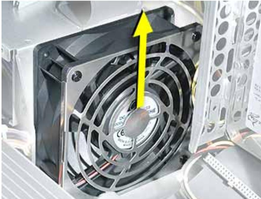
**Replacement Note:** Align the fan with the three latches in the drive shelf and slide straight down until you feel the fan lock into place.
