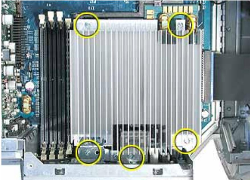
2. Lift the heatsink straight up and remove it from the computer.
