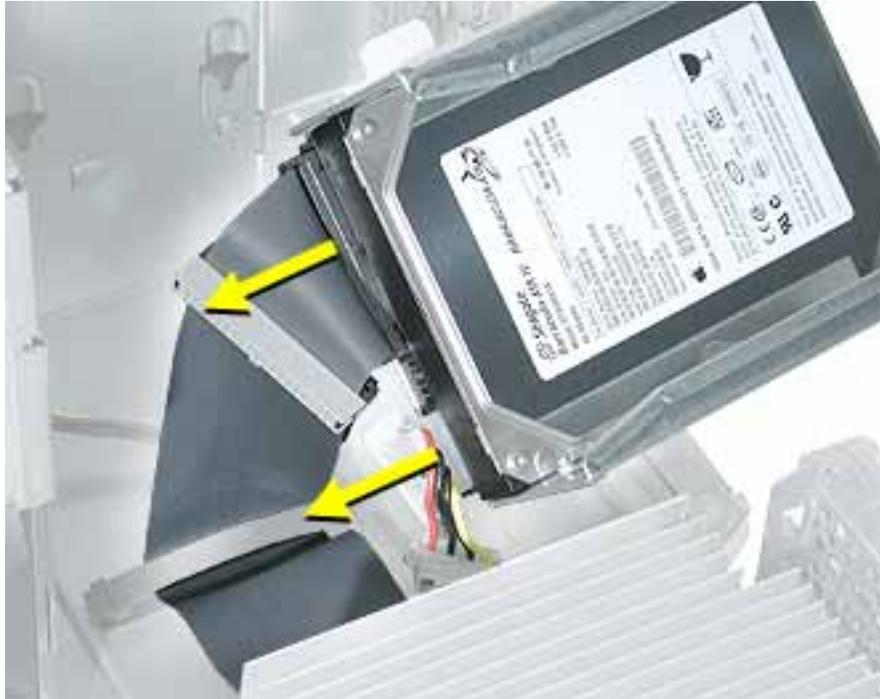
4. Remove the carrier and drive(s) from the computer.
