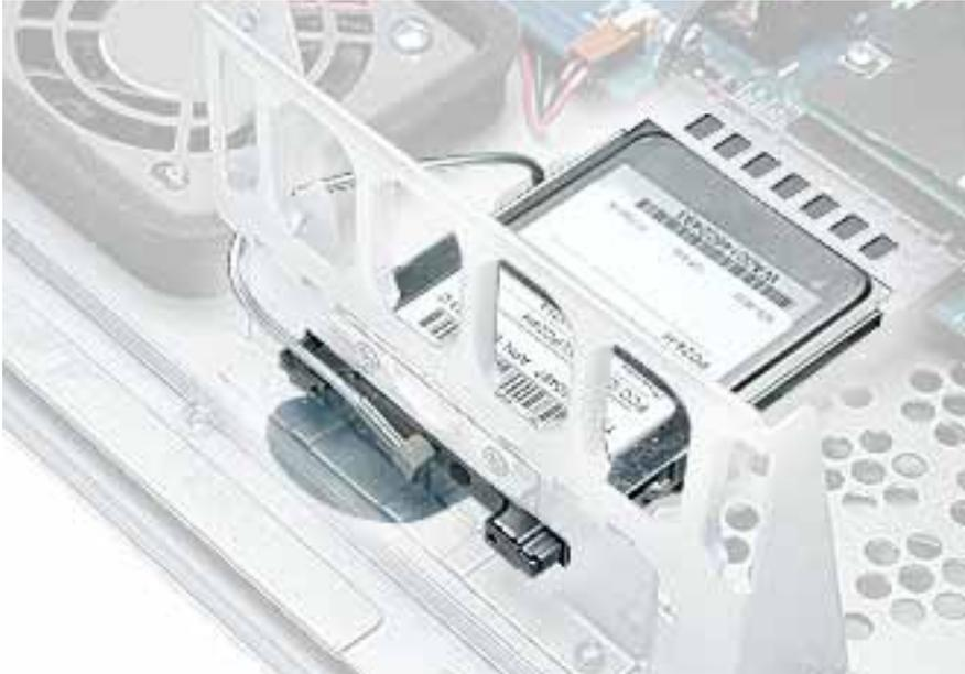
2. Pull the clear plastic tab on the AirPort Card to disconnect the card from the connector on the logic board.
