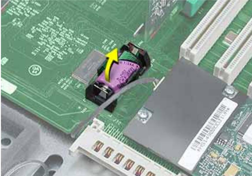
**Note:** When replacing the battery, make sure the positive (+) end of the battery aligns with the + symbol on the battery holder.
