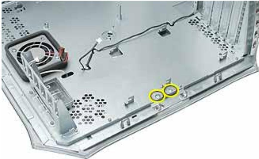
4. Using needlenose pliers, squeeze the plastic tabs (protruding through the chassis), to release the right side panel from the metal chassis.
