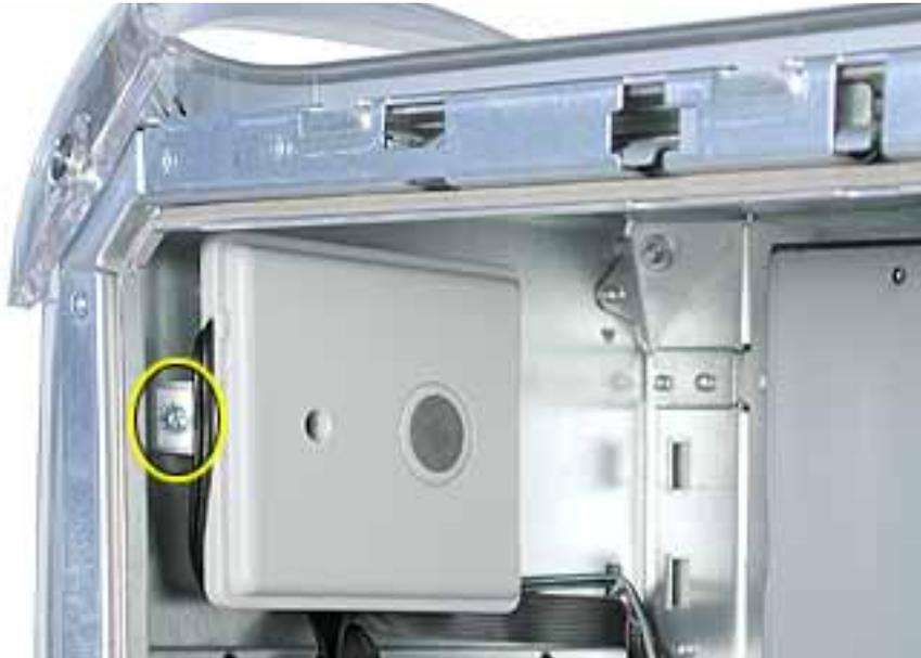
5. Swing the speaker away from the chassis. Press in on the two latches on the right side of the speaker and release the speaker from the chassis.
