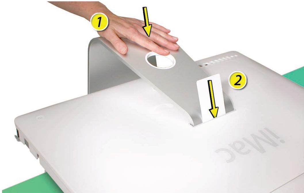
2. Insert the card as far as it will go, and press the stand down until you hear a click—the audible cue that tells you that the stand is locked into place.
