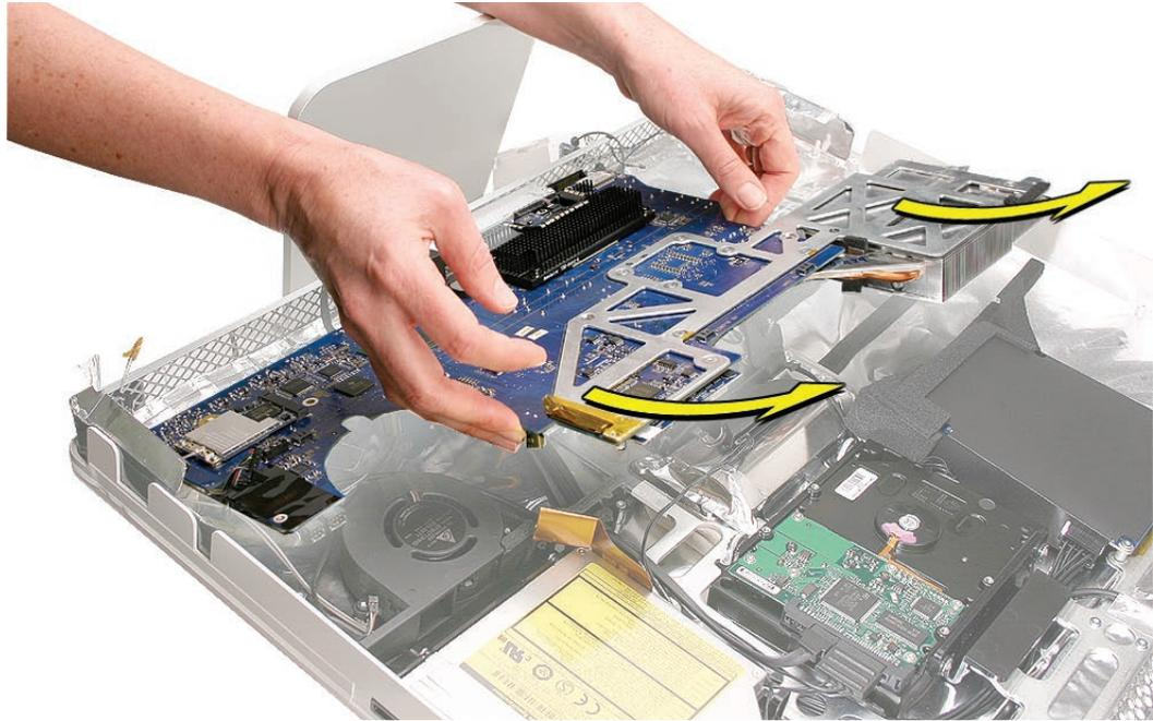
7. When the board is removed, check that the two washers on the processor side of the logic board did not fall off.
