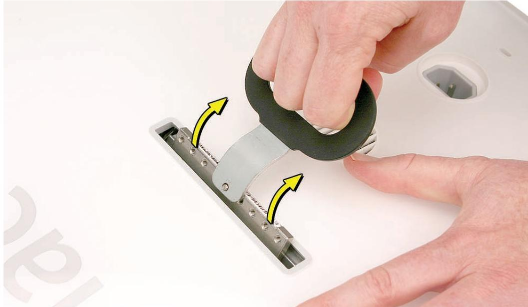
14. The clutch mechanism is now locked into place and ready to accept the installation of the stand or VESA mount.
