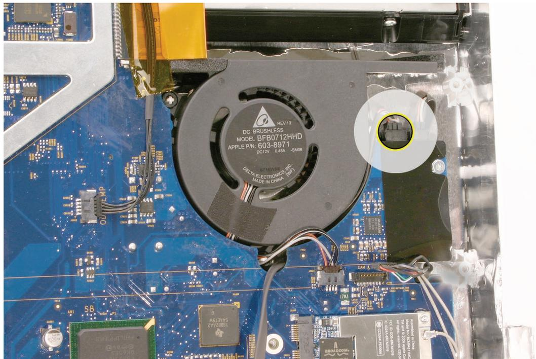
5. Route the speaker cable between the fan and logic board and out from underneath the optical fan cable.
