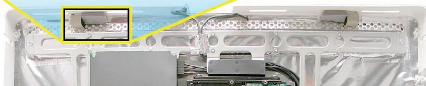
2. At the top of the rear cover, pry up the left antenna board with a black stick and carefully peel up the EMI shielding to unroute the left antenna board and attached gray cable.
