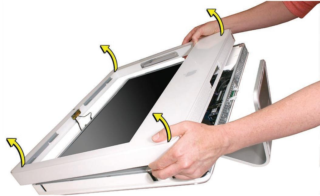
5. Lift up the top of the bezel and notice the connected microphone and camera cables. Without straining the cables, hold the bezel up, and disconnect the camera cable from the camera board and the microphone cable from the cable extension.
