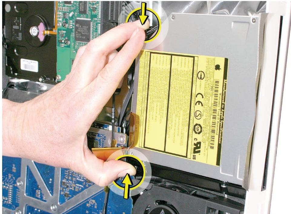
6. Peel back the strip of EMI mesh tape that anchors the bezel end of the drive to the rear cover.
