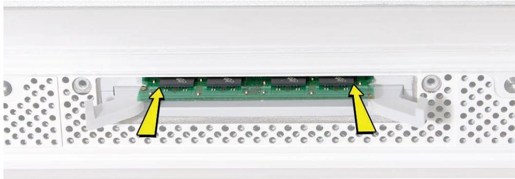
4. Do not use the DIMM levers to push in the DIMM. Trying to push the DIMM into the slot using the levers may damage the SDRAM DIMM. You'll hear a slight click when the memory is fully seated. After the memory is fully seated, close the levers.
