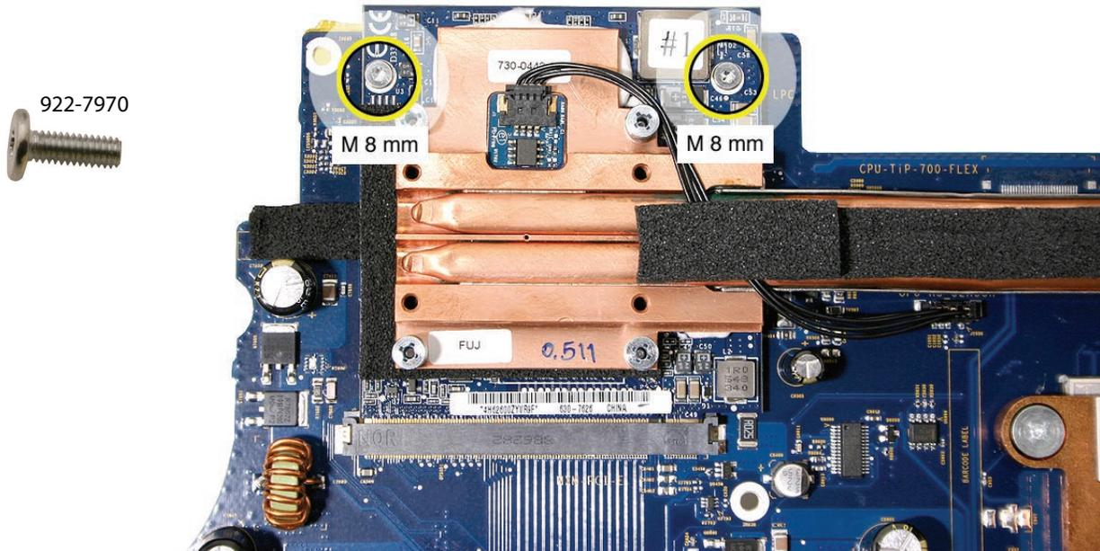
2. At the far right end of the video card heatsink, remove the 4-mm long support screw.
