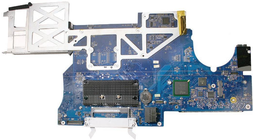
3. Check the board for two spacers. If they are not already present, install the spacers and aluminum tape on the logic board (see steps 3-6). If they are present, go on to step 7.
