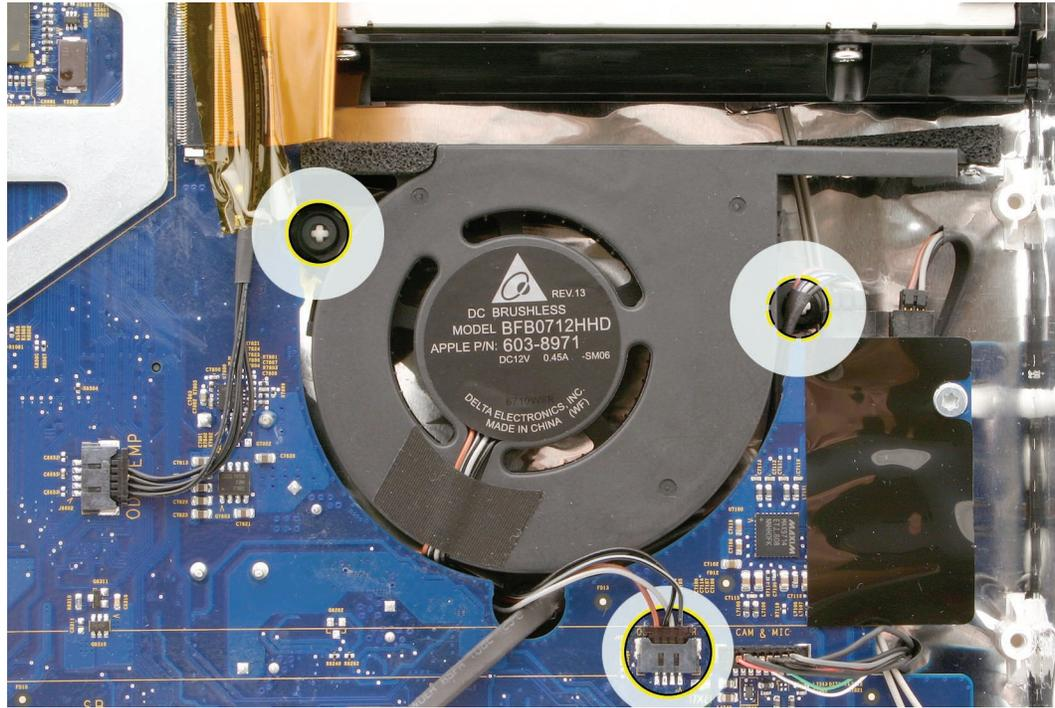
3. Holding the top edge of the fan, pull the body of the fan off of the guide posts on the rear cover.
