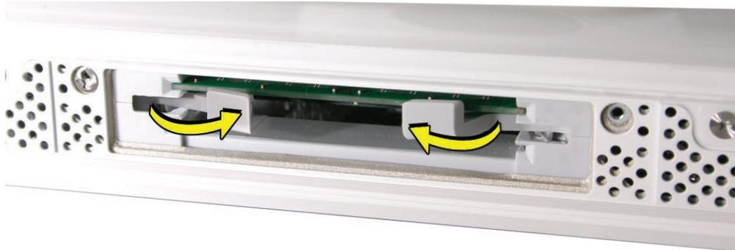
5. Replace the access door on the memory compartment.
