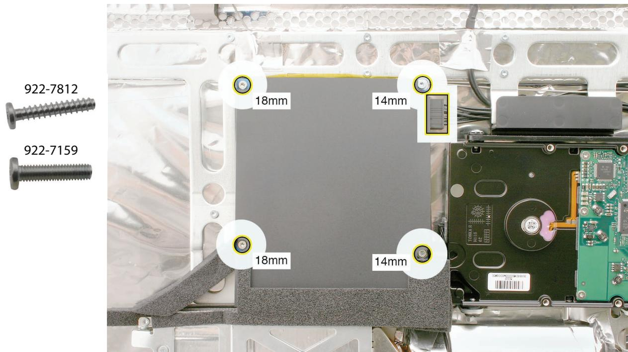
3. Position the computer assembly so you can see under the right side of the power supply. Tilt the power supply slightly and see how the adhesive plastic at the lower right corner of the body connects the power supply to the foam gasket and chassis. Use a black stick to wedge between the plastic and the chassis and pry up the lower corner.
