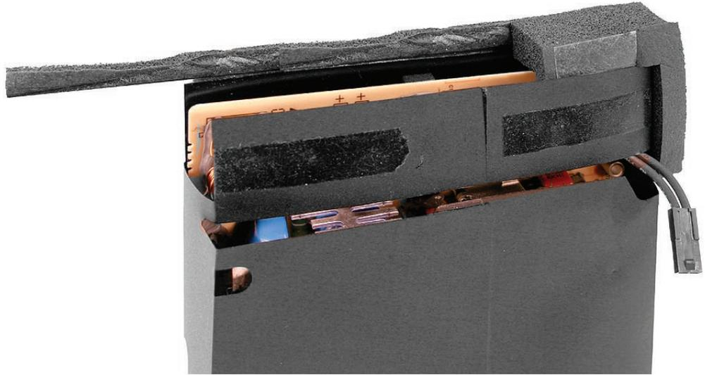
3. On a new power supply, make sure the L-shaped foam gasket completely covers the lower right corner of the power supply.
