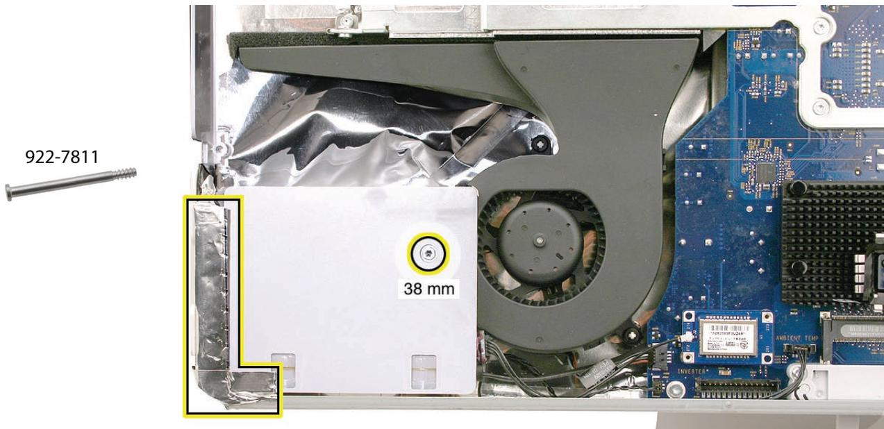
2. Remove the body of the left speaker, and, without straining the speaker cable, rest the speaker on the table.
