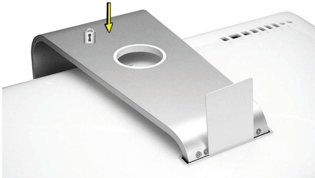
3. Remove the access card, and remove the eight T10 clutch-to-stand screws.
