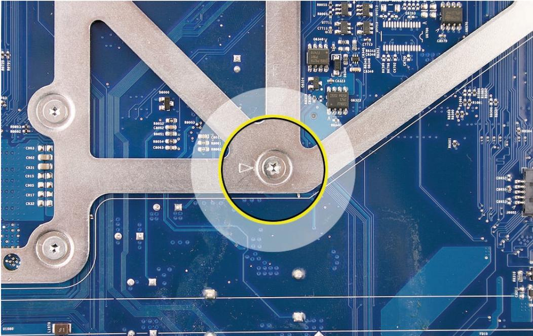
4. Remove the two screws at the support bracket.
