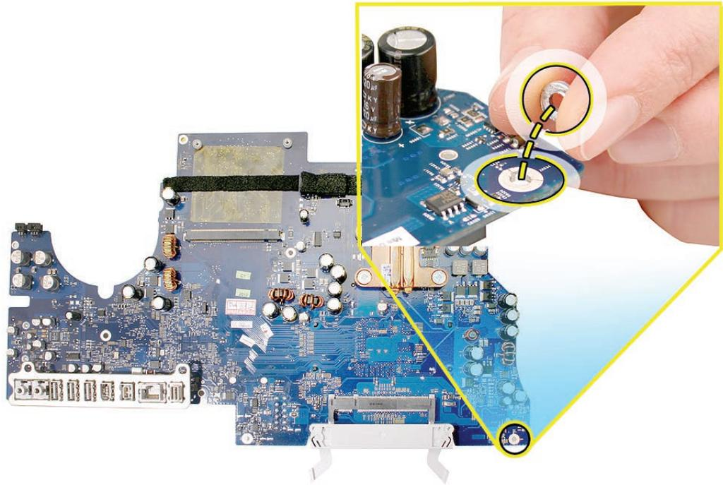
5. The second spacer and the strip of aluminum tape are installed on the white screw post in the rear housing at the location circled below.
