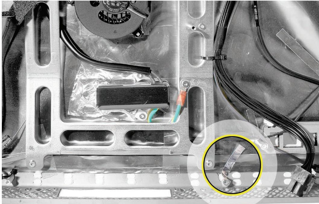
6. Place the second spacer on top of the white screw post in the rear housing.
