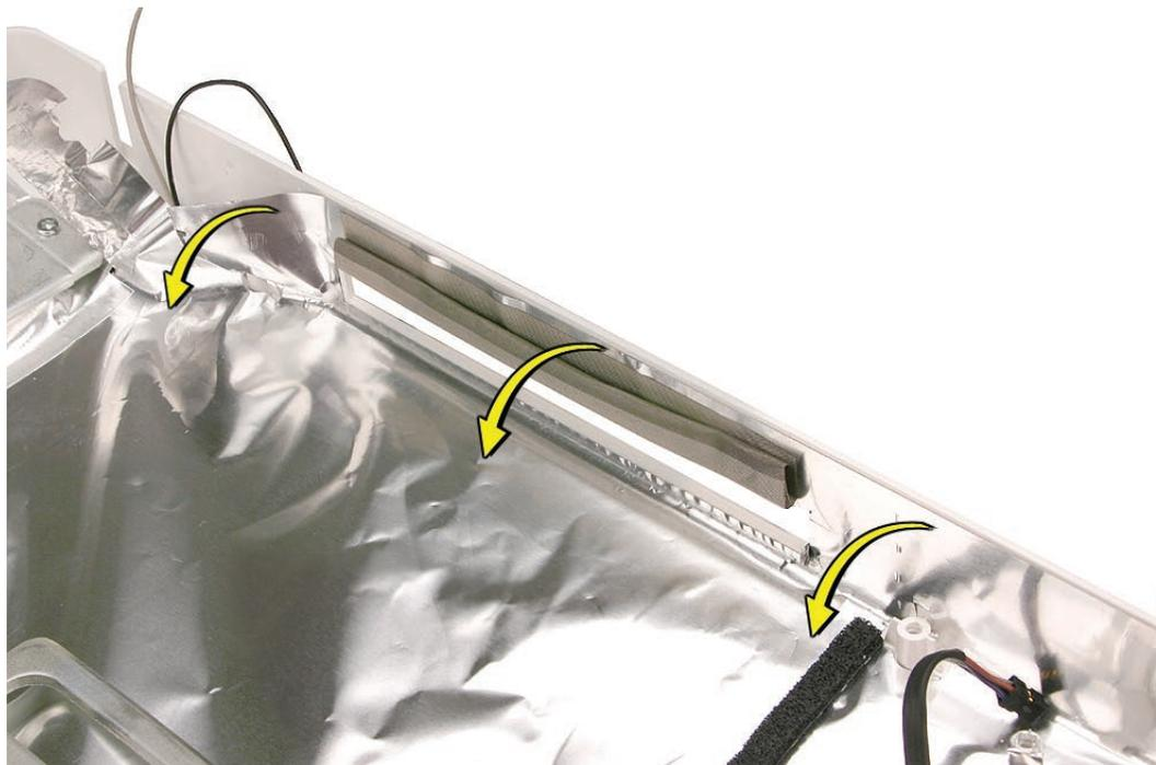
7. Underneath the EMI shielding at the slot-load opening, peel up the two clear strips of tape that secure the antenna cables directly to the rear cover. Do not tug on the cables.
