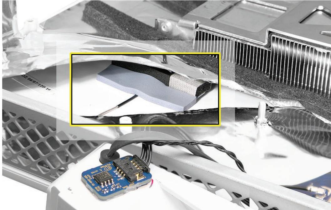
3. Close the EMI sleeve, and secure the opening with a strip of EMI tape.
