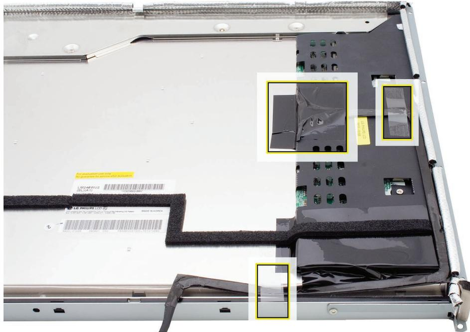
2. Grasp the inverter cable close to the connector and disconnect it from the inverter board.
