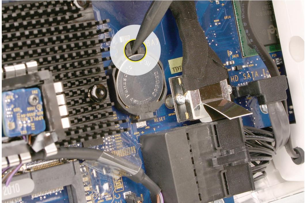
2. Before installing the battery, make sure the side with the engraved markings (+ side) is up.
