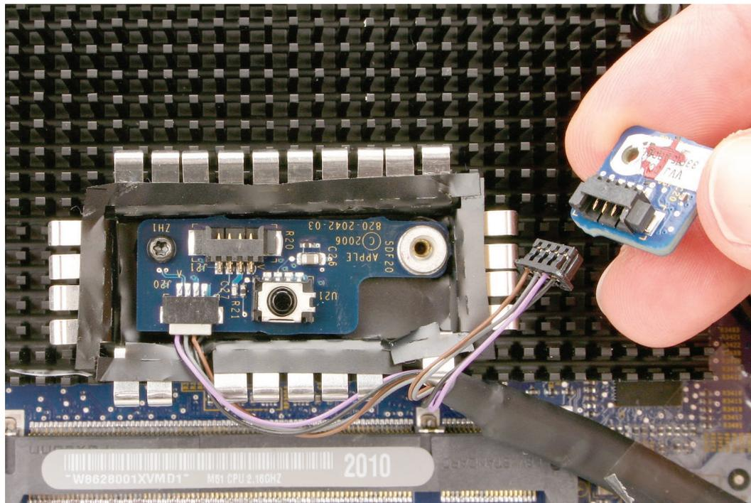
3. Lift out the IR board and disconnect the cable from the IR board.
