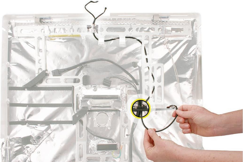
2. At the top of the rear cover, peel back the tape that secures the cable onto the chassis.
