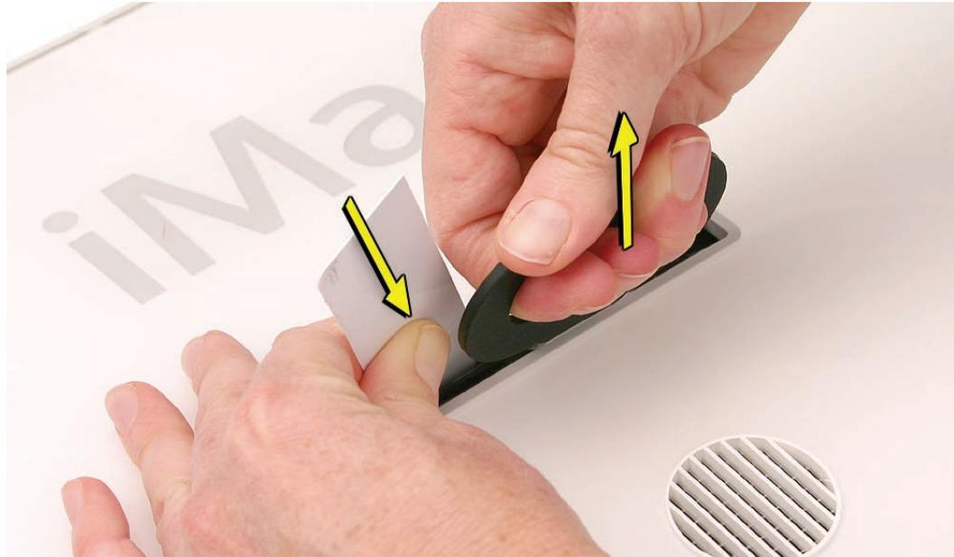
12. When you can pull up the clutch mechanism and easily see it emerge through the slot, maintain the pull force on the clutch mechanism retrieval tool, but remove the access card.
