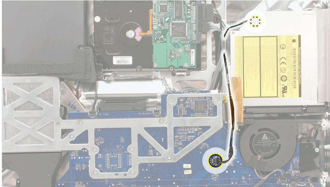
2. Disconnect the cable from the sensor on the top edge of the optical drive.
