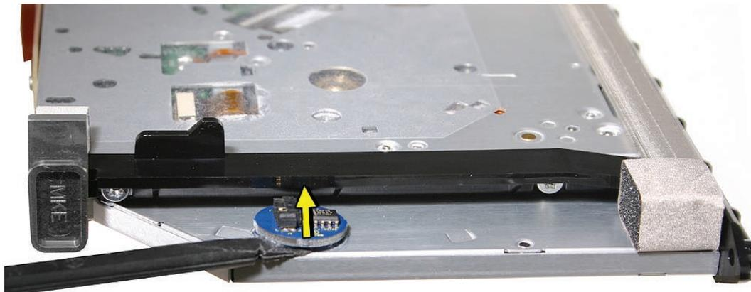
10. If you are replacing the optical drive, transfer the flex cable (two 4-mm long T6 shoulder screws) and sensor to the replacement drive. The replacement drive includes the plastic mounting brackets, slot-load bezel, and gaskets.
