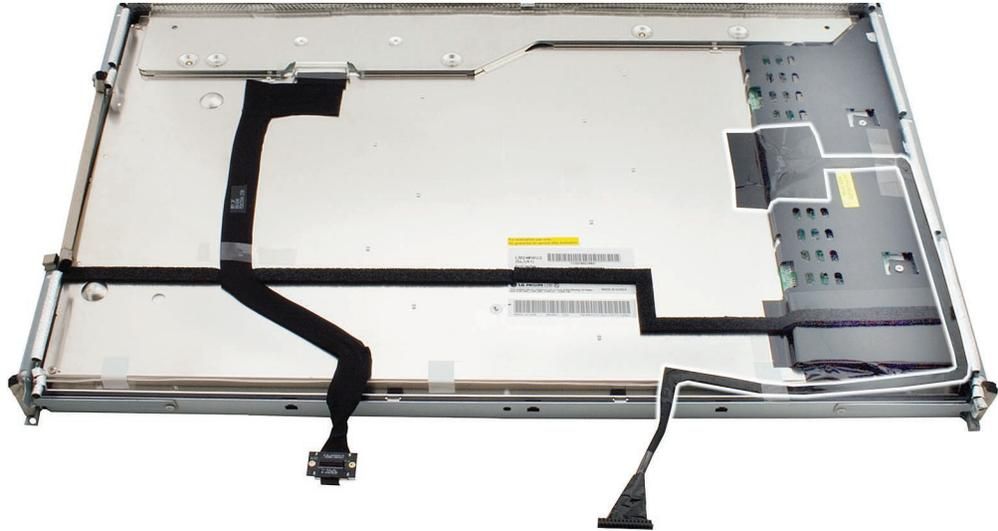
3. Make sure the tape at each lower corner is back far enough so it cannot be pinched as you lower the LCD panel into the computer assembly.
