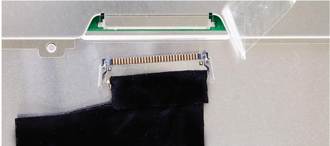
2. Replace the tape over the LVDS cable connector.
