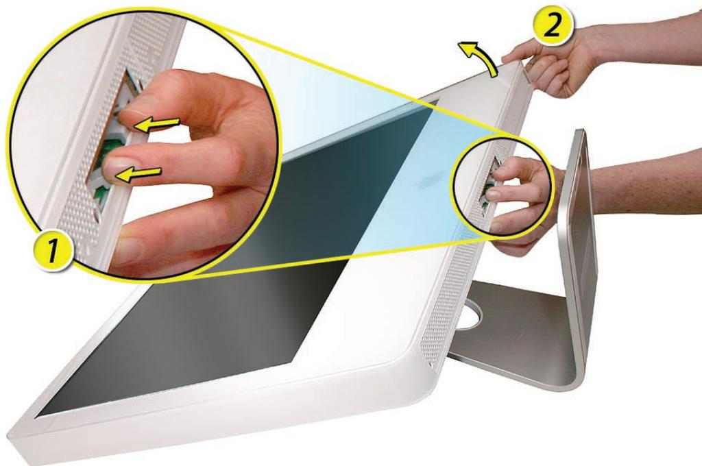
4. With the lower corners loosened, lift up—but do not remove—the bezel.
