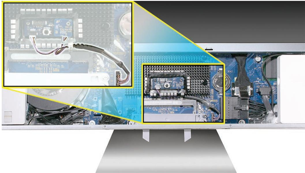
2. Position the shield over the logic board and install the two screws.
