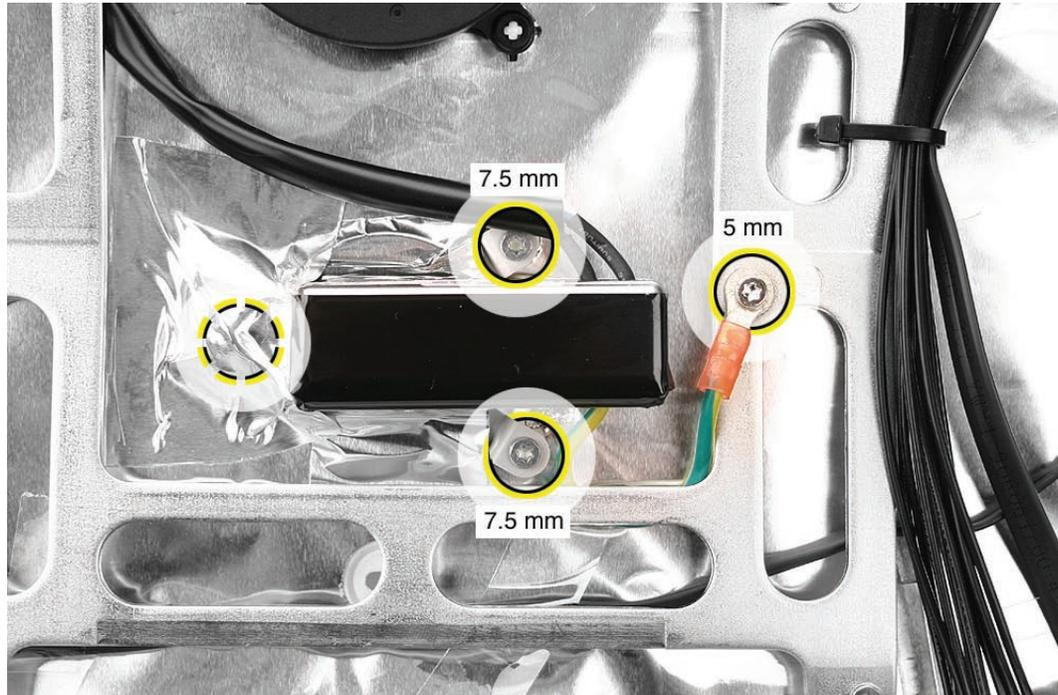
6. Replace the power supply, and connect the AC power inlet cable.
