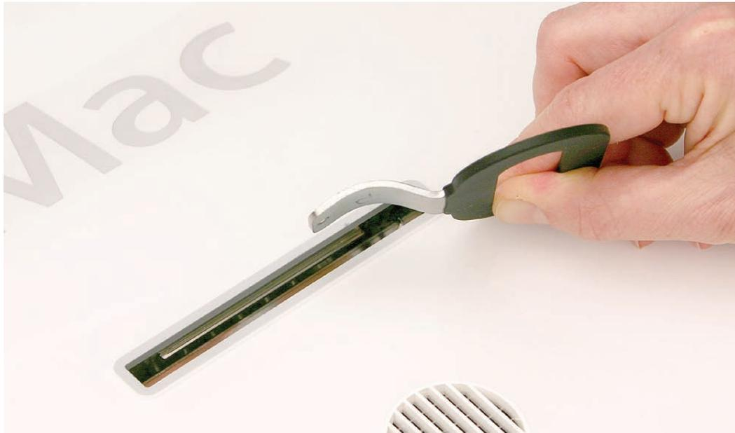
8. Note that the small round opening on the end of the clutch mechanism retrieval tool must hook onto the pin on the recessed clutch mechanism.
