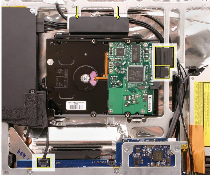
4. Tilt out the hard drive from the computer assembly.
