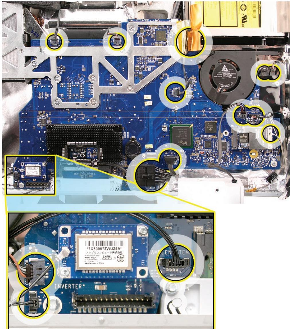
2. Remove the eight T10 screws from the logic board.
