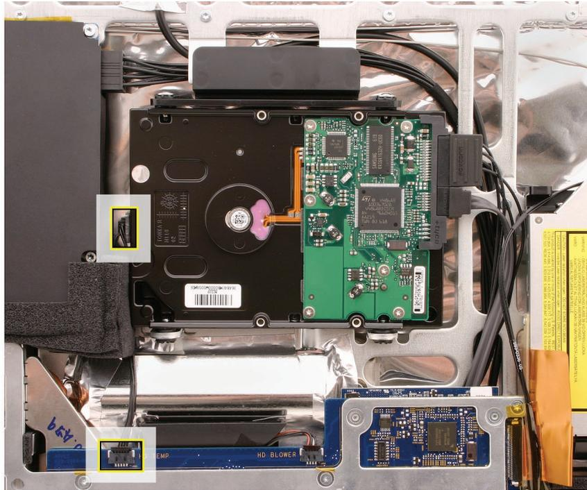
2. Remove the sensor cable from under the foam gasket on the power supply.
