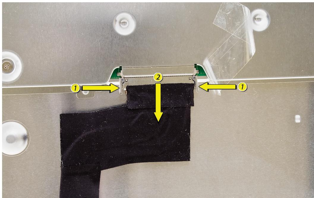
3. Lift the LVDS cable from the display panel.
