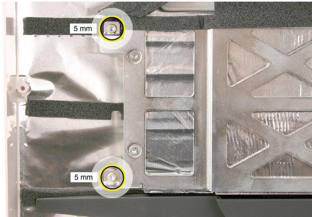
5. Peel up the power supply gasket material where it overlaps the backer plate.
