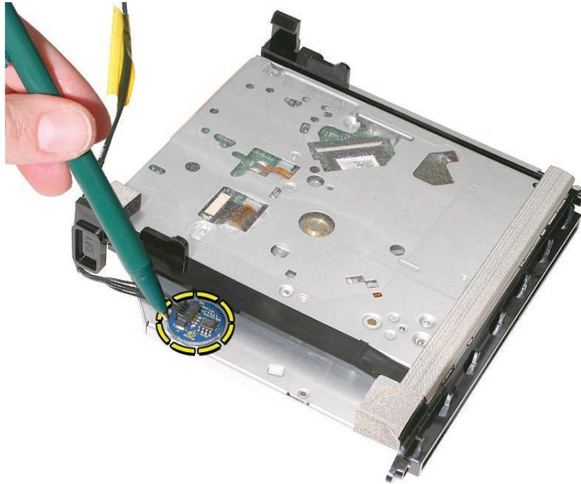
2. Use a black stick to peel up the temperature sensor from the adhesive on the bottom of the drive.
