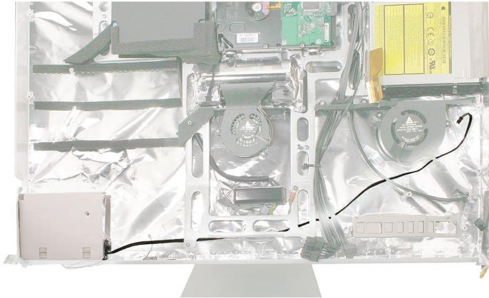
7. With the logic board removed, peel up the tape that secures the speaker cable between the chassis and the EMI shielding.
