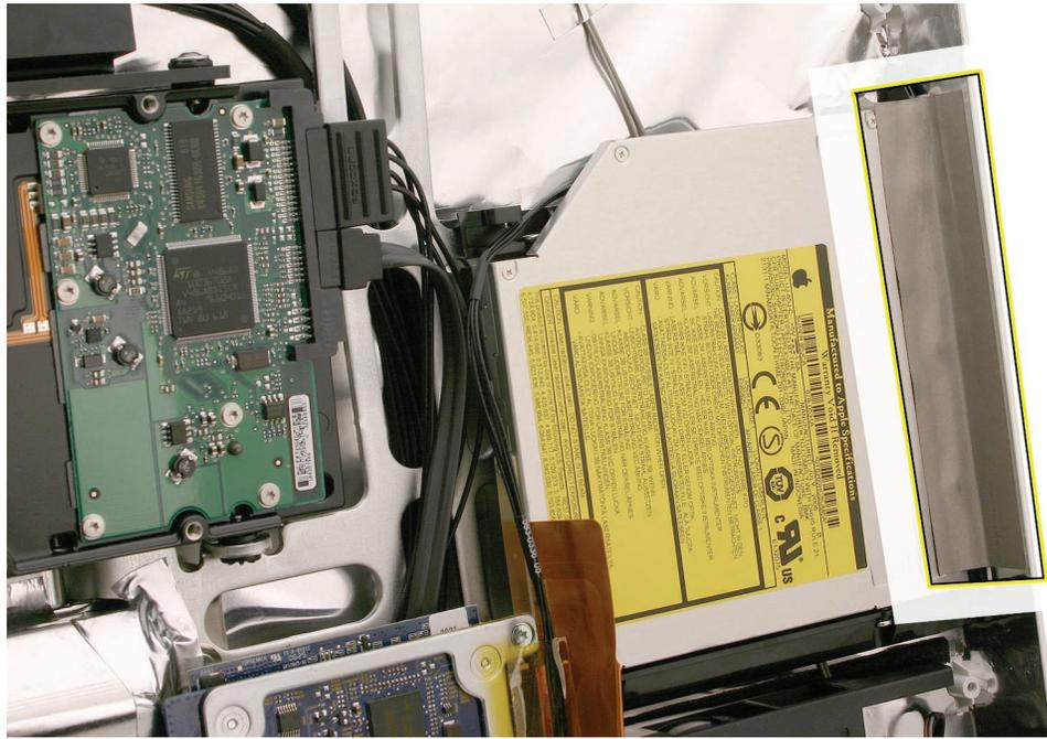
7. Tilt up the optical drive, and lift it out of the computer assembly.
