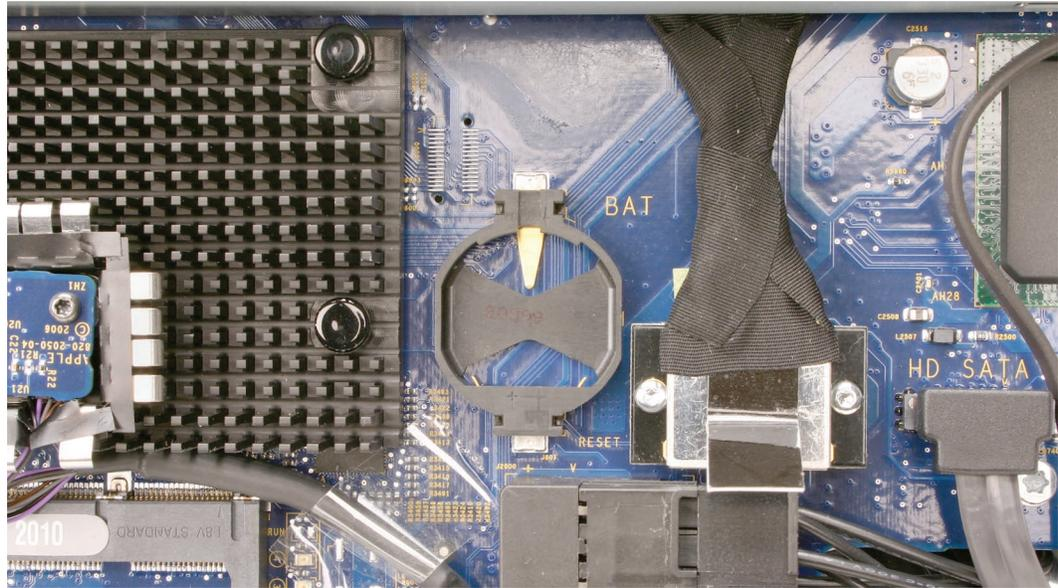
2. Press the battery into the socket. While holding the memory eject levers closed, replace the front bezel.
