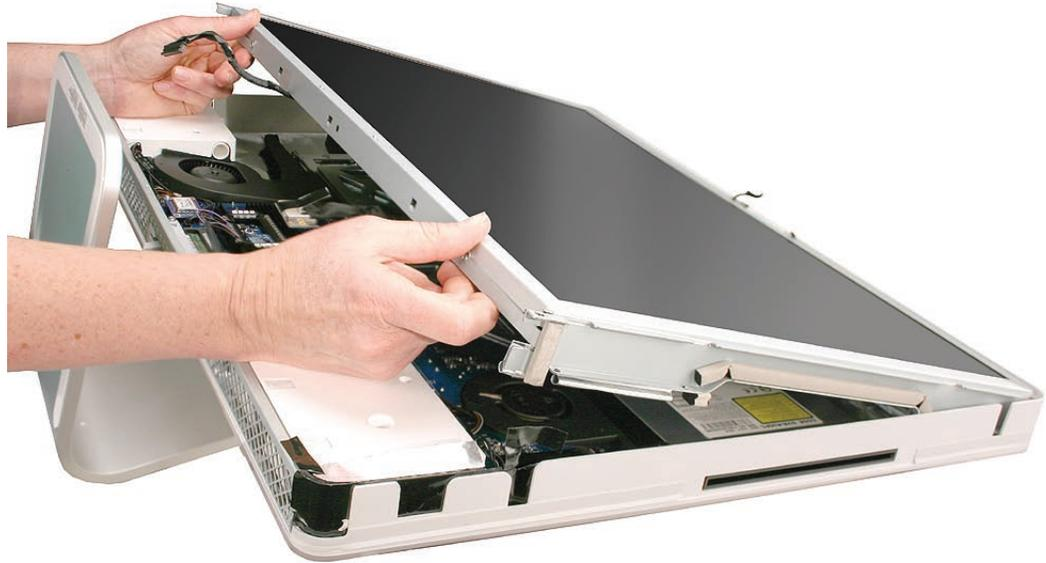
7. **Note:** If replacing the display panel, disconnect the LVDS cable from the panel and the inverter cable from the inverter board before returning the module to Apple. Transfer the two cables to the replacement panel. A replacement panel includes the inverter board, both display panel mounting brackets, the EMI strip surrounding the panel, and the foam strip and gaskets, as shown below.
