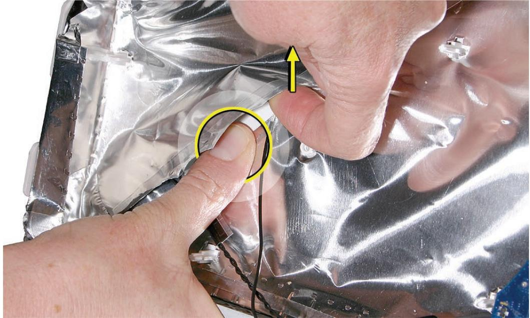
5. Use a black stick to pry up the rectangular end of the antenna from the rear housing. Pull the remaining antenna cable through the opening in the EMI sleeve.
