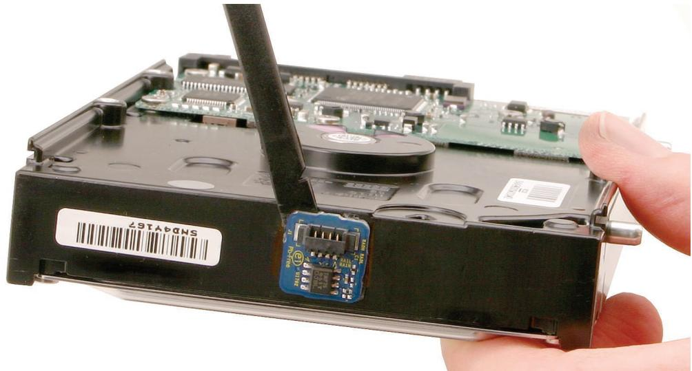
8. At the lower side of the drive, remove the two screw pins.
