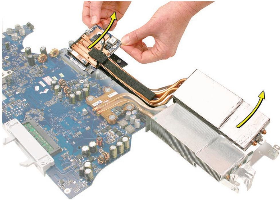
4. When handling the video card, hold it by the heat pipe brace.
