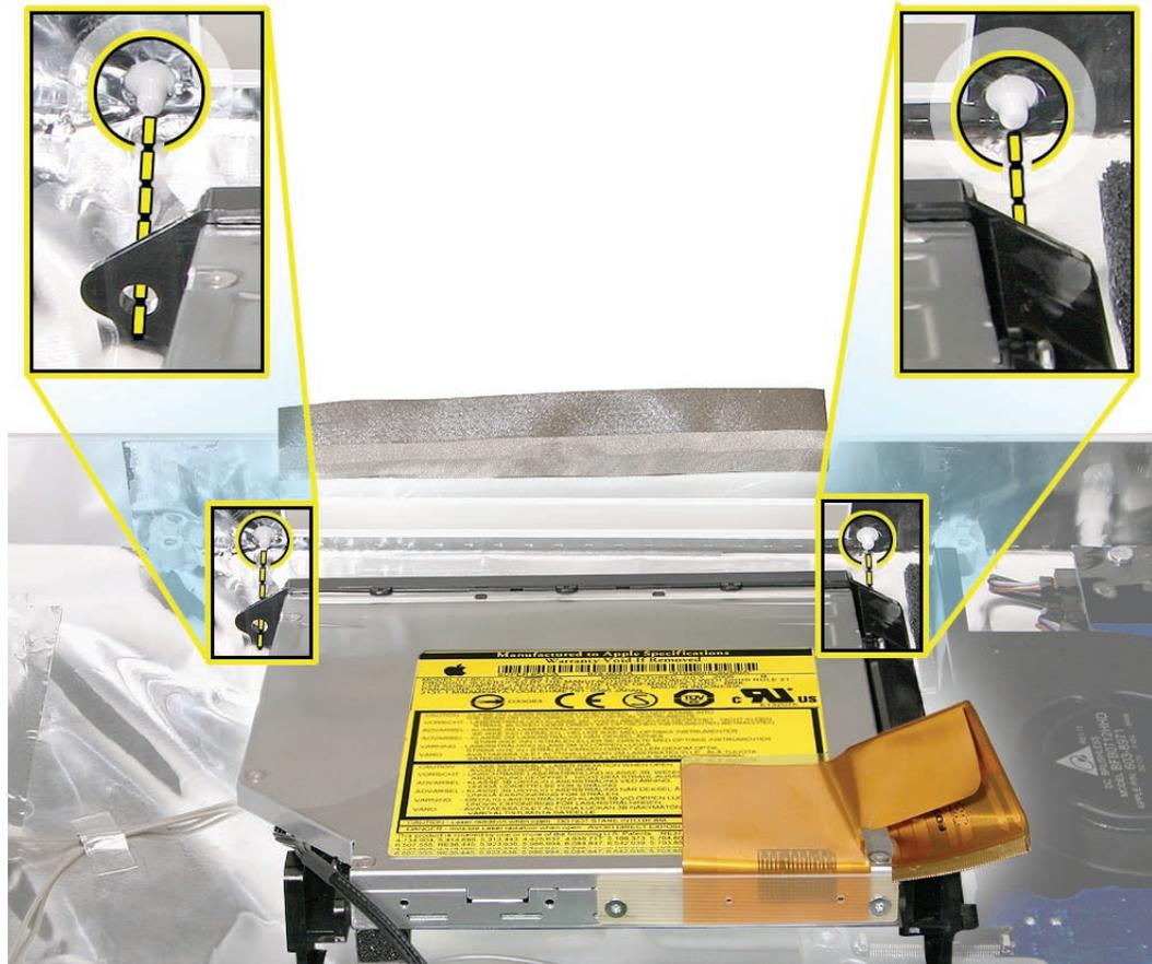
4. Push down on the mounting brackets clips to lock the optical drive securely into place on the chassis.
