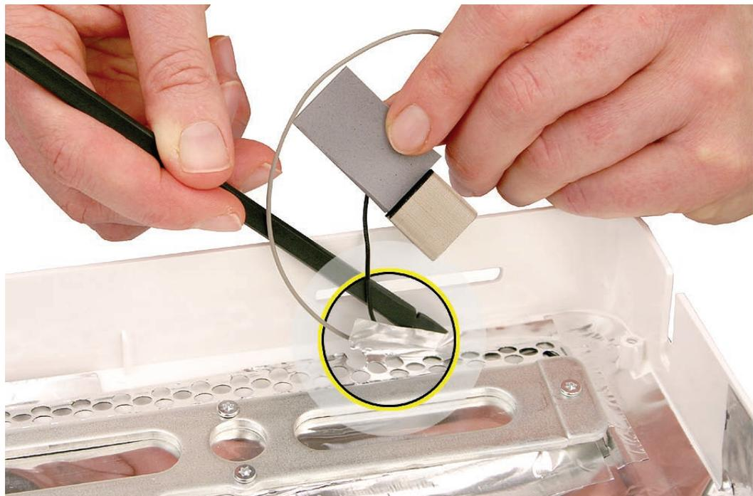
5. Note how the cables are routed at the right corner of the chassis.
