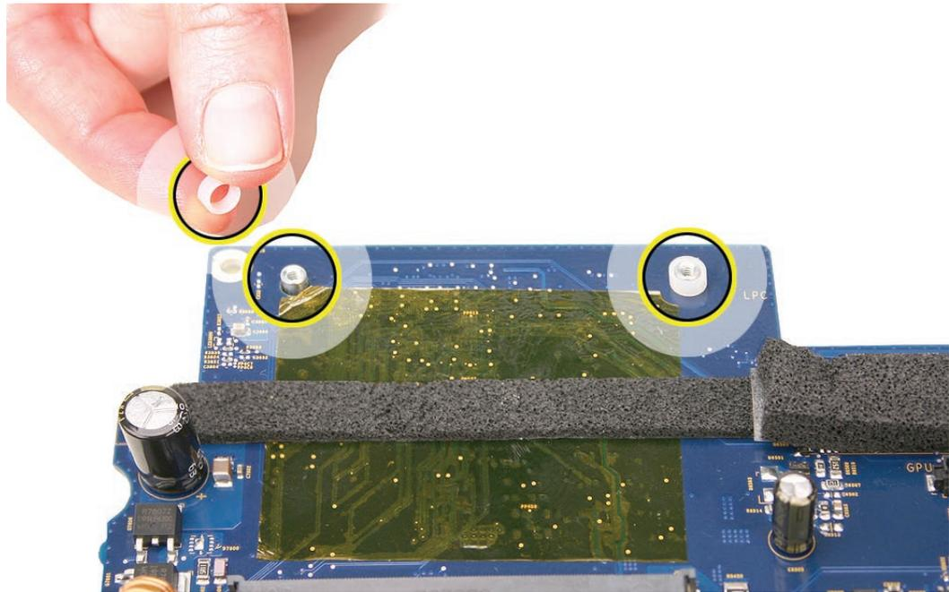
3. Connect the video card to the logic board, and install the three screws.
