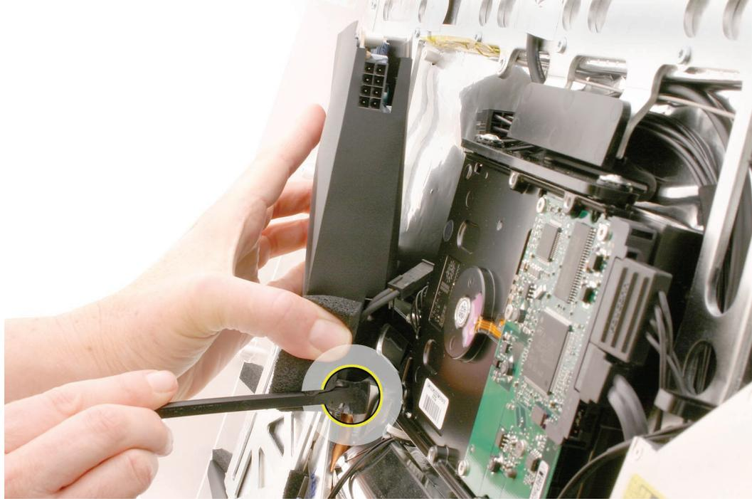
4. Tilt the power supply to disconnect the lower right locking cable from the power supply.
