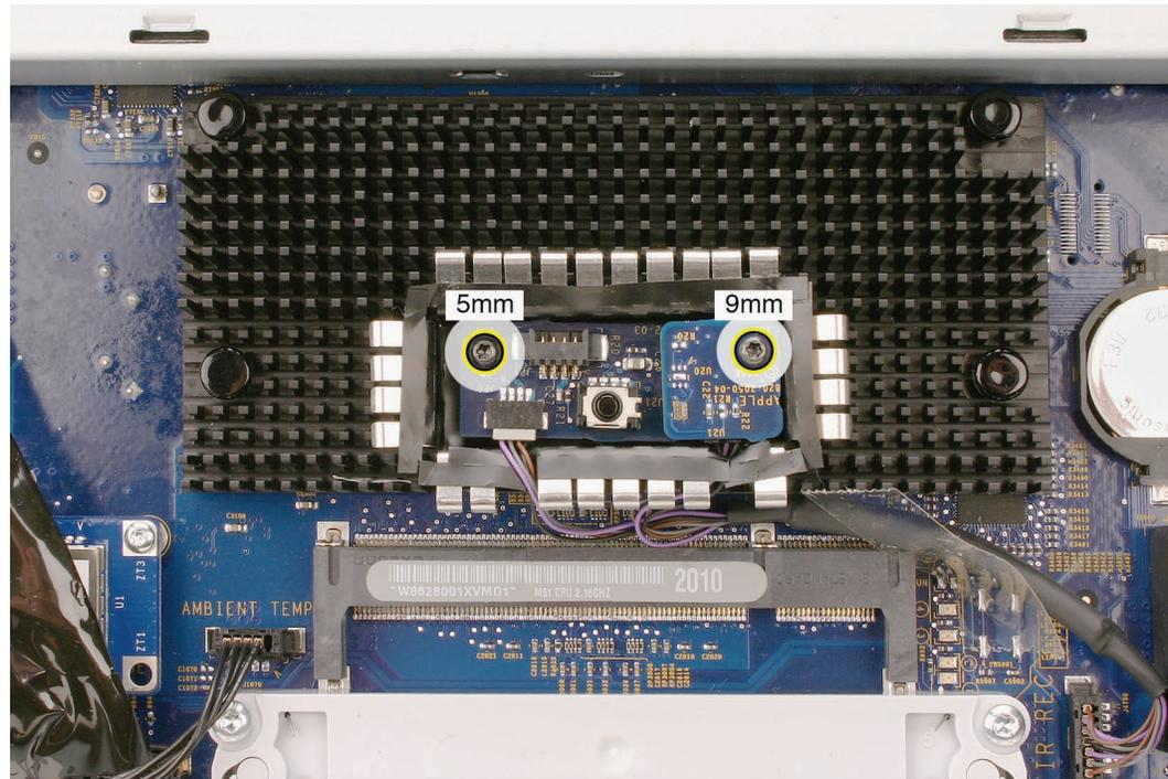
2. Tilt out the IR board, and disconnect the IR/ALS cable from the IR board. Lift the IR board from its IR shield.
