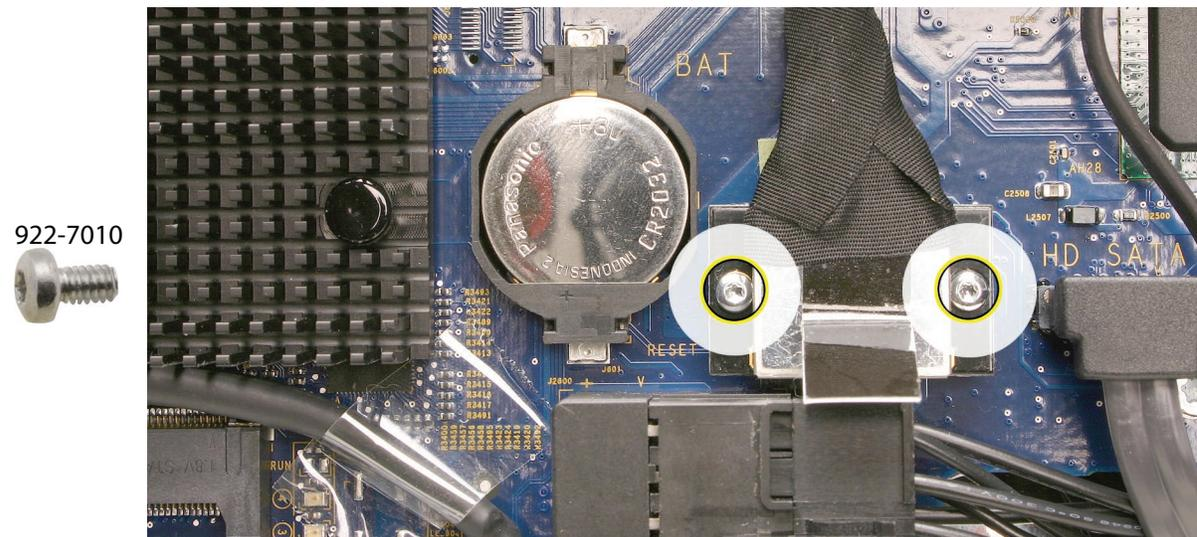
6. Connect the inverter cable to the logic board.
