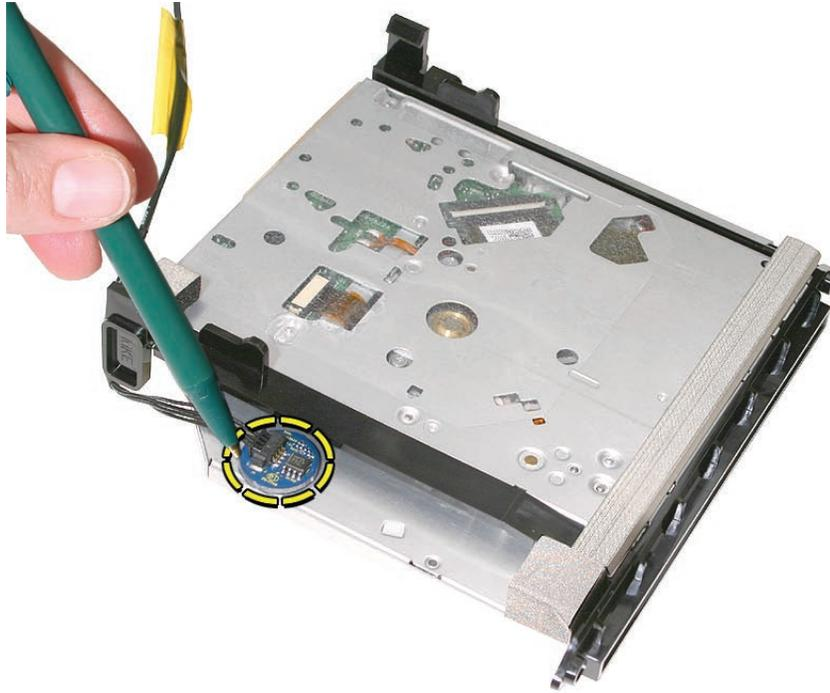
9. Use a black stick to peel up the temperature sensor from the adhesive on the bottom of the drive.
