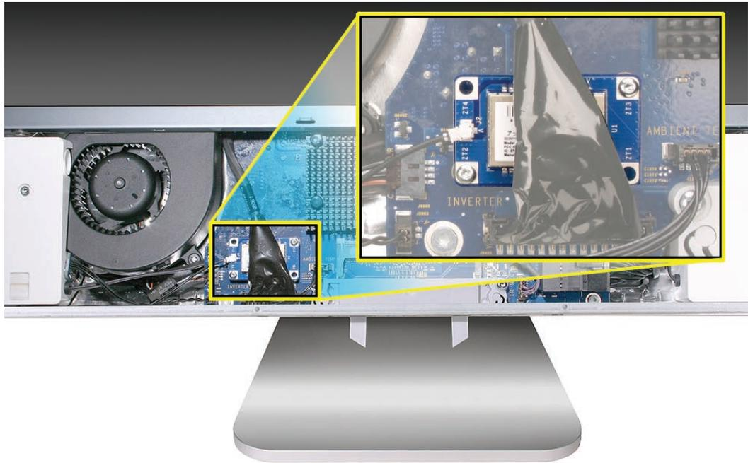
3. Disconnect the Bluetooth antenna from the left side of the card.
