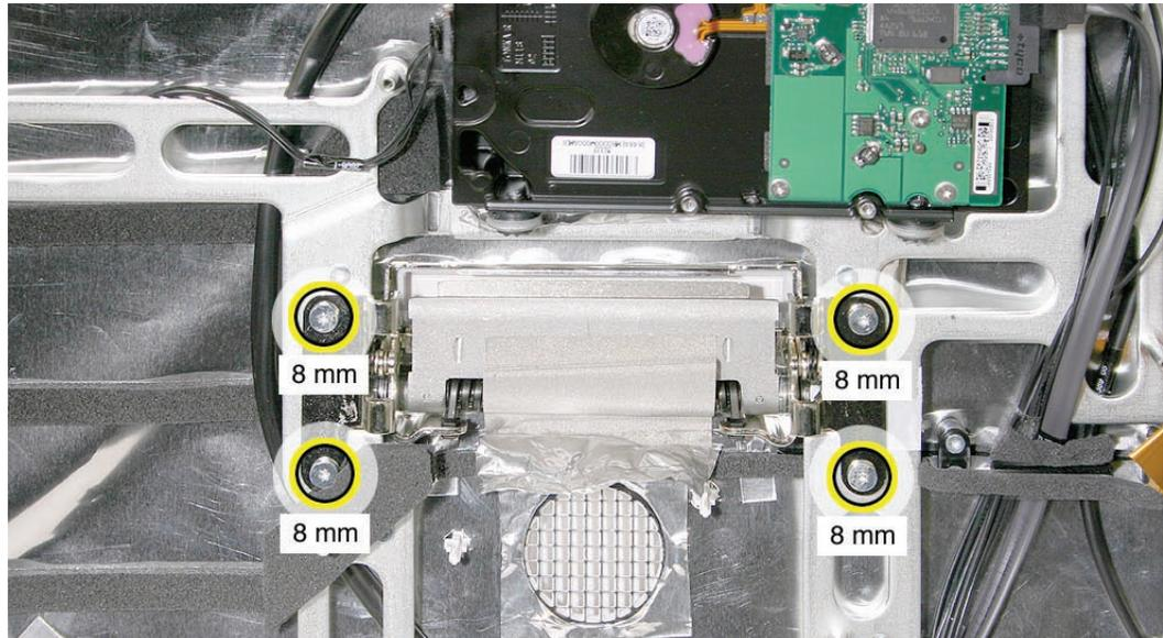
2. Peel back the mesh tape on top of the mechanism.
