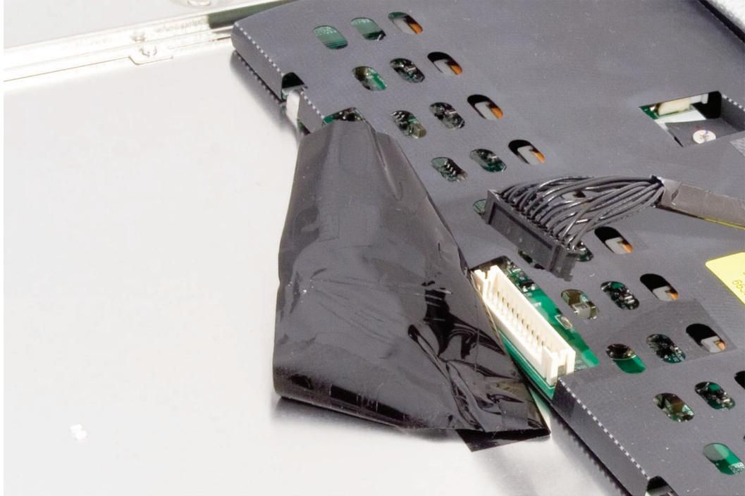
2. With both the LVDS cable and the inverter cable connected to the back of the display panel, install the display panel with eight mounting screws.
