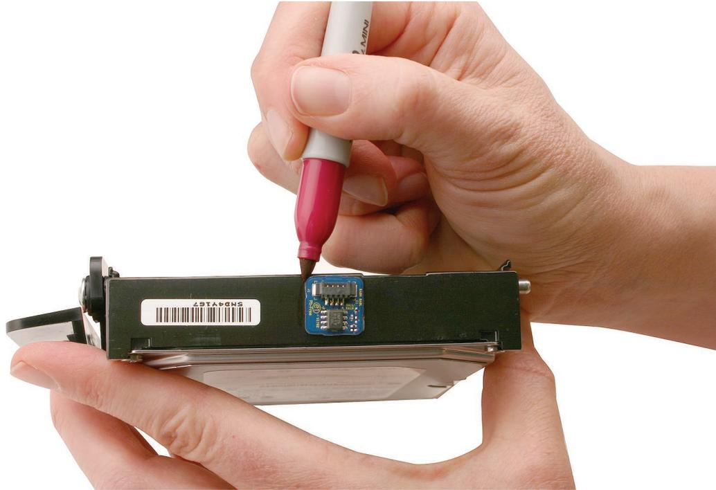
2. Use a black stick to peel up the temperature sensor from the adhesive on the left end of the drive.
