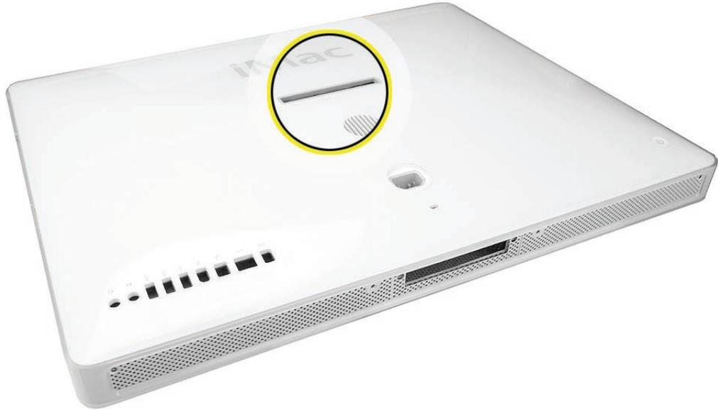
5. Insert the access card into one end of the stand slot and push the latch away from you. (When the latch moves, you feel the moderate resistance of the latch spring.)
