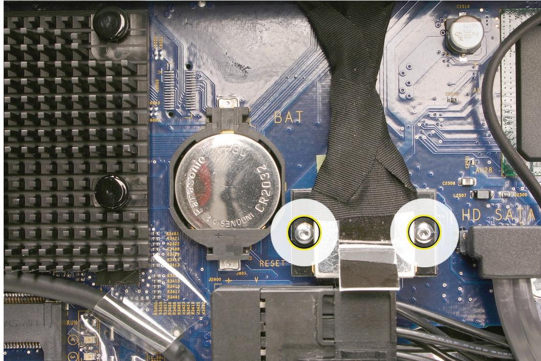
3. Disconnect the LVDS cable and inverter cable from the logic board.
