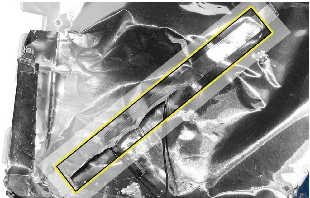
4. Open the “sleeve” of the EMI backing to access the rest of the antenna cable.
