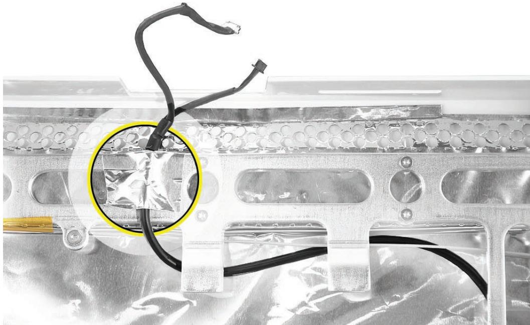
3. Route the rest of the cable out from under the chassis.
