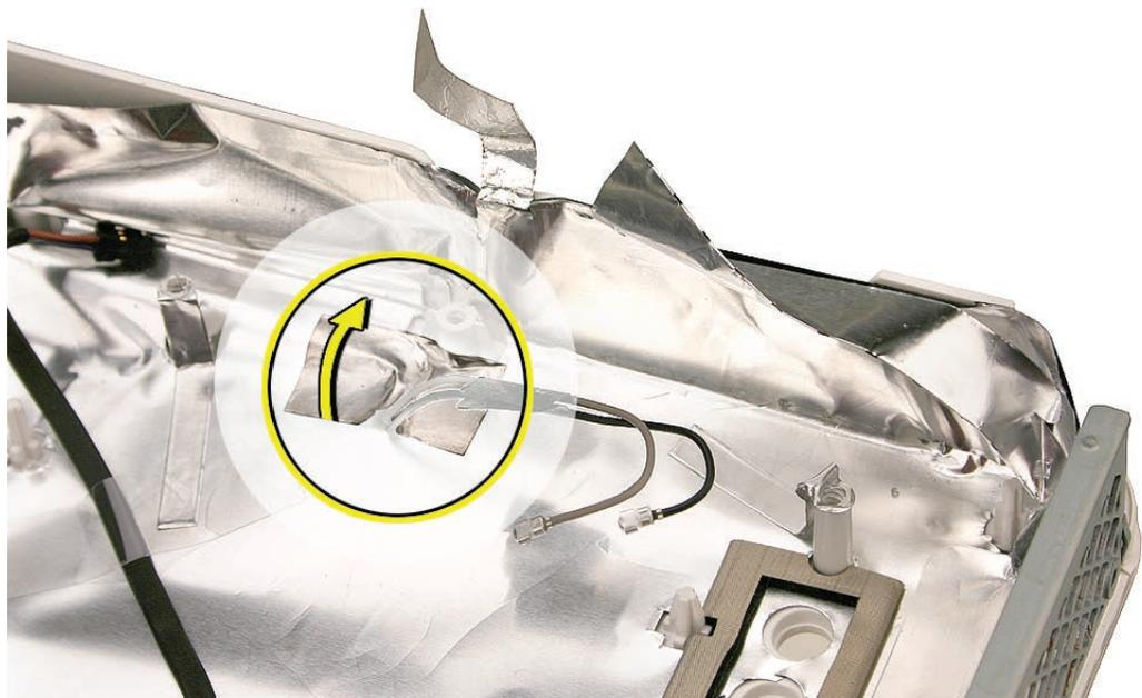
9. At the lower right corner on the underside of the EMI shielding, use a black stick to carefully guide the remaining section of the cables out through the opening in the shielding.
