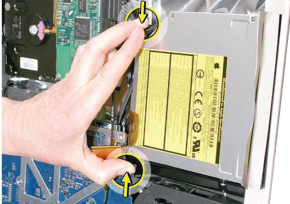
5. Connect the flex cable to the logic board
