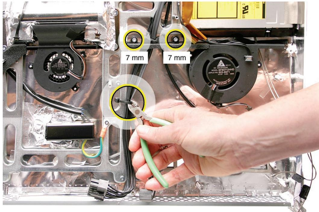
2. Disconnect the hard drive data cable from the hard drive, and route the cable down through the cable channel.
