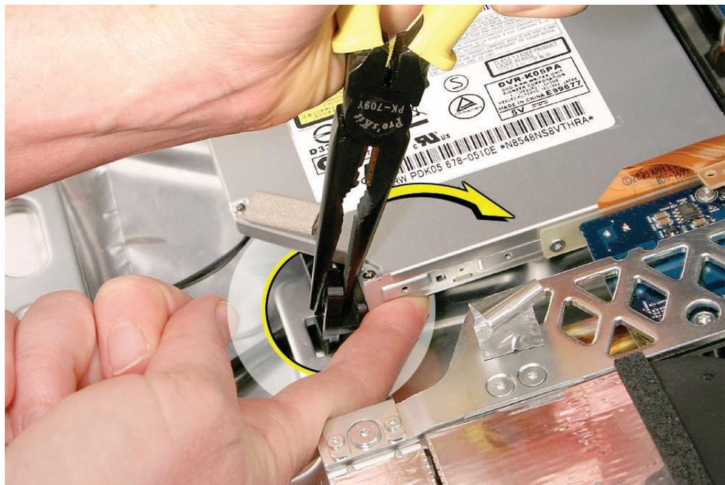
5. Squeeze the clips toward each other to unhook the drive from the chassis.
