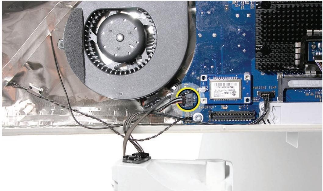
4. Pull out the fan from the guide posts on the rear cover.
