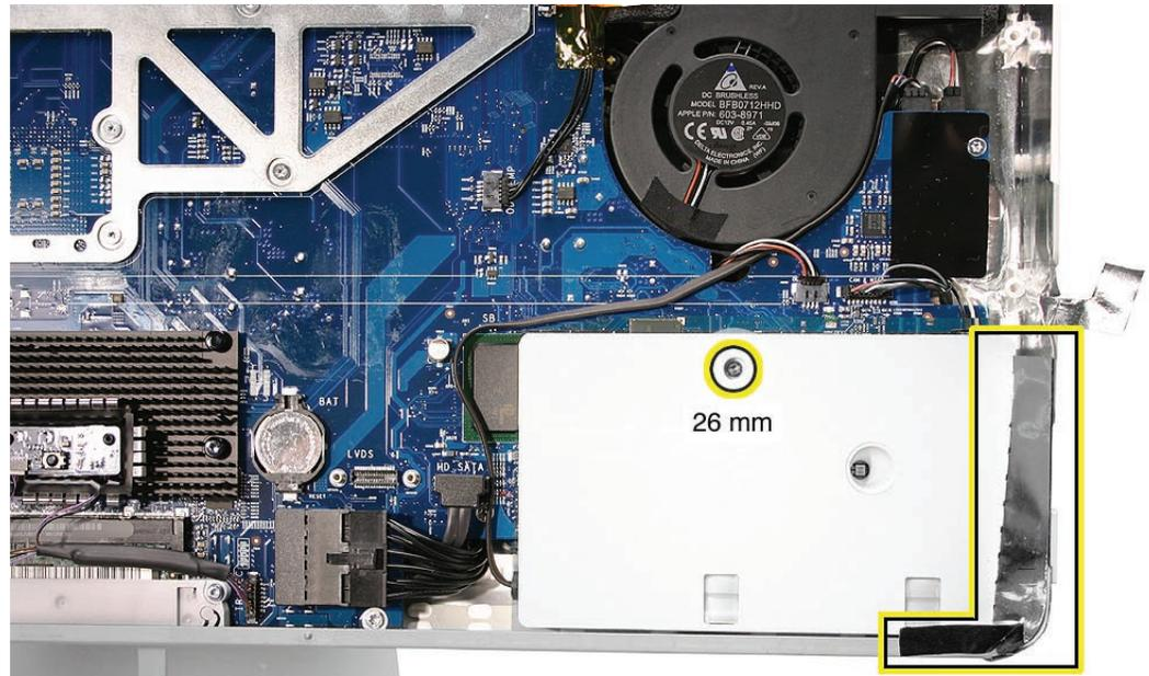
2. Without straining the speaker cable, pull up the speaker body and rest it on the table.
