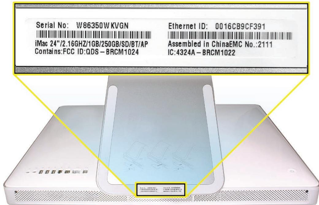
This label also provides the computer configuration and an “EMC” number (EMC No.). The EMC number for the iMac (24-inch) computer is 2111. The EMC number is unique for different iMac models.
