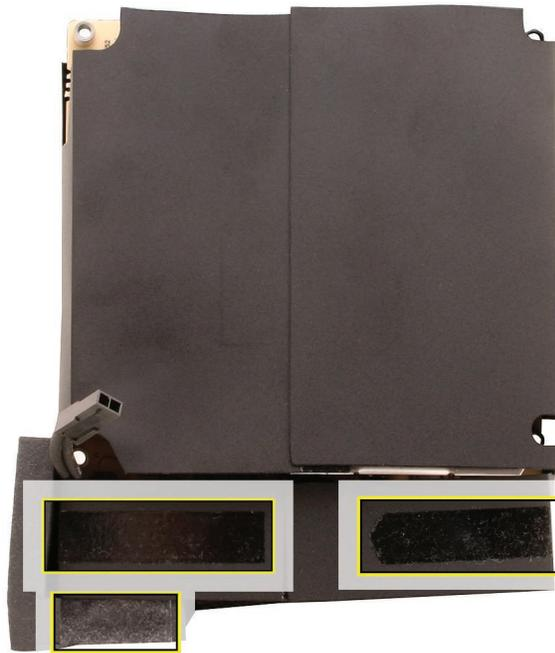
7. Note that a replacement power supply comes with the attached cable, mylar sleeve, foam gaskets, and adhesive strips.
