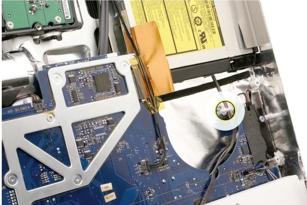
2. Lower the fan onto the guide posts in the rear cover. Connect the fan cable.
