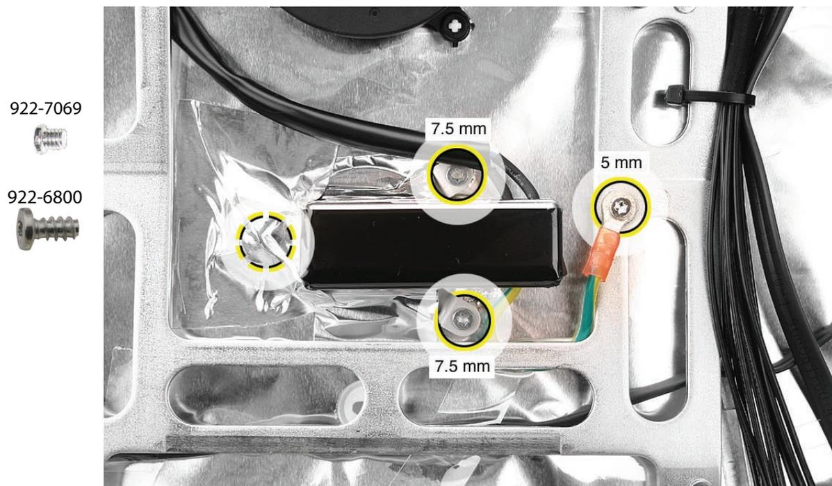
3. Route the cable out from under the chassis, and remove the AC power inlet.
