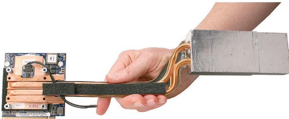
5. Be sure to retain the two plastic spacers on the video card area of the logic board.
