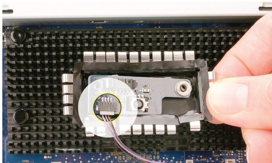
3. Remove the IR board from the IR shield and logic board.
