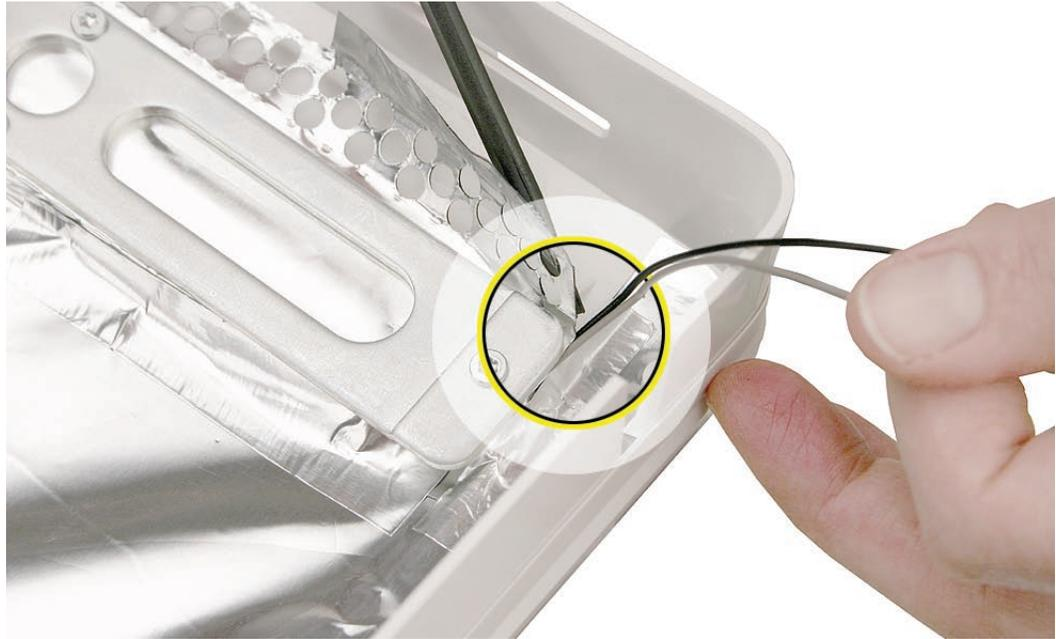
6. Continue to route the antenna cables from underneath the EMI shielding. However, because the shielding runs up the entire right side of the rear housing, you must carefully peel back the right side of the EMI shielding (including the slot-load drive opening).
