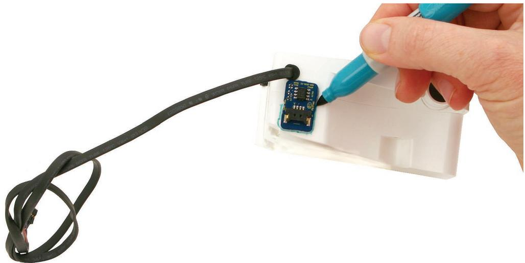
2. Install the sticky side of the sensor on the speaker within the outlined marking.
