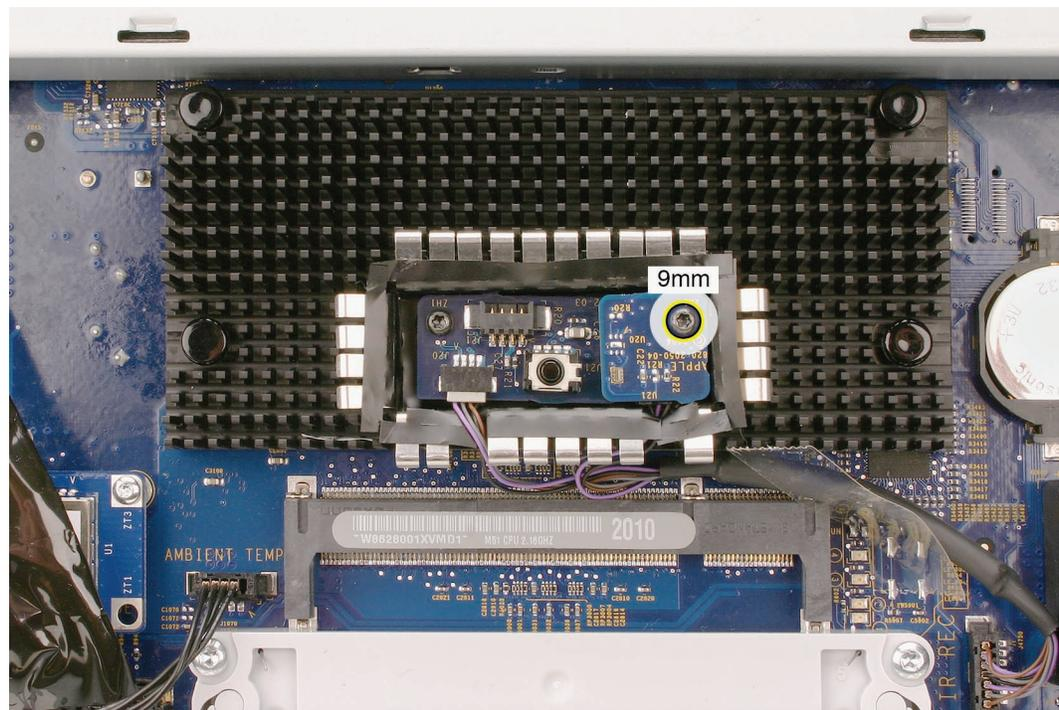
2. Tilt out the ALS board, and disconnect the IR/ALS cable from the board. Lift the ALS board from the IR board and IR shield.
