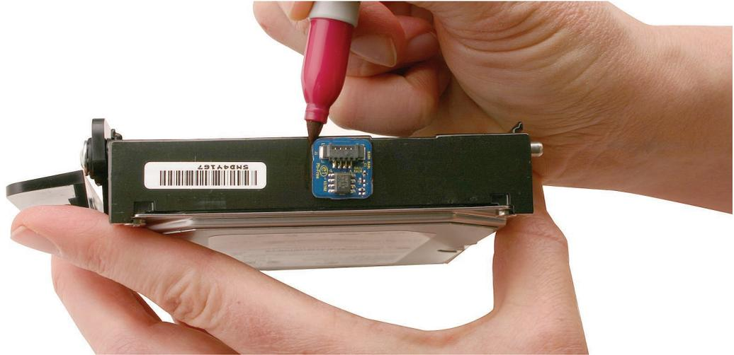
7. Use a black stick to peel up the temperature sensor from the adhesive on the left end of the drive.
