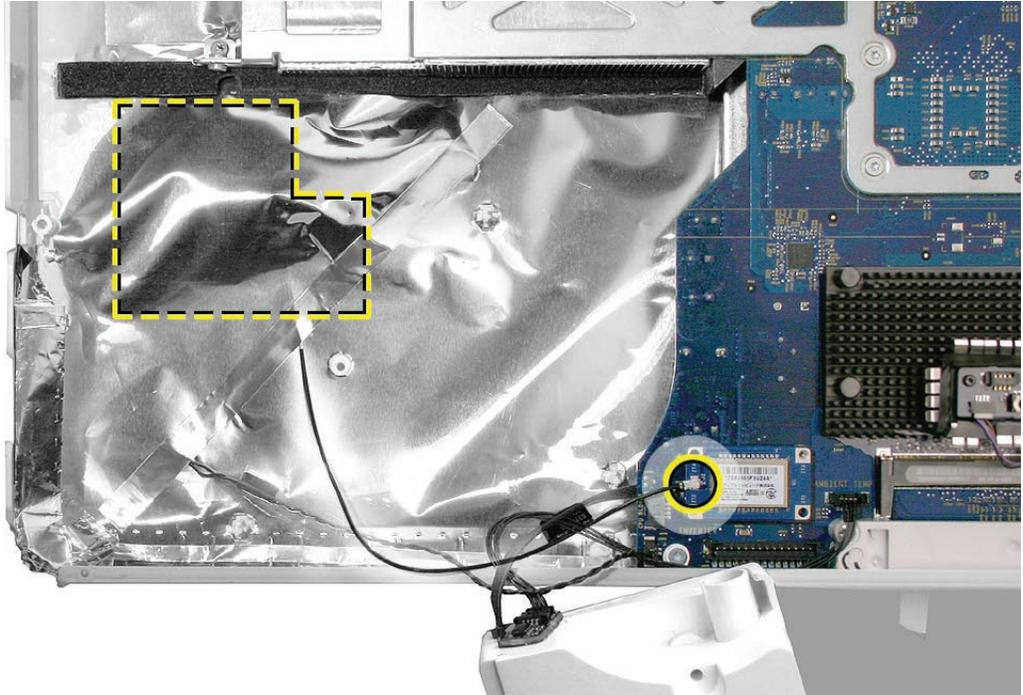
3. Carefully peel back the long strip of EMI tape from the lower left corner of the rear cover, as shown below.
