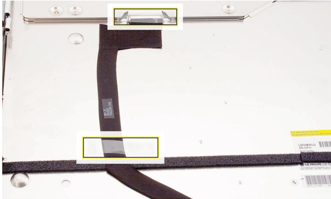
2. Press in on the cable clips and then pull straight down on the cable to disconnect the LVDS connector.
