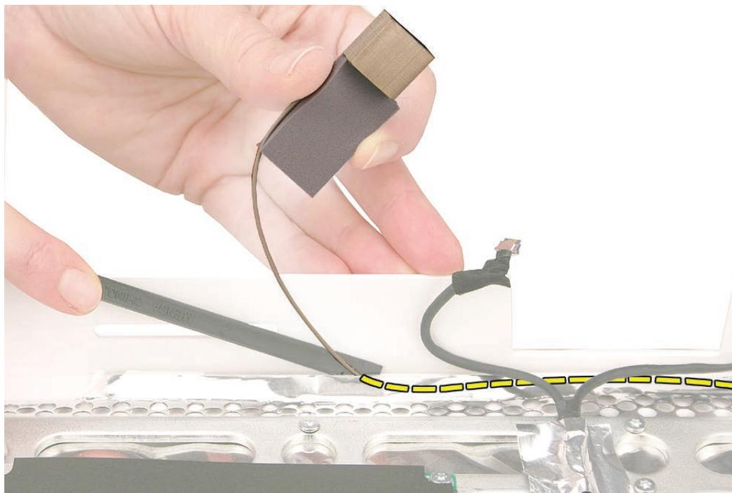
3. At the top of the rear cover, note the location and placement of the right antenna board.
