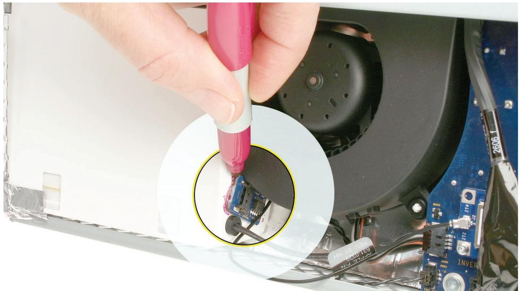
3. Use a black stick to peel up the sensor from the adhesive on the side of the speaker.
