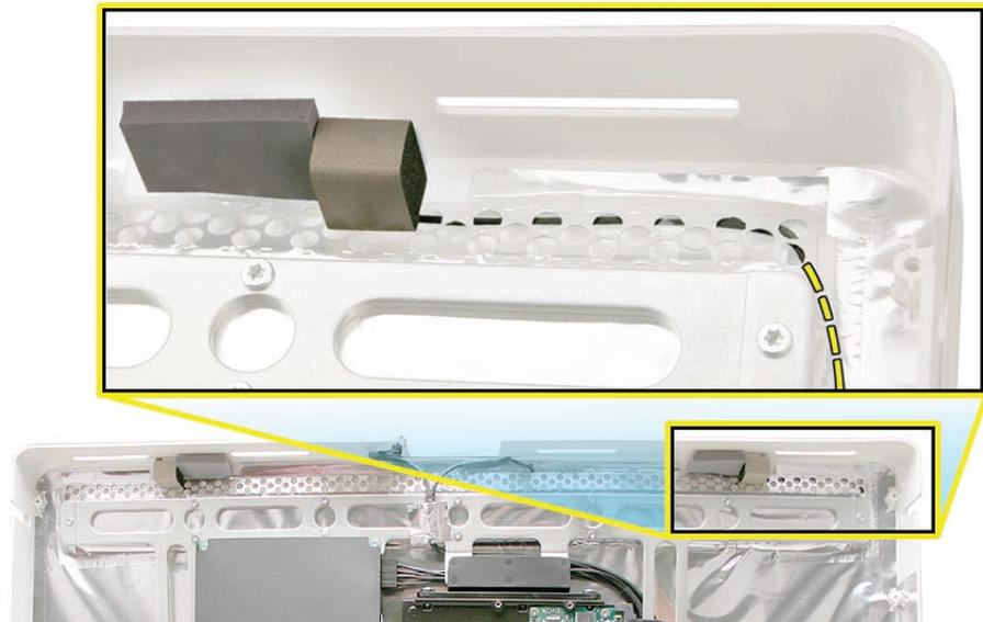
4. At the top right corner of the rear cover, pry up the right antenna board. Carefully pull up both antenna cables from under the edge of the EMI shielding.
