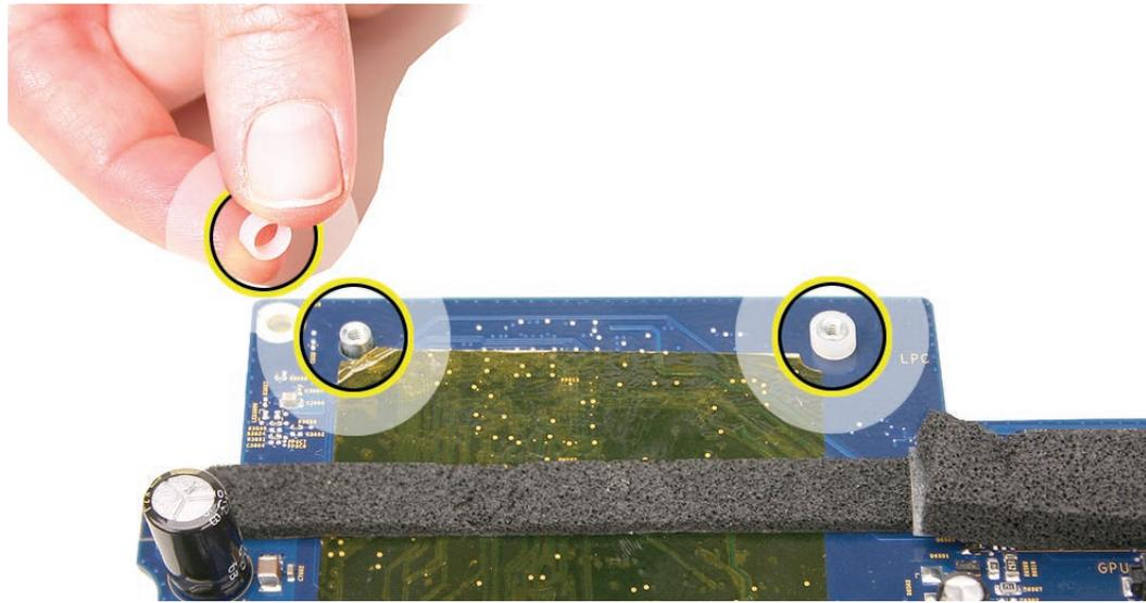
6. Note that a replacement video card includes a temperature sensor and cable. Make sure these are pre-installed on the card before you replace the video card. (The sensor cable runs under the foam strip.)
