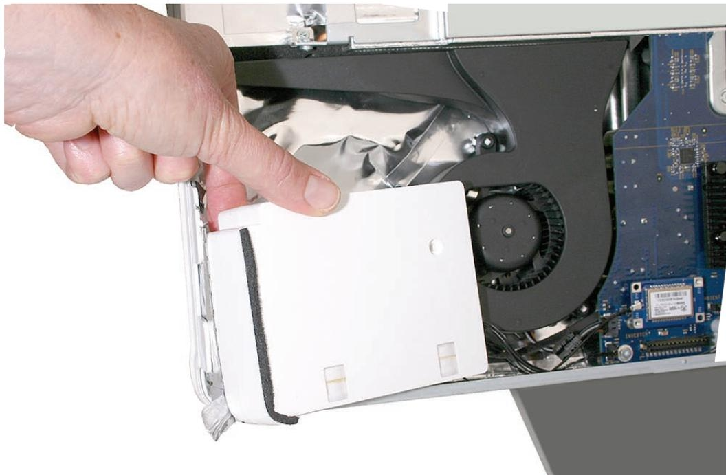
3. Disconnect the fan cable from the lower left corner of the logic board.
