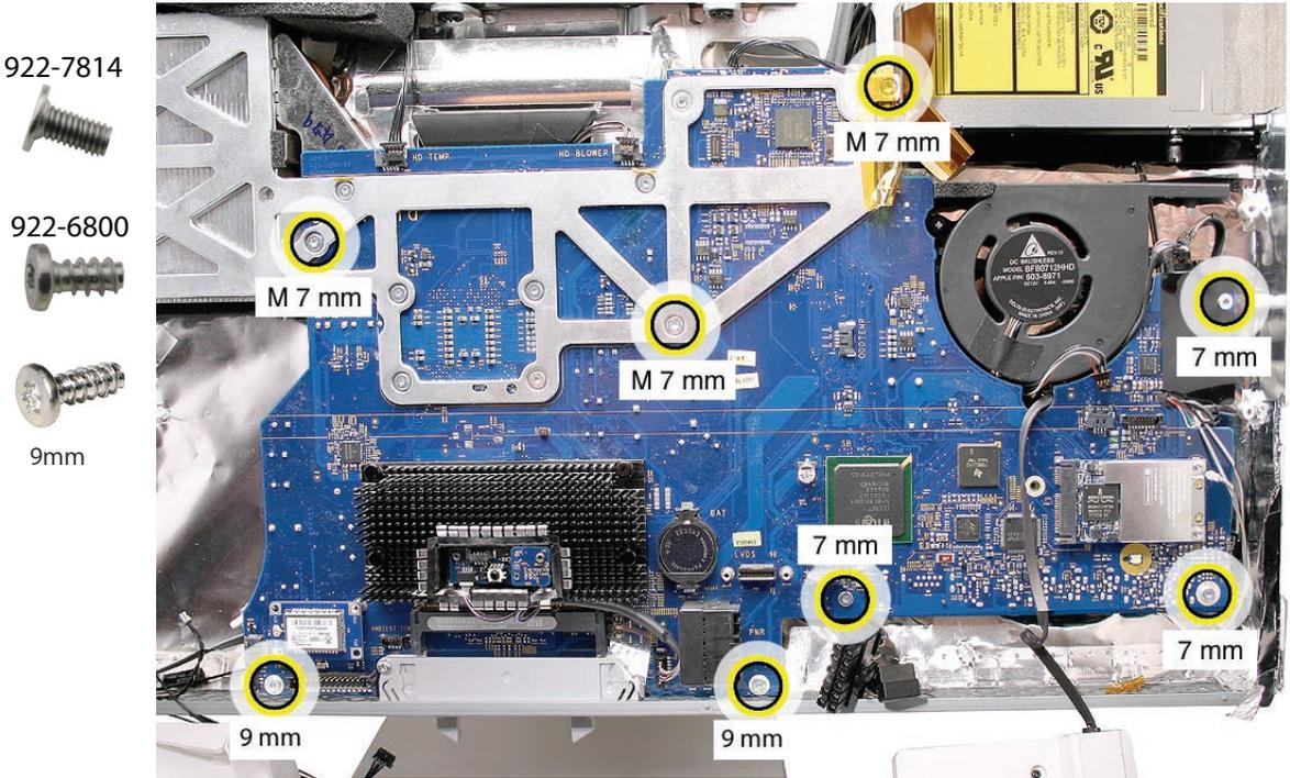
3. Note that the three machine screws on the backer plate have an arrow designation.
