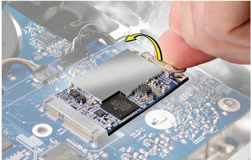
5. Holding the card by the edges, pull the AirPort Extreme card out of the slot, and disconnect the antenna cables.
