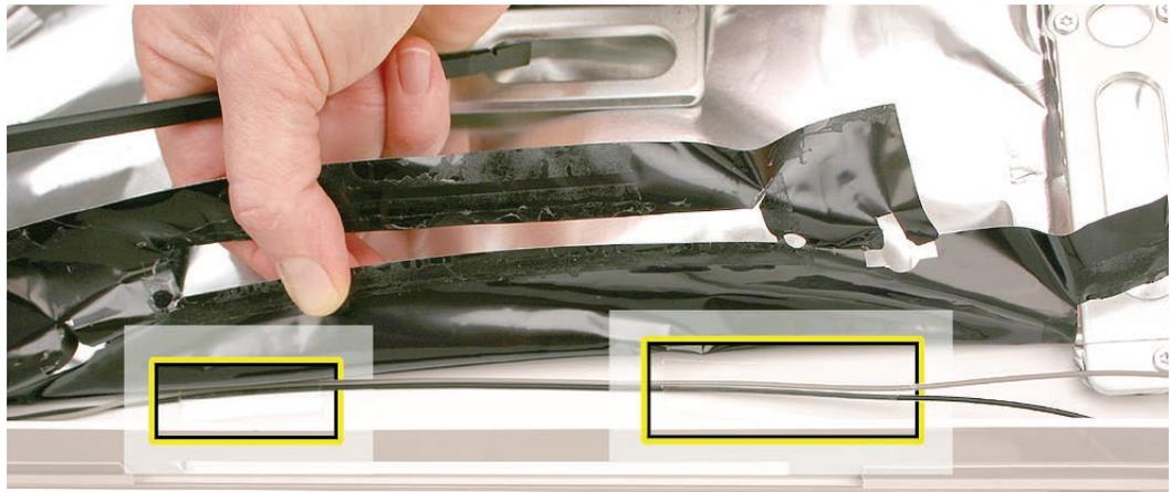
8. Down near the lower right corner where the antenna cables exit the EMI shielding, peel up the single strip of aluminum tape.
