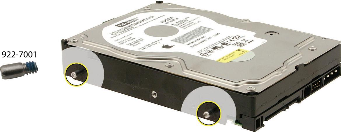
9. At the upper side of the drive, remove the two screws and the plastic clip.
