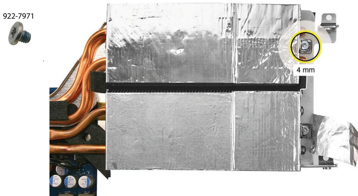
3. Tilt up the video card with attached heatsink, and disconnect it from the card connector on the logic board.
