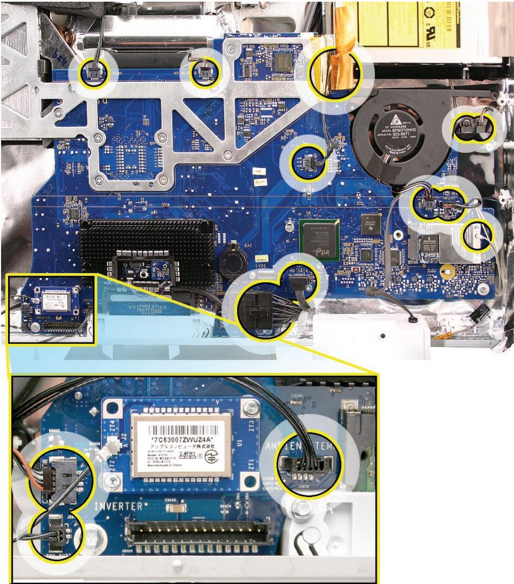
13. Replace the three machine screws first; then replace the five self-tapping screws.
