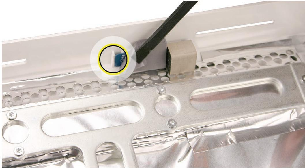
5. When securing the left antenna board, make sure the edge of the board fits directly beside the vertical ridge on the rear cover.
