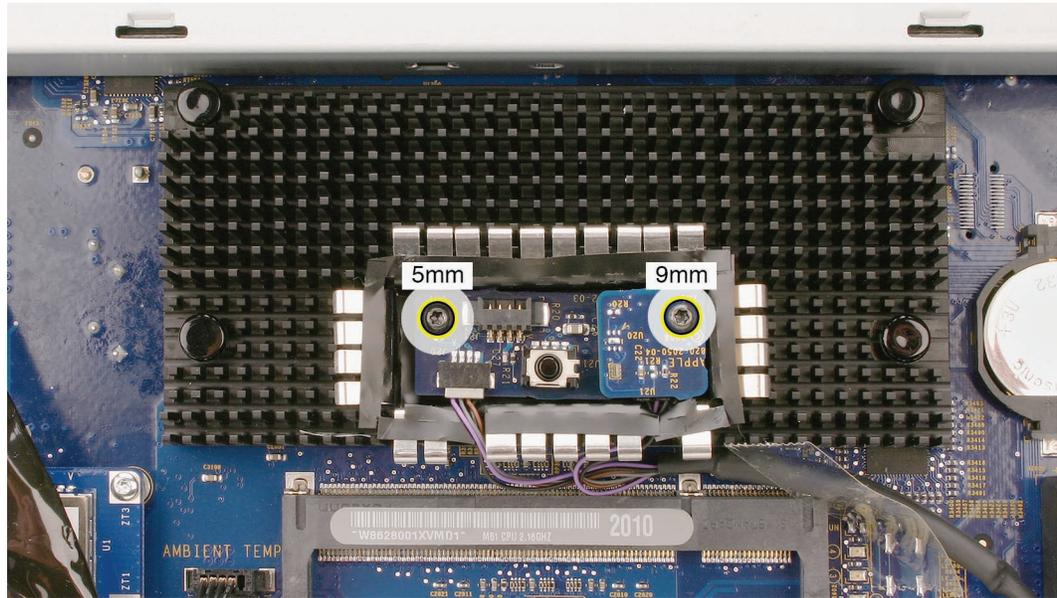
2. Lift out the ALS board and disconnect the cable from the ALS board.
