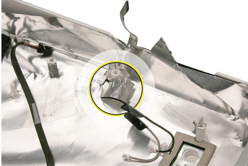
3. Follow the removal instructions in reverse to route the antenna cables up the right side of the rear cover and underneath the EMI shielding.
