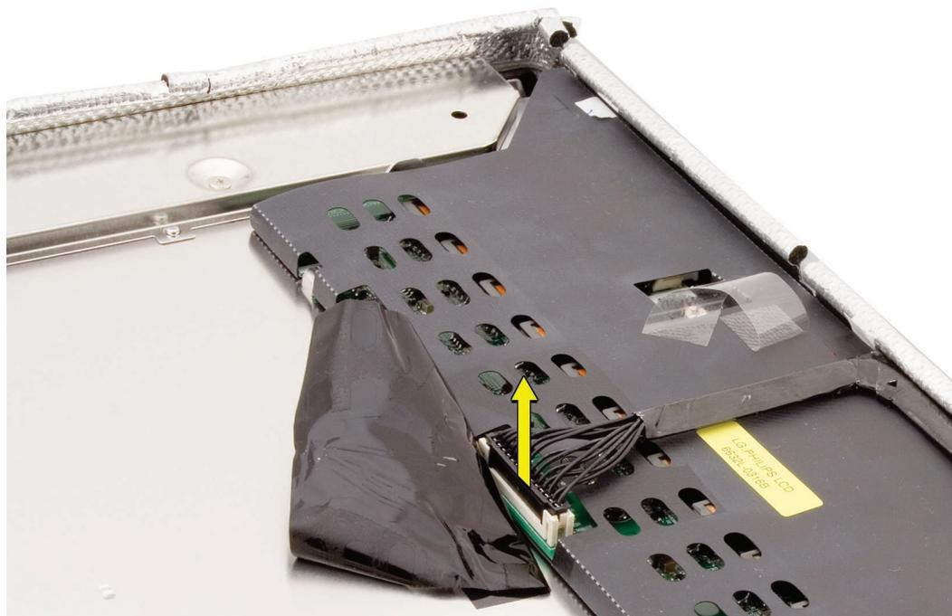
3. Lift the inverter cable from the display panel.
