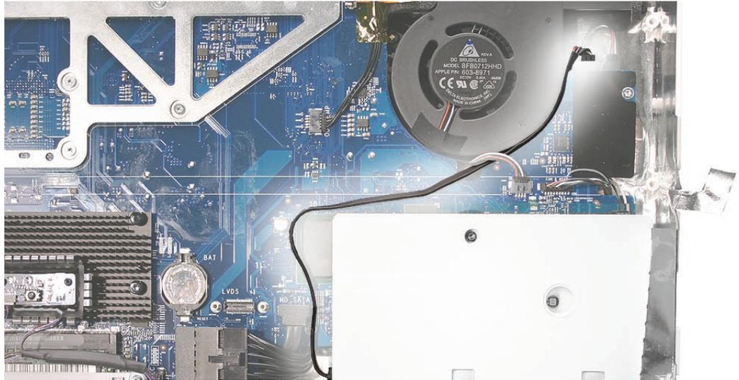
2. Peel up the EMI tape at the lower right corner of the speaker, and remove the 26-mm long screw from the right speaker.
