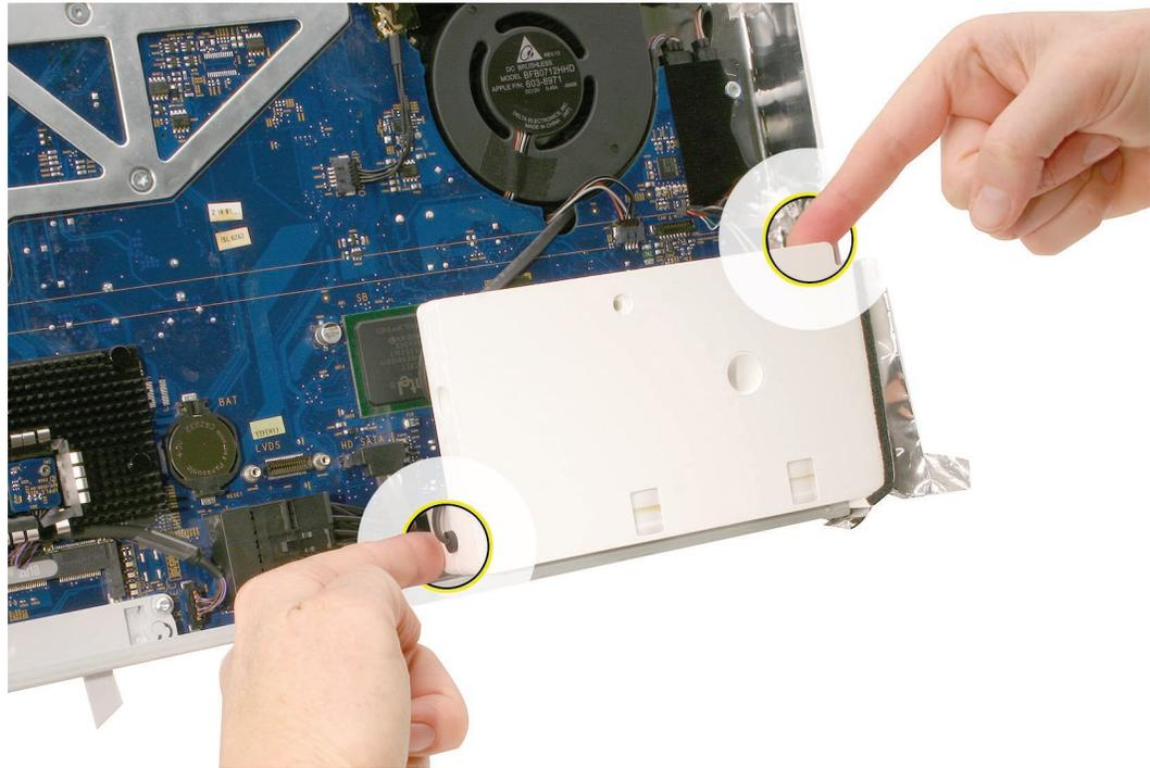
4. Rest the speaker on the table as you disconnect the right speaker cable from the top right corner of the logic board.
