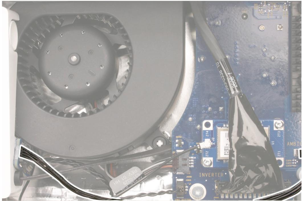
2. Check the position of the ambient temperature sensor on the left speaker. Use a permanent ink marker to draw an outline of the sensor.
