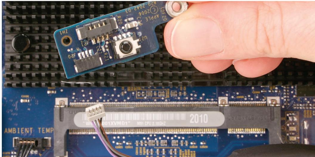
4. Peel up the strip of tape that secures the cable to the logic board, and disconnect the other end of the cable from the logic board.
