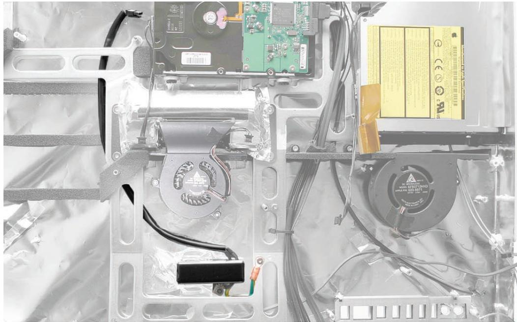
2. Using a torx T10 screwdriver, remove the three 7.5-mm long self-tapping screws from the power inlet and the 5-mm long machine screw from the ground cable. Remove the EMI tape on the metal case.
