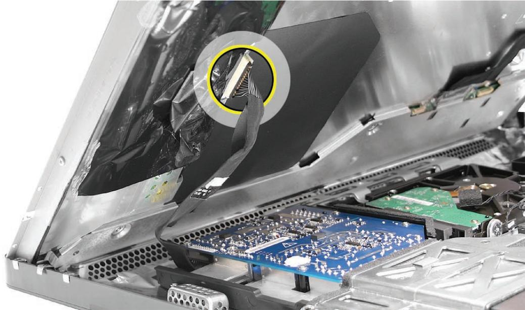
3. Connect the other end of the inverter cable to the power supply.
