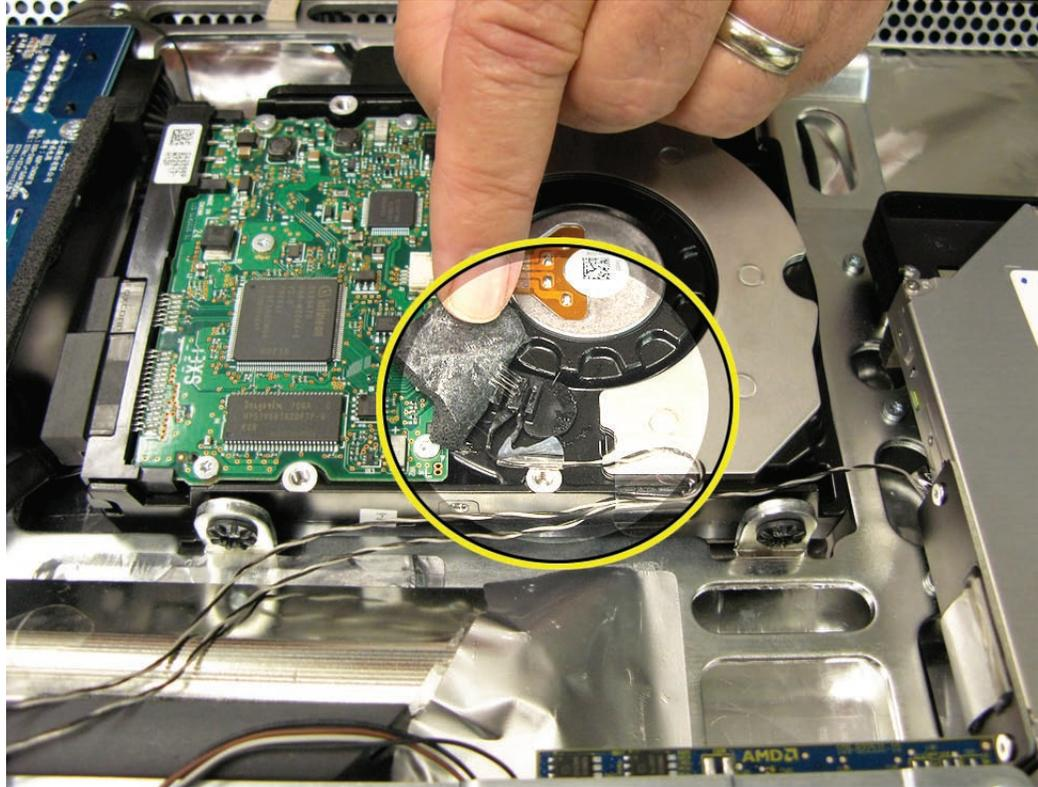
6. Connect the other end of the temperature sensor cable to the logic board.
