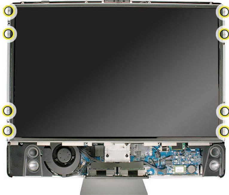
5. Grasp the LCD panel at the bottom edge, and tilt up the panel. Peel back the black tape covering the inverter cable connector on the back of the LCD panel. Pull the connector straight out, toward the power supply. If you are replacing the cable, disconnect the other end from the power supply. Lift the LCD panel off the rear housing.
