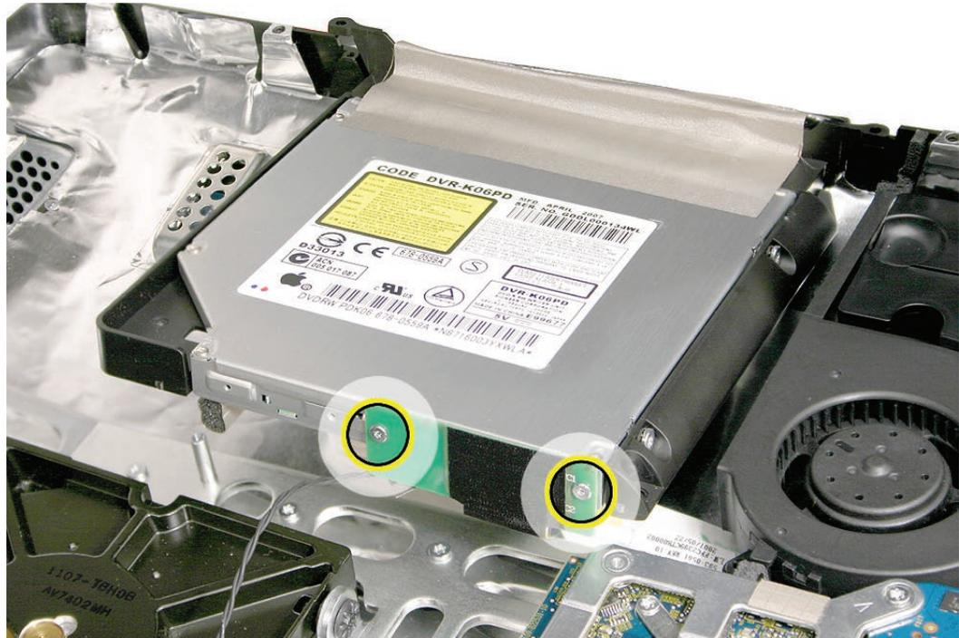
4. Disconnect the temperature sensor cable from its connector on the logic board. On the bottom of the optical drive, peel back the foam gasket (not shown) and disconnect the sensor from the sensor clip. **Replacement Note:** Install a new foam gasket when replacing the optical drive. A replacement foam gasket is included with all optical and hard drives.
