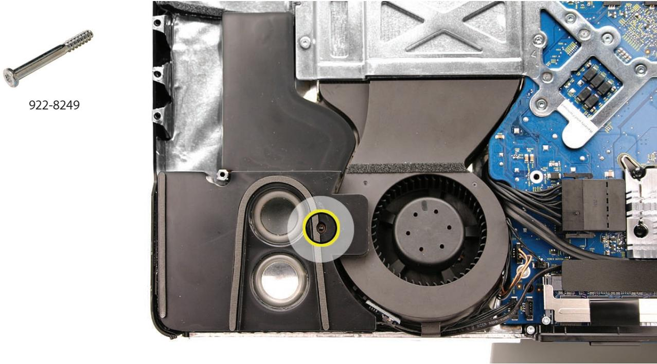
2. Route the speaker cable under the cable clip on the CPU fan and under the long cable guide above the memory slots. Connect the speaker cable to the audio board on the right side.
