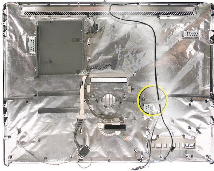
4. Remove any tape securing the camera cable to the rear housing. Lift the camera cable from the rear housing.
