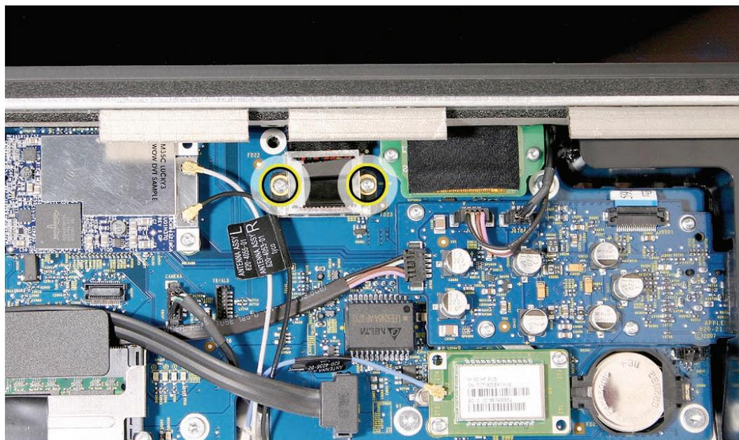
7. Connect the display temp sensor cable to the left side of the logic board.
