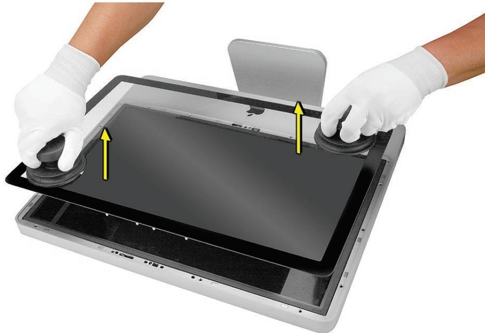
6. Set the glass down on the microfoam bag or clean lint-free surface and remove the suction cups. Squeeze the base of each suction cup to release them from the glass panel.
