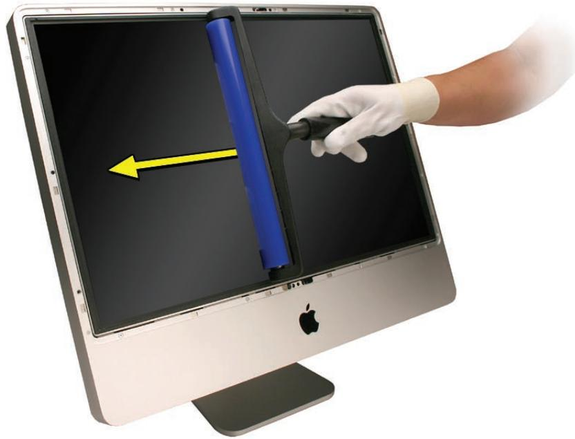
3. Remove the new glass panel from the service packaging. **Note:** The new panels have a removable film protecting the glass on both sides.
