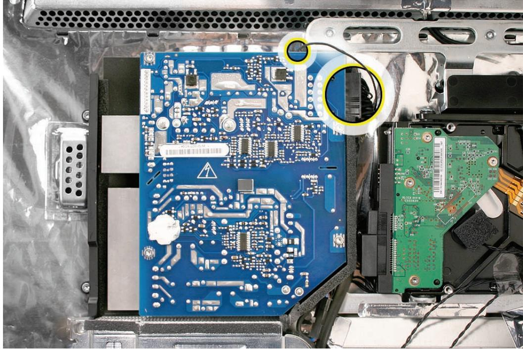
4. This shows a close up of the two-pin ground cable connector on the underside of the power supply.
