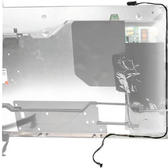
3. On the top right corner of the panel, peel back the mylar tape and foam gasket covering the temp sensor. Disconnect the display temp sensor cable from the sensor. **Note:** Use a black stick to pry the sensor from the top of panel.
