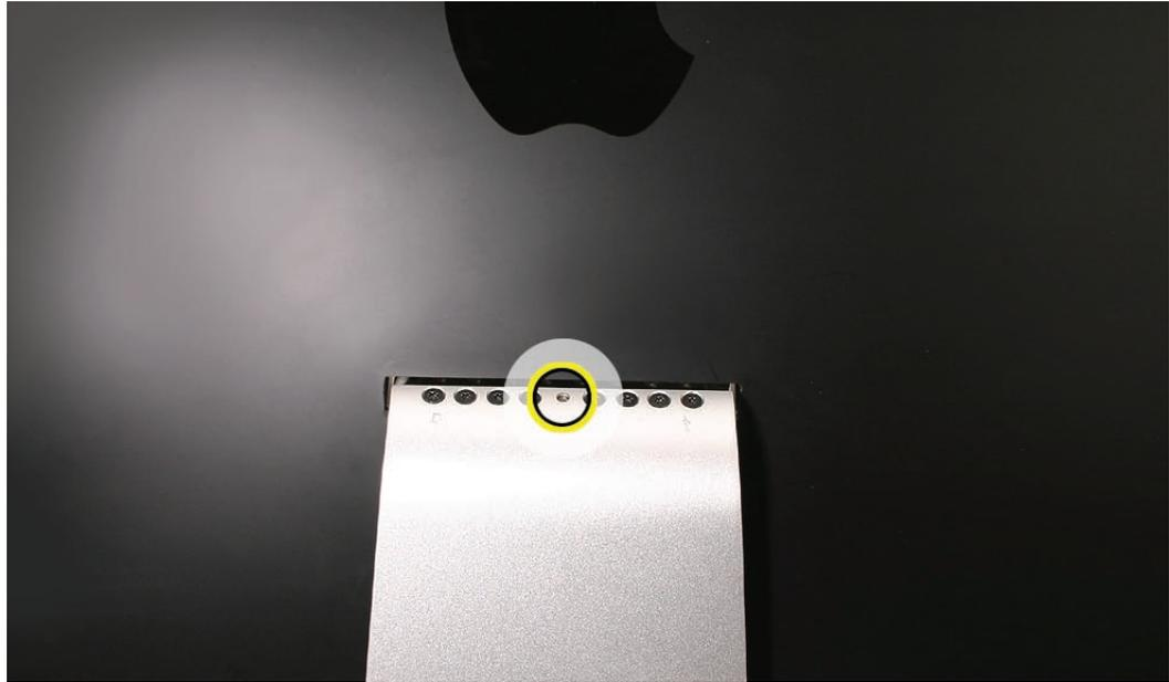
2. Position the stand on the clutch mechanism. Install the eight mounting screws.
