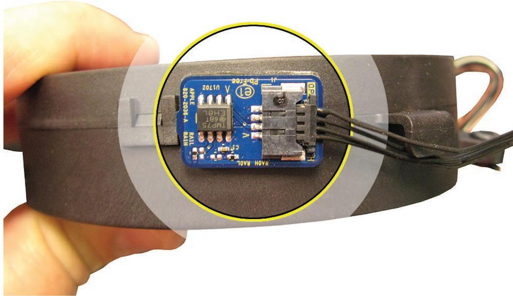
2. Lower the fan into the rear housing. Press the foam gasket into place across the top of the fan.
