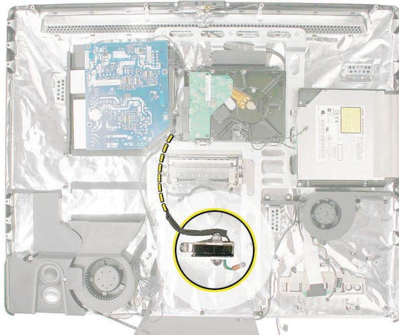
2. Using a torx T10 screwdriver, remove the three 7-5-mm long self-tapping screws from the power inlet and the 5-mm long machine screw from the ground cable. Remove any EMI tape on the metal case.
