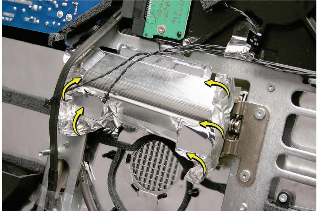
2. Lift the cover off of the clutch mechanism.
