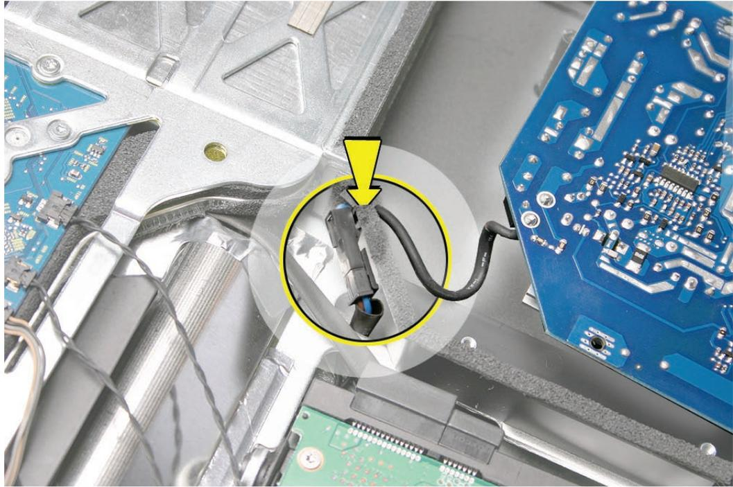
4. Connect the DC power cable and the ground cable to the underside of the power supply.
