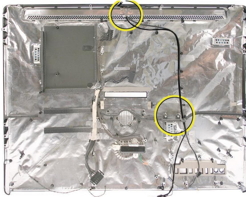
2. Tape the camera cable to the rear housing. Replace the piece of EMI tape at the top, covering the exposed piece of cable.
