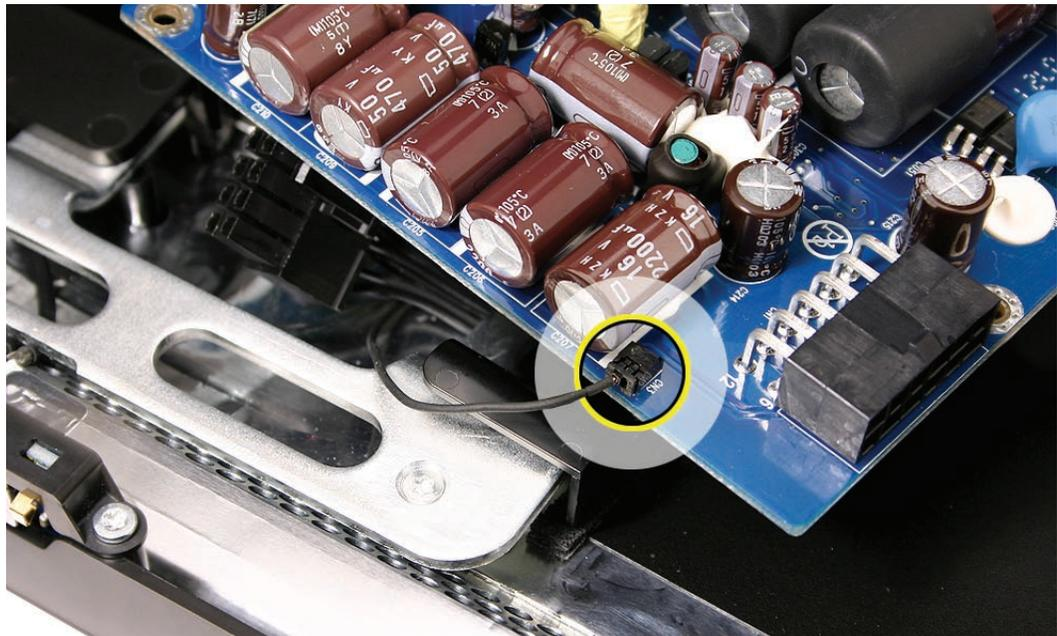
5. Disconnect the AC power inlet cable from the power supply. The cable is tucked neatly between the right pressure wall (black piece of molded plastic along the right side of the power supply) and the top of the logic board.
