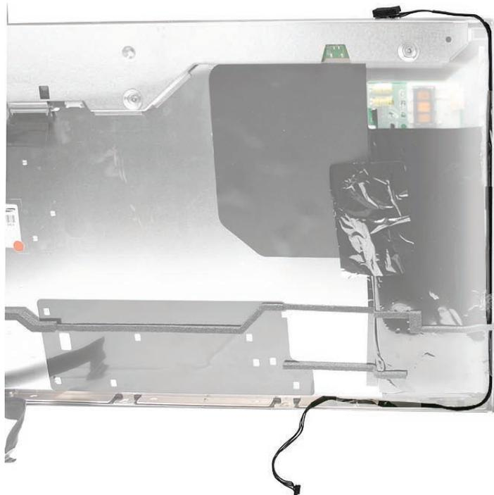
3. Connect the inverter cable to the inverter board on the rear of the display panel. Replace the black mylar tape over the inverter cable connector.
