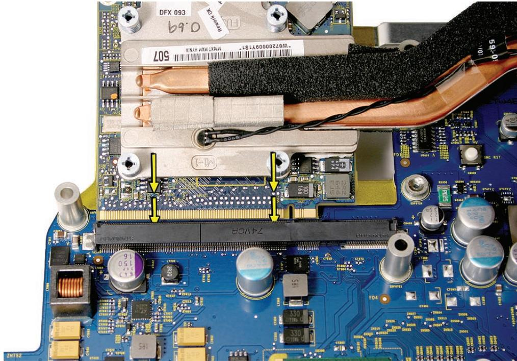
2. Install the three screws and connect the sensor cable to the logic board. **Replacement Note:** The shorter screw attaches at the far right end of the video card heatsink.
