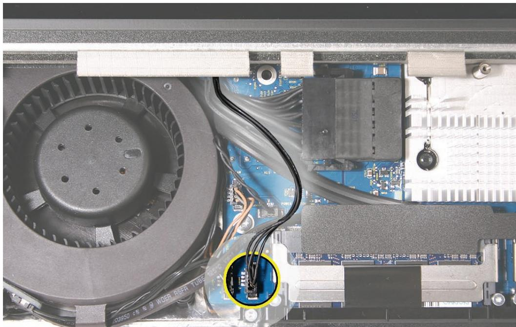
6. Connect the LVDS cable to the logic board. Replace the two T6 screws.
