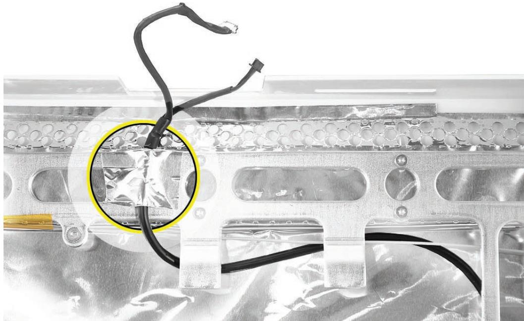
3. Near the middle of the rear housing, remove the two T8 screws on the cable guide
