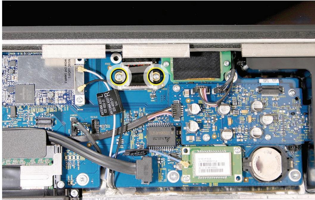
3. Disconnect the display sensor cable from the left side of the logic board.
