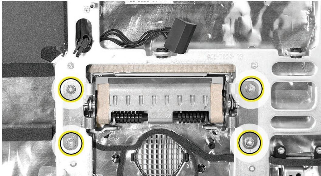
2. If necessary, peel back the mesh EMI tape on the mechanism.
