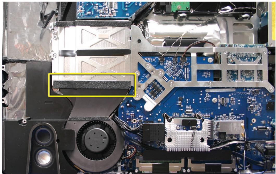
3. Connect the sensor cable and the fan cable to the logic board.
