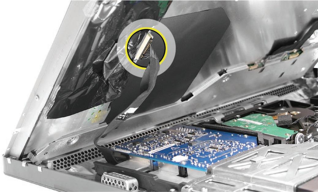
2. If you are replacing the inverter cable, disconnect the other end of the cable from the power supply.
