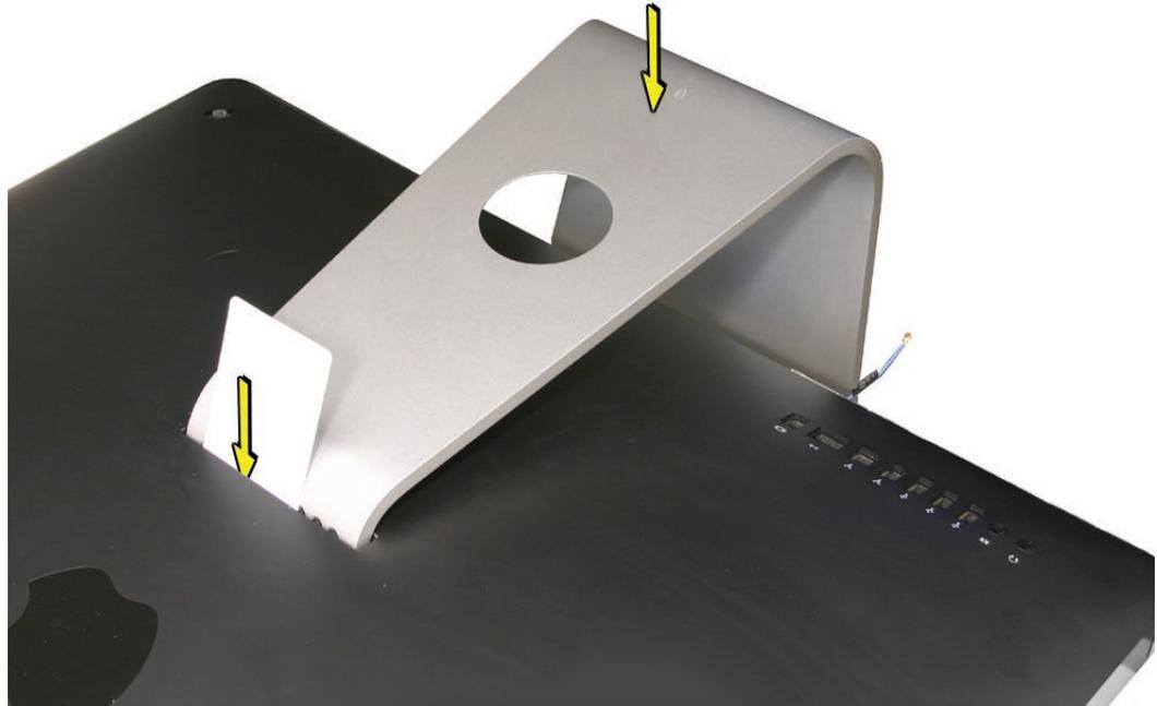
2. Insert the card as far as it will go, and press the stand down until you hear a click—the audible cue that tells you that the stand is locked into place.
