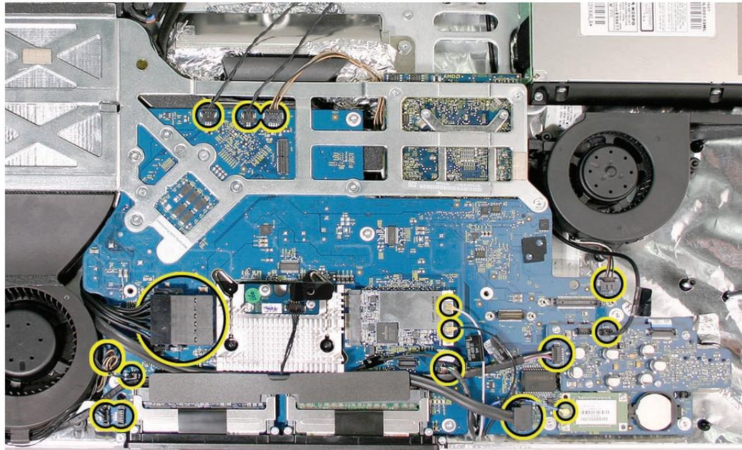
3. Remove the thirteen screws from the logic board. Note that the machine screw location has an arrow designation stamped onto the metal backer plate.
