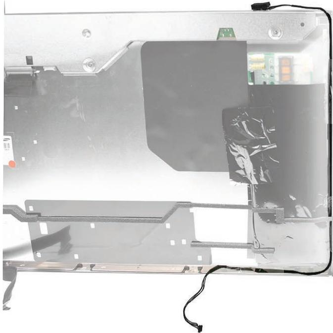
2. Make sure the LCD temp sensor cable is fully inserted into the connector on the bottom left corner of the logic board.
