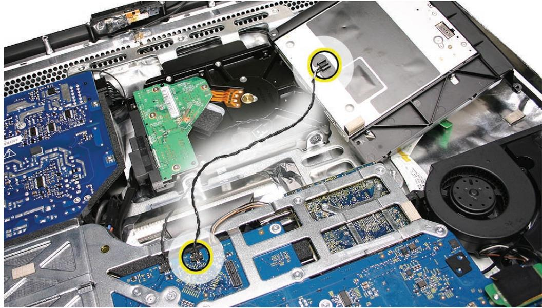
2. Replace the T6 screws on the optical flexible cable.
