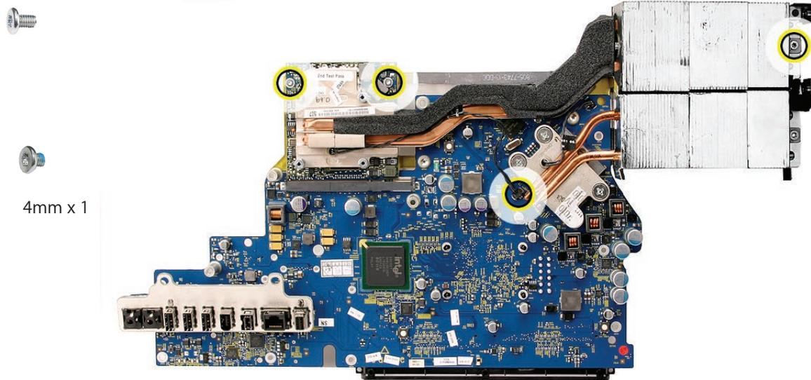
2. Tilt up the video card with attached heatsink, and disconnect it from the card connector on the logic board (as shown with the iMac (24-inch) video card.)
