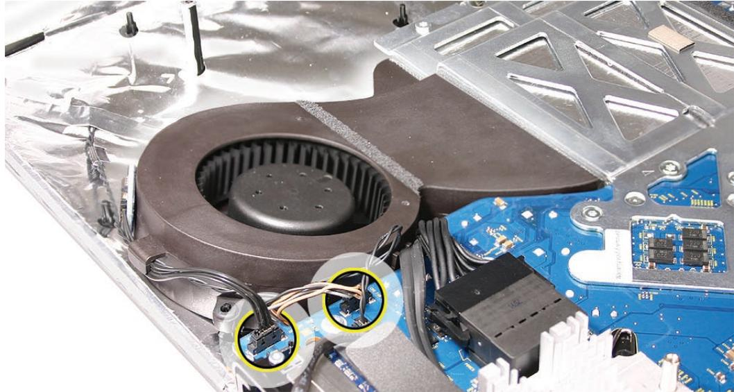
2. Lift the CPU fan from the system. Disconnect the ambient temperature sensor cable from the sensor.
