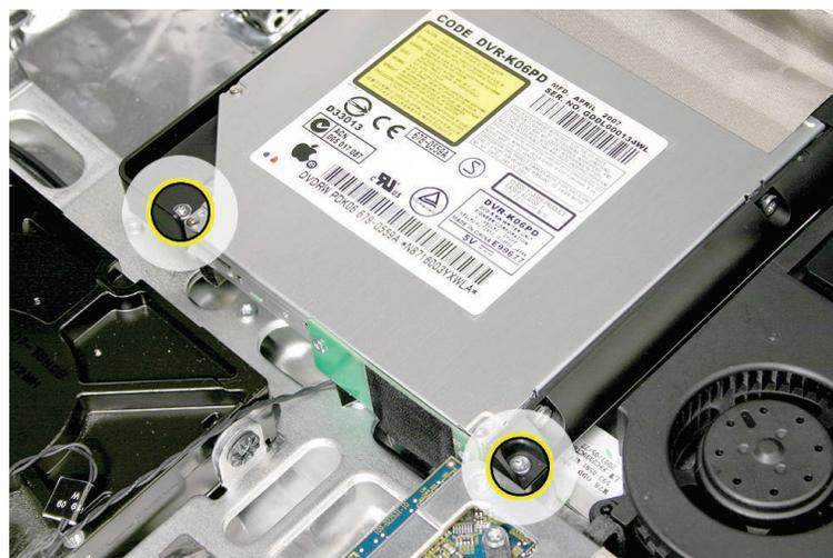
4. Replace the EMI mesh tape. **Important:** Make sure the EMI mesh tape does not cover any of the slot-load opening on the rear cover as you replace the optical drive into the computer assembly.
