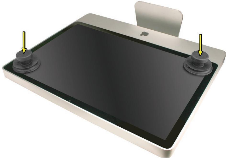
5. Hold onto the suction cups and gently lift the glass panel **straight up and off the bezel**.
