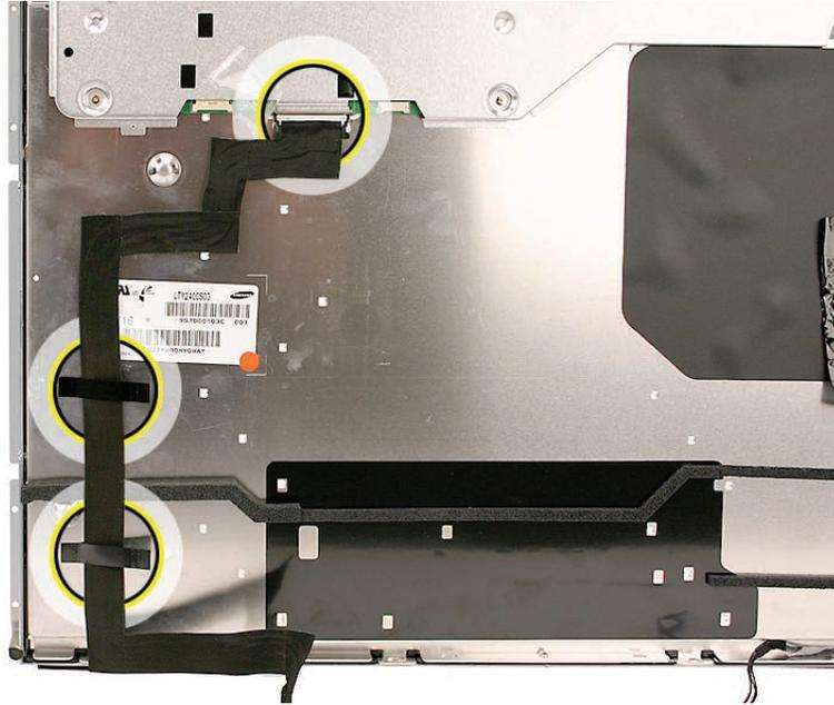
2. Press in on the LVDS connector lock release clips (1) and gently pull (2) to disconnect the LVDS cable from the back of the panel.
