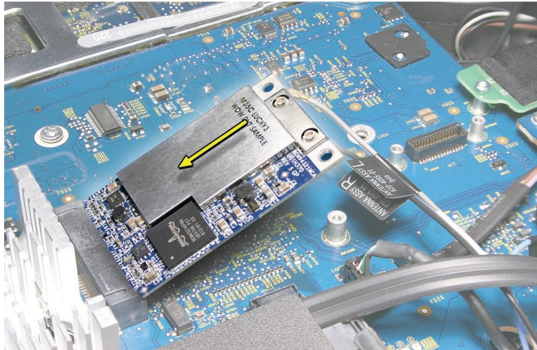
2. Connect the antenna cables to the connectors on the AirPort Extreme card.
