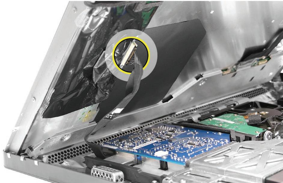
4. Make sure the other end of the inverter cable is connected to the power supply.
