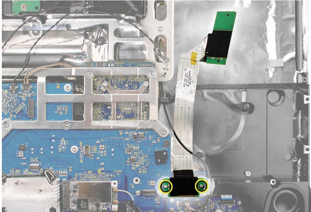
2. Lift the flexible cable out of the rear housing.
