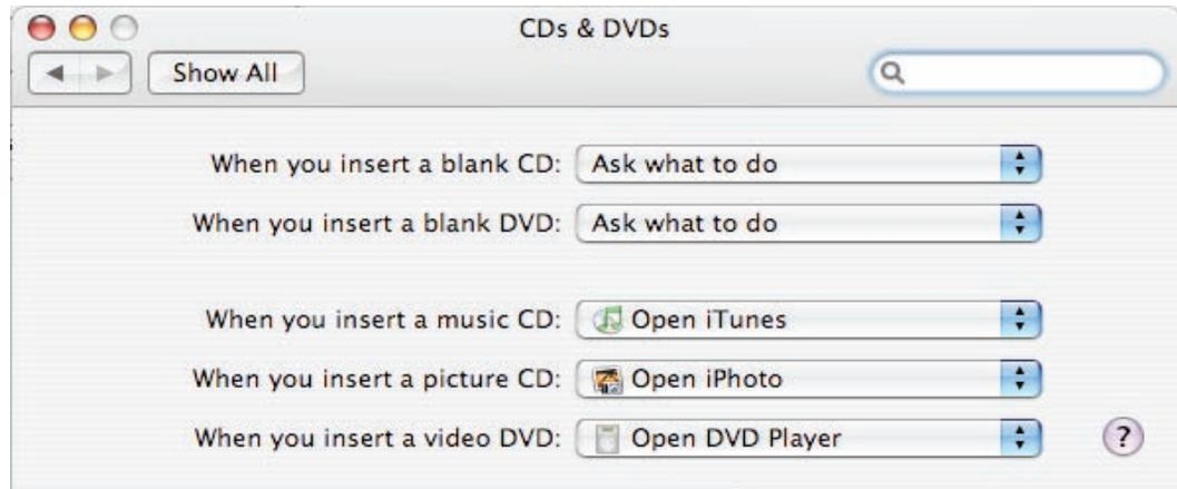
3. Check that the drive can read discs normally. Insert an audio CD and check whether it shows up on your desktop or launches iTunes.
