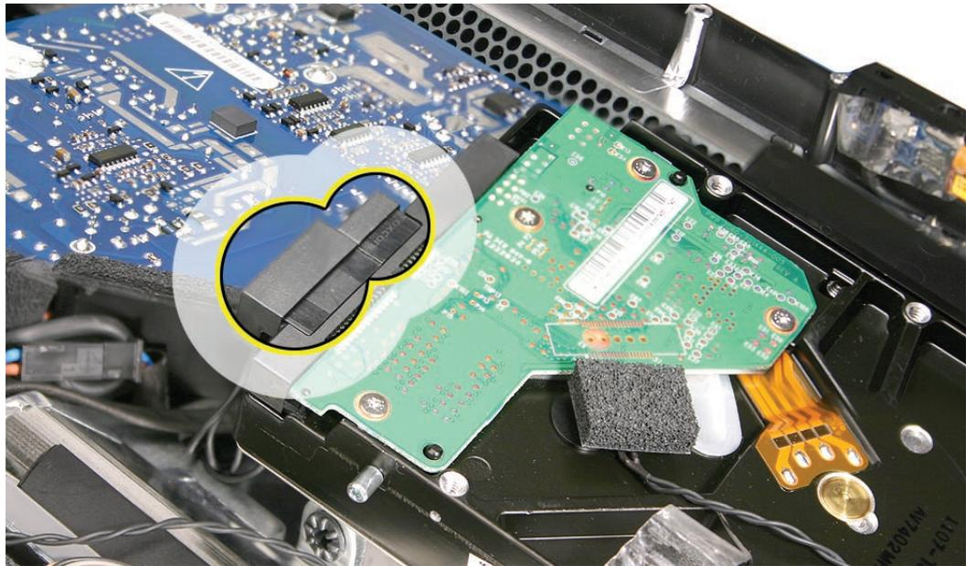
4. Press the hard drive the rest of the way into the rear housing. You will hear a snap when the black plastic clip at the top hard drive clicks into place on the chassis.
