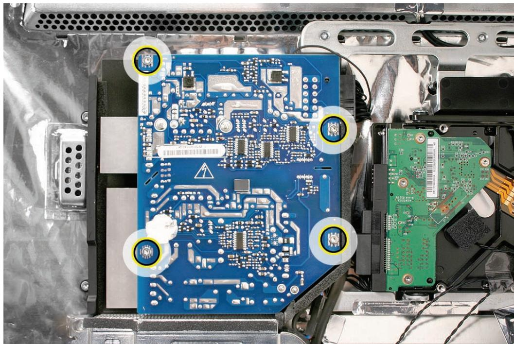
3. Lift the power supply up to access the connectors on the underside. Pinch the black tab on the AC/DC power cable connector (the bigger connector) to disconnect the cable. Carefully remove the small ground connector cable from the underside of the power supply. (See next photo for a close up.)
