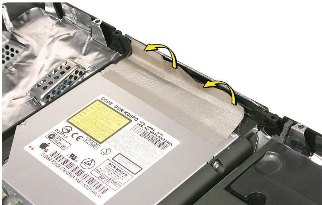
3. Tilt up the optical drive, remove the two T6 screws on the flex cable board. Remove the flex cable board from the optical drive.
