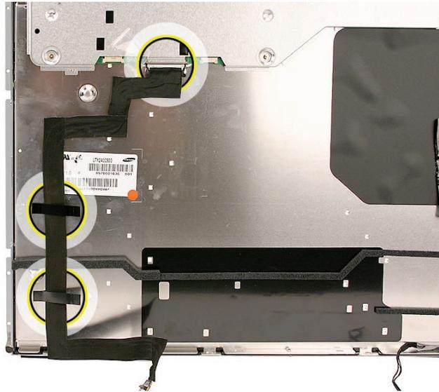
7. On the right side of the panel is the display temp sensor (under the foam gasket at the top) and the display temp sensor cable. These are included with the LCD panel, but they are also offered separately as service parts.
