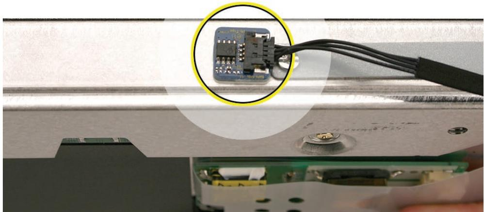
2. Route the cable along the right side on the back of the panel. Press the black sticky insulator over the top of the cable and the sensor. Replace any clear tape holding the cable in place on the panel..
