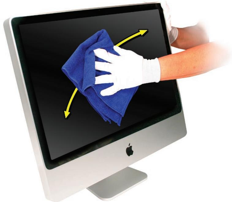
9. Once the glass has been cleaned and polished, visually inspect the glass for any remaining dust, fingerprints, or a hazy residue. If there are contaminants trapped between the LCD panel and the glass panel repeat the cleaning procedure described in this section before returning the system to the customer.
