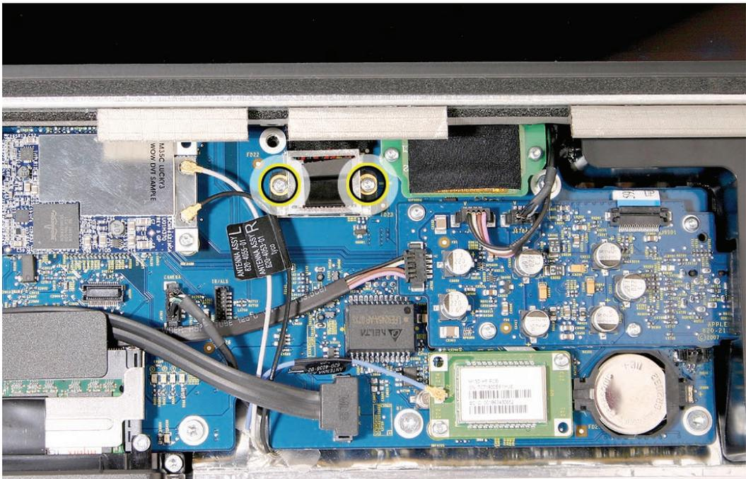
7. Connect the LCD temp sensor cable to the bottom left corner of the logic board. Tuck any extra length of the cable in the area between the CPU fan and the edge of the logic board.
