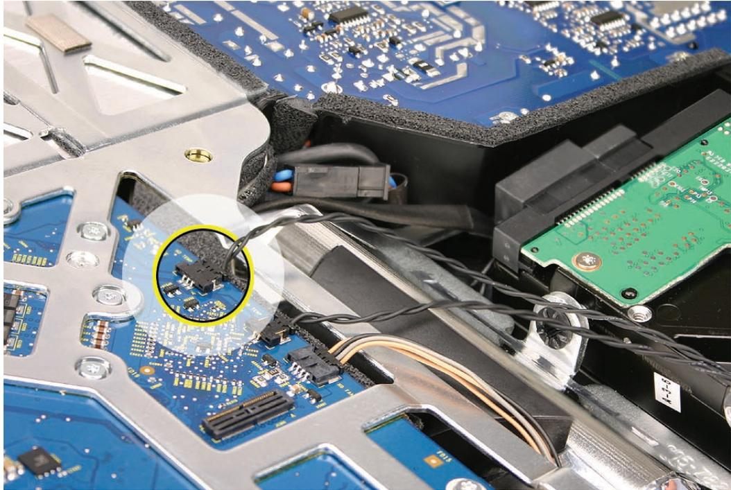
2. Peel back the foam gasket on top of the hard drive. Remove the sensor cable from the sensor clip.
