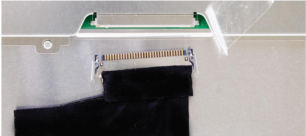
2. Replace the clear Kapton tape over the LVDS cable connector.
