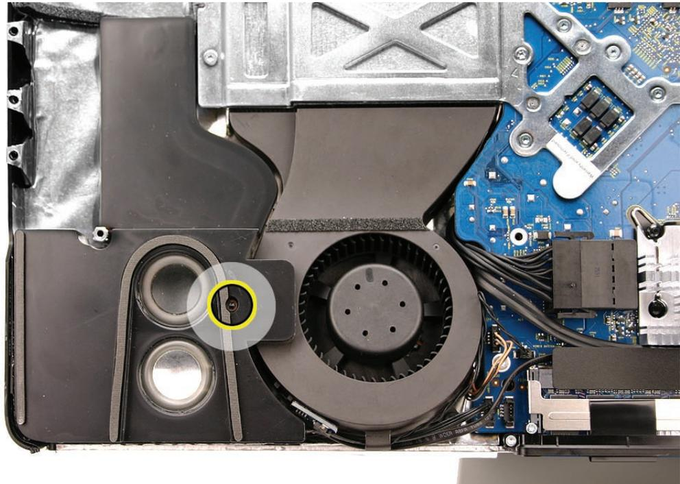
2. Disconnect the speaker from the audio board. The speaker cable runs under the black plastic cable guide (above the memory slot) and connects to the audio board on the right side of the logic board.
