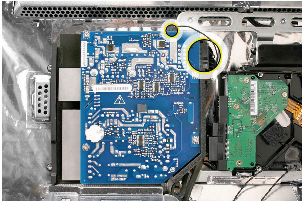
5. Replace the four T10 power supply screws. Install the machine screws (on the right side) first when installing the power supply.
