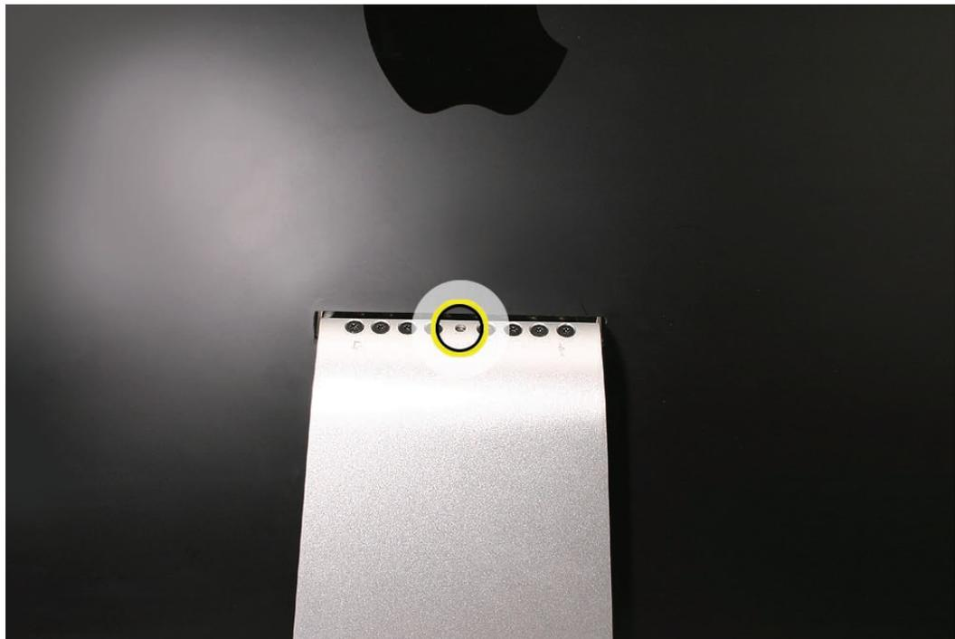
5. Install the eight long, clutch-to-stand mounting screws.
