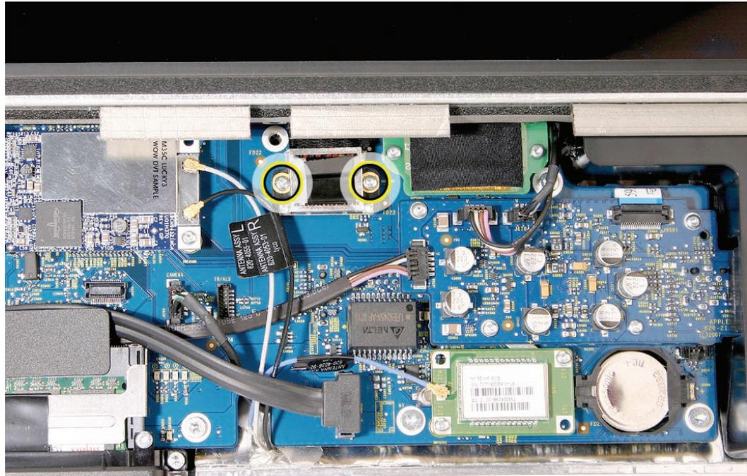
7. Connect the display temp sensor cable to the left side of the logic board.
