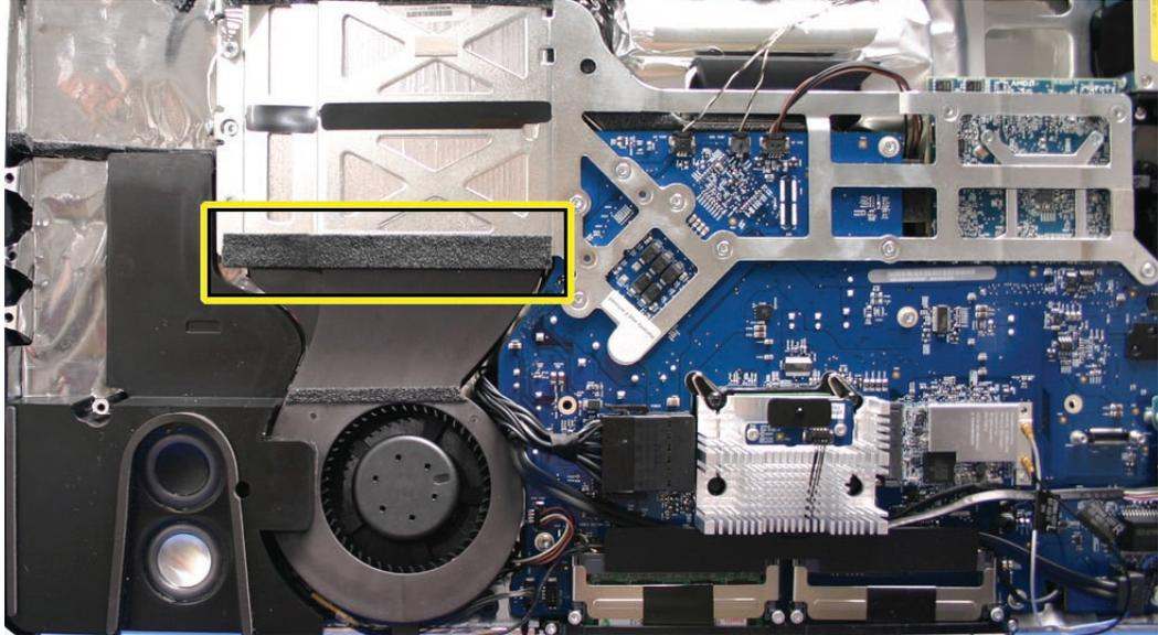
3. Connect the ambient temp sensor cable and the fan cable to the logic board connectors.
