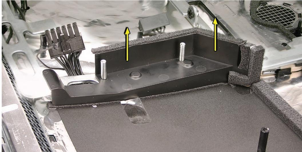
2. Remove the chassis screws. **Note:** The three screws across the top of the chassis have a flatter head than the other chassis screws.
