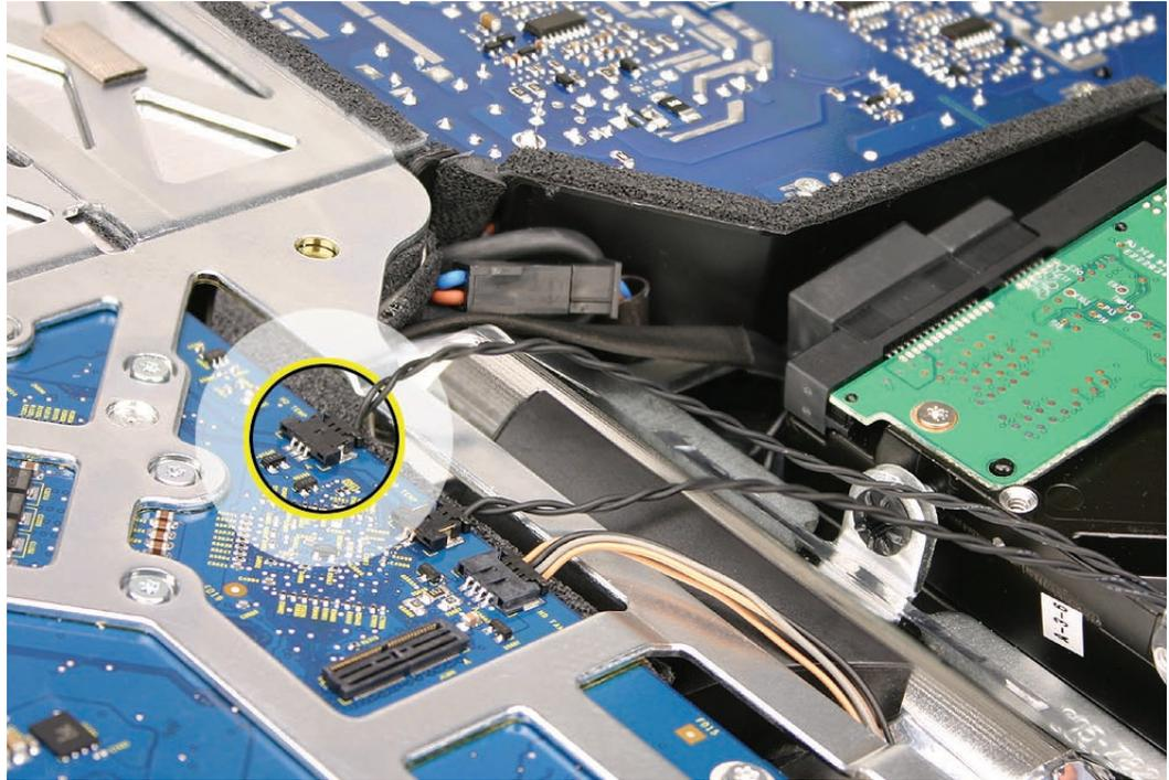
2. Push HARD and toward the logic board on the black plastic clip at the top of the hard drive to release it from the chassis.
