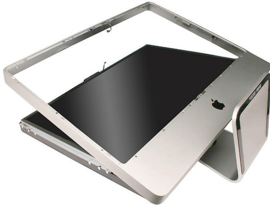
5. Replace the twelve screws around the bezel. The two longer screws (30mm) attach to the bezel along the bottom of the panel, on the right and left side of the Apple logo. The four medium length screws (19mm) attach above and below the optical drive on the right side, and on either side of the 30mm screws. The six shorter screws (15mm) attach around the top, and left side.
