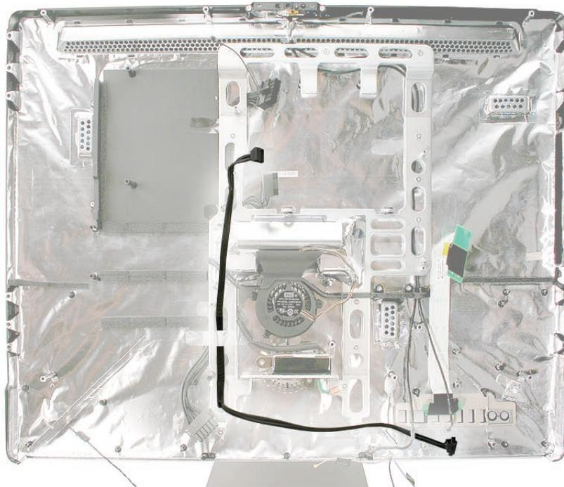
2. Secure the cable to the chassis with kapton tape.
