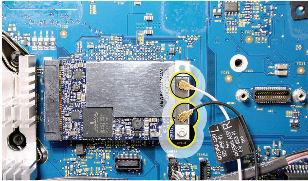
2. Holding the card by the edges, pull the AirPort Extreme card out of the slot.
