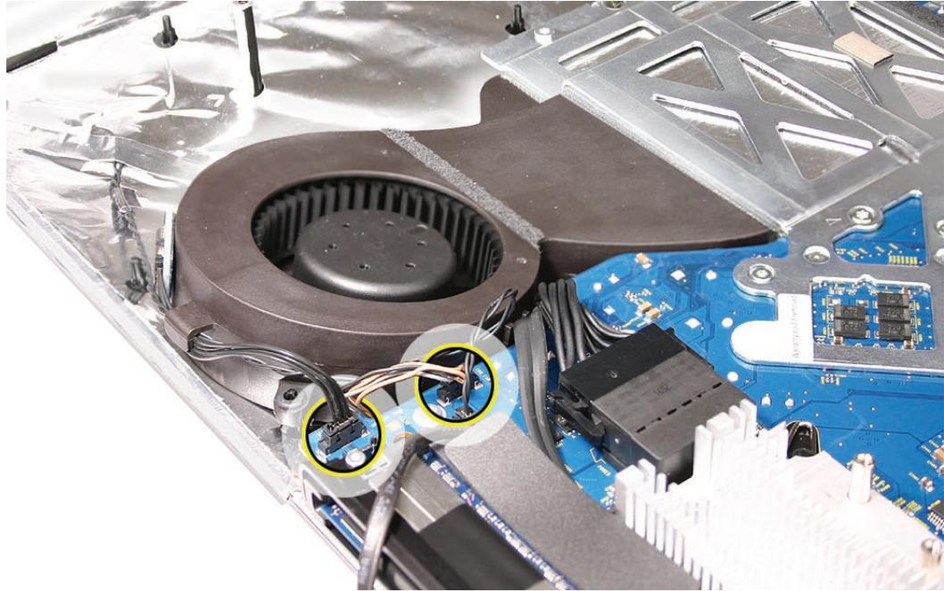
2. Disconnect the cable from the sensor board on the speaker.
