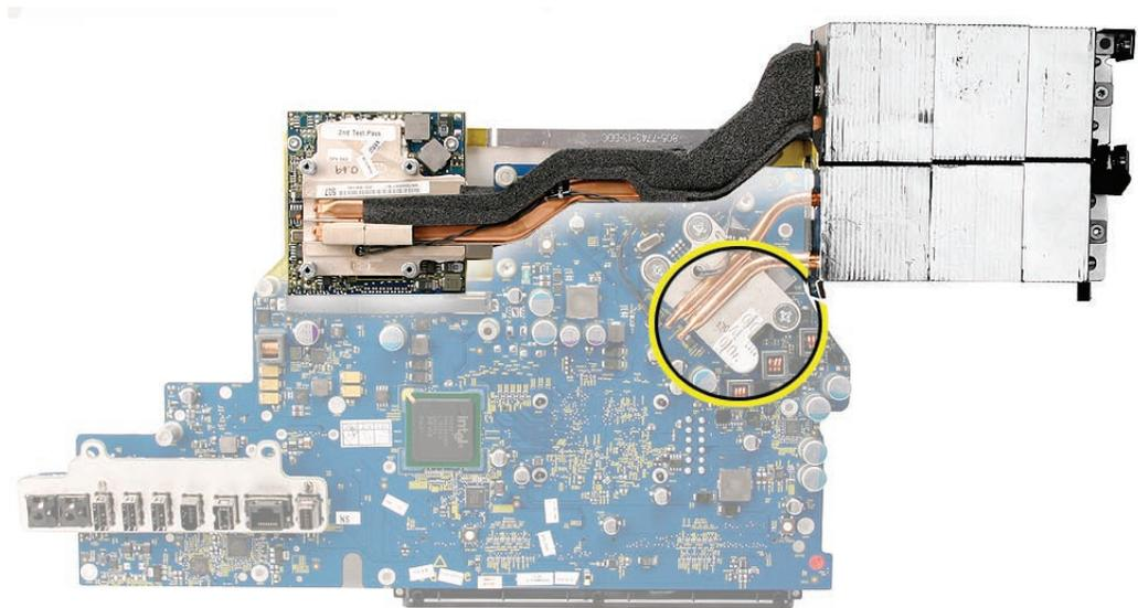
9. This shows the tamper-proof label on the top side of the logic board.
