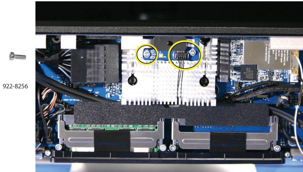
2. Lift the IR board from the heatsink.
