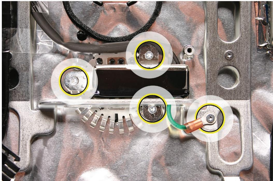
5. [Replace the power supply](#), and connect the AC power inlet cable.
