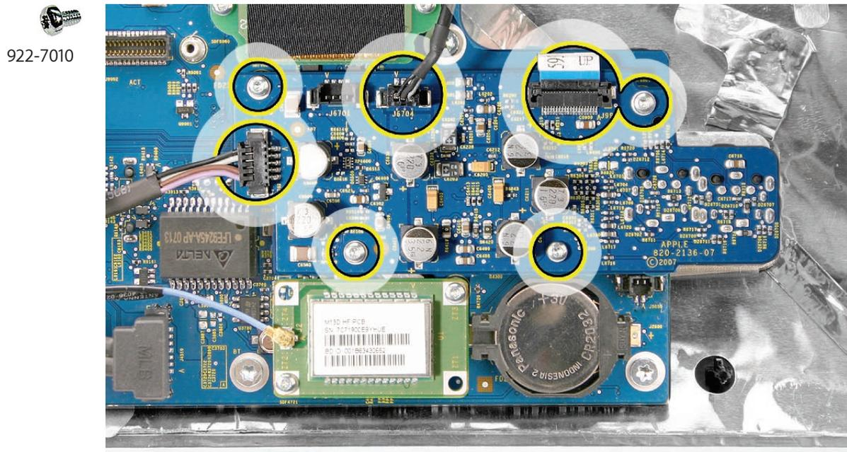
3. Lift the audio board off the logic board.
