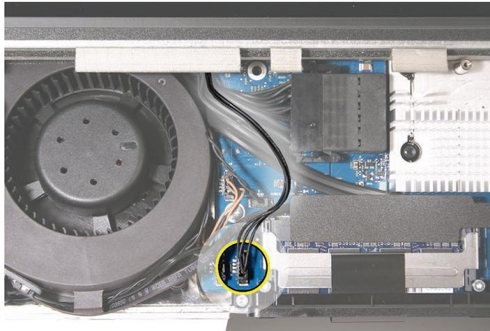
3. Boot to the EF1 tests of the latest version of Apple Service Diagnostic, version 3S116 This will test the fans and thermal input of the sensors. If the tests fail, replace the component(s) indicated by the test.
