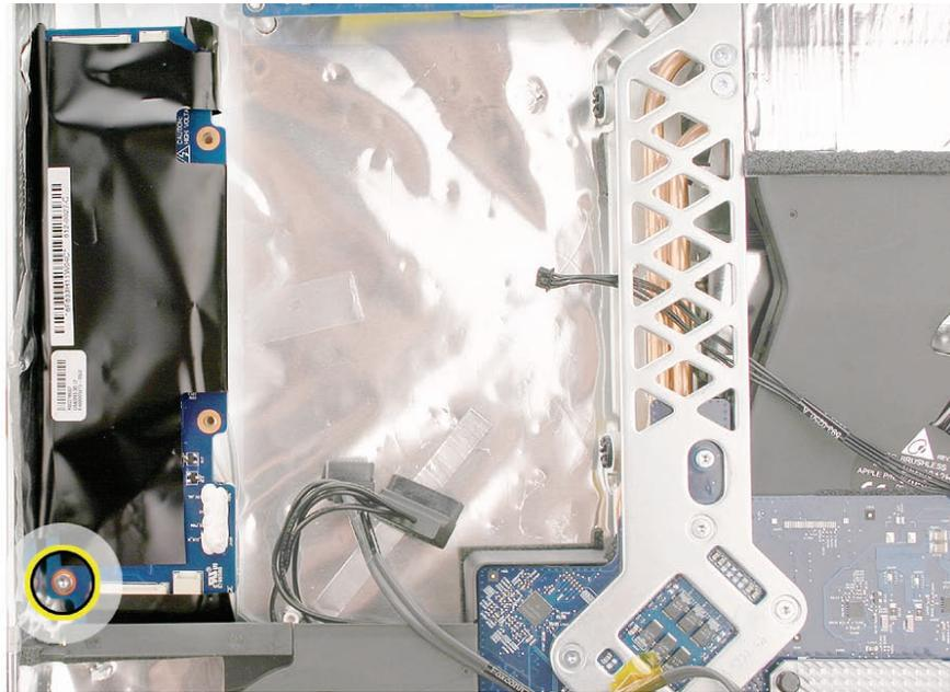
2. Flip over the inverter board to locate the inverter-to-DC cable connector. Disconnect the cable; lift the inverter out of the rear housing.
