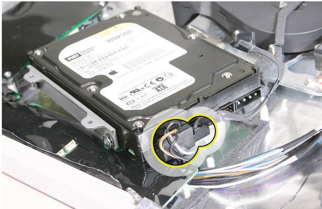
3. Route the hard drive sensor cable under the metal chassis. Connect the sensor cable to the logic board.
