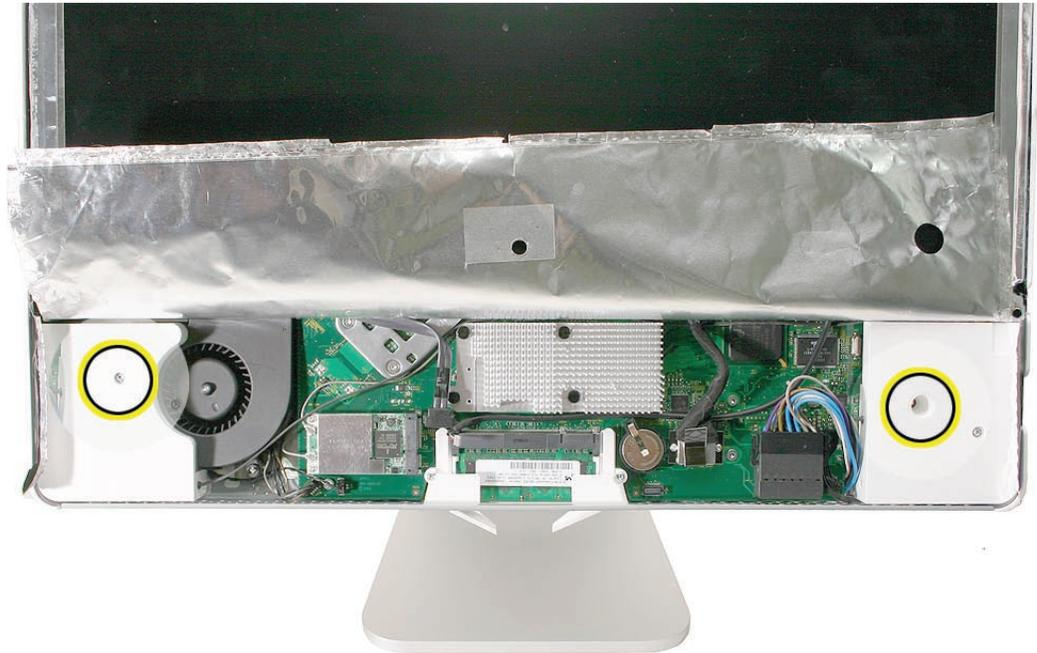
2. Remove the two T6 screws on the IR mounting bracket so the speaker cable insulation is not sliced on the metal bracket.
