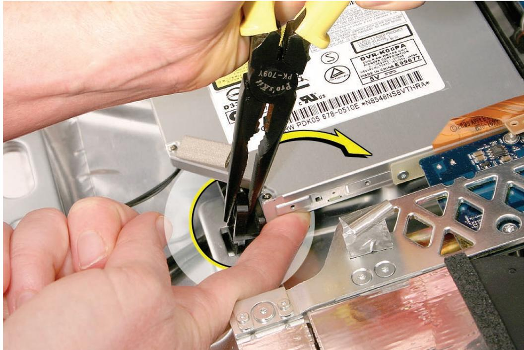
**Warning:** iMac main logic boards returned with physical damage such as scratches, fractures, or broken or missing components caused by improper servicing may be classified as customer abuse. When using a tool to release the latches, be careful not to apply pressure to the logic board or it may be damaged.
