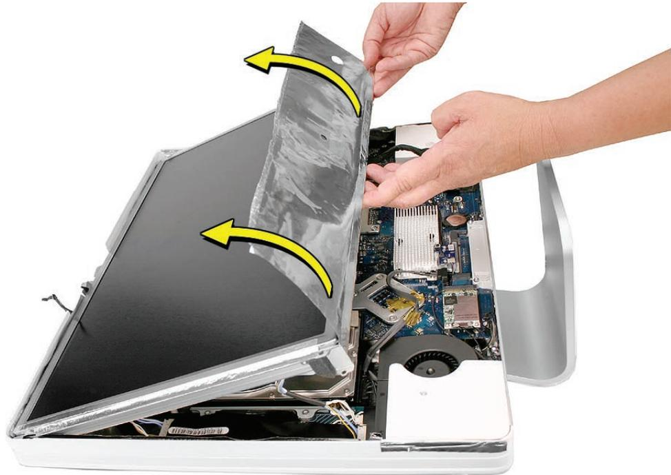
6. Disconnect the two panel-to-inverter cables above the left speaker. **Replacement Note:** The cable connectors are marked with dots to indicate “right-side-up.”
