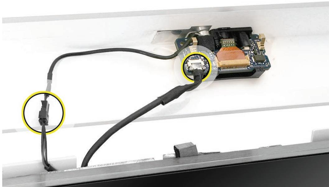
12. Lift the front bezel off the computer. If replacing a damaged front bezel, also remove the camera board. **Note** the microphone is part of the front bezel assembly.
