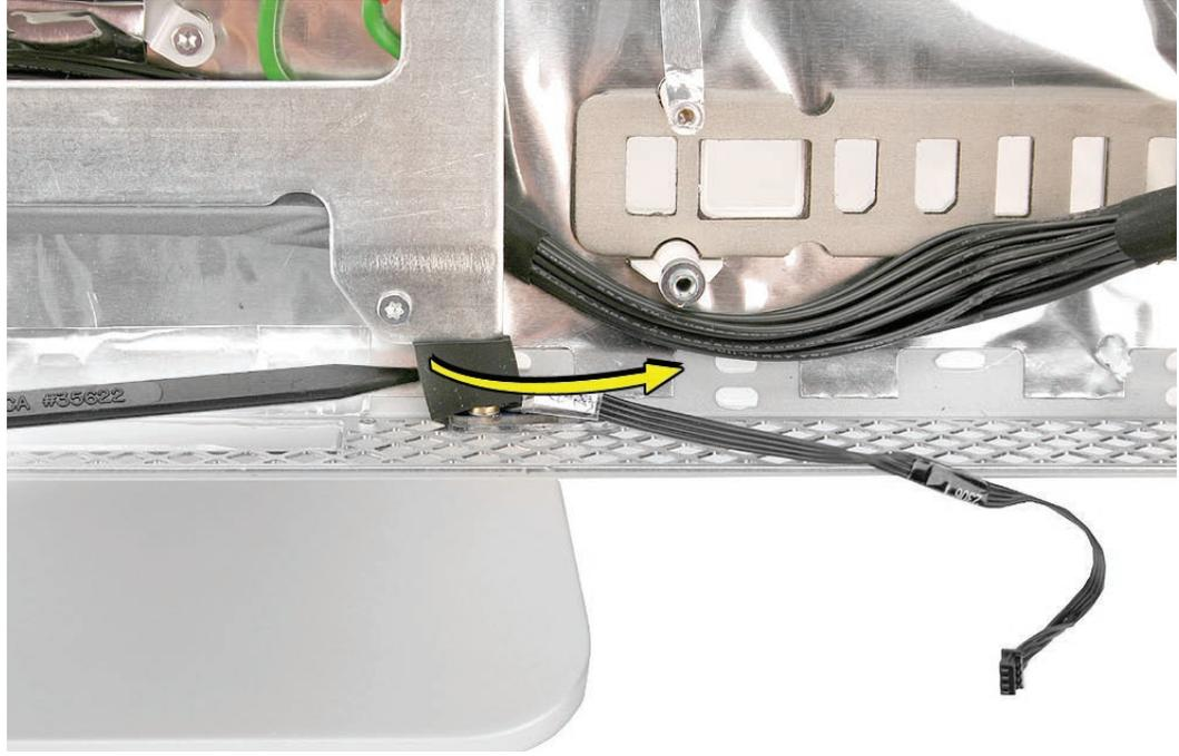
2. With the rubber bumper gone, use a black stick, pry the ambient light sensor off the inside of the rear housing. **Note:** Never poke the ambient light or you could damage the sensor board.
