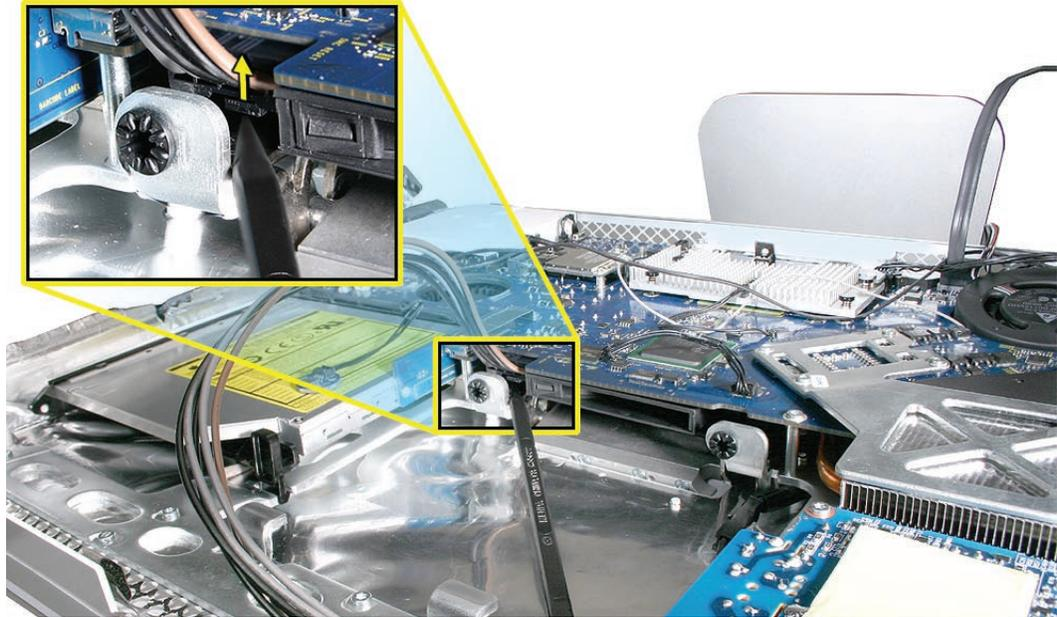
4. Pull the board toward you and slightly lift the board up. **Note:** The I/O ports fit tightly into the port hole openings on the rear cover. You may have to fidget with the board a bit to free the ports from the rear cover. Remove the logic board out of the rear housing.
