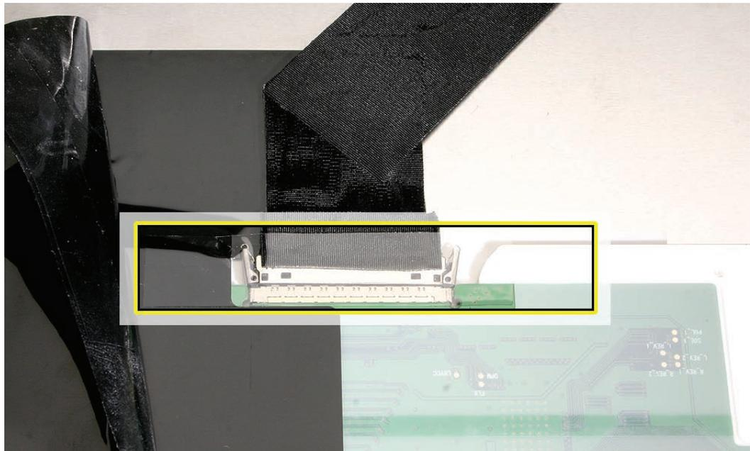
10. Pinch together the connector locking levers, and disconnect the LVDS cable connector.
