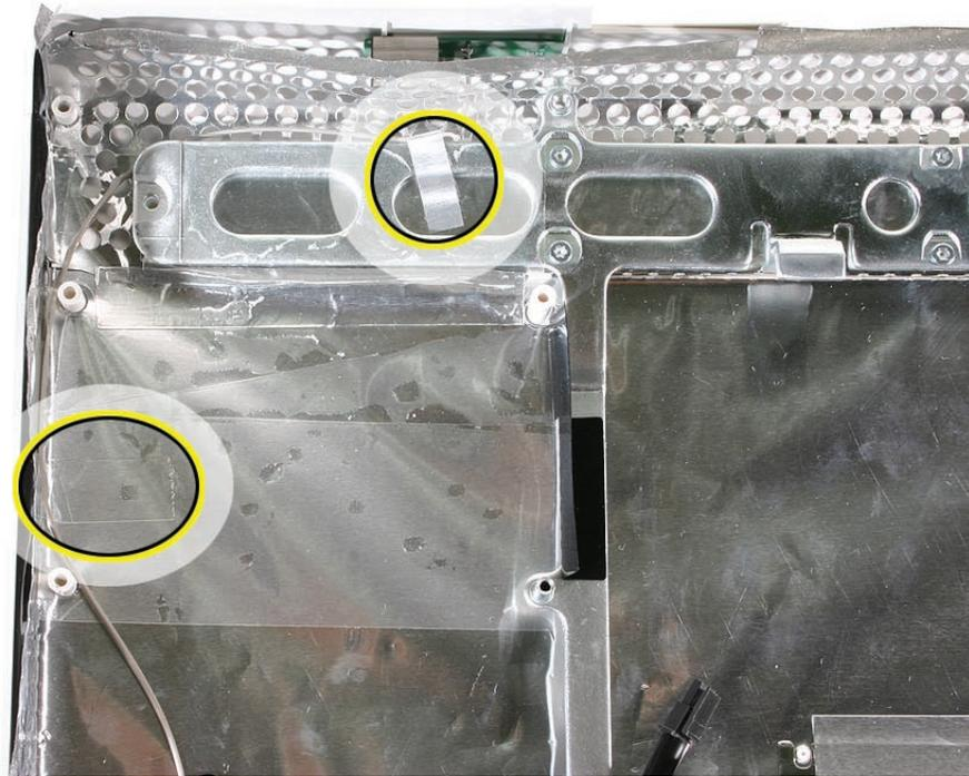
2. Remove any tape that secures the antenna cable to the rear housing.
