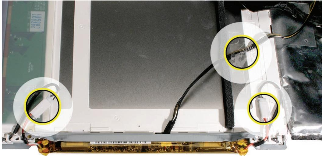
7. Turn over the panel. If the lower EMI shield was removed, reattach the lower EMI shield across the bottom of the panel.
