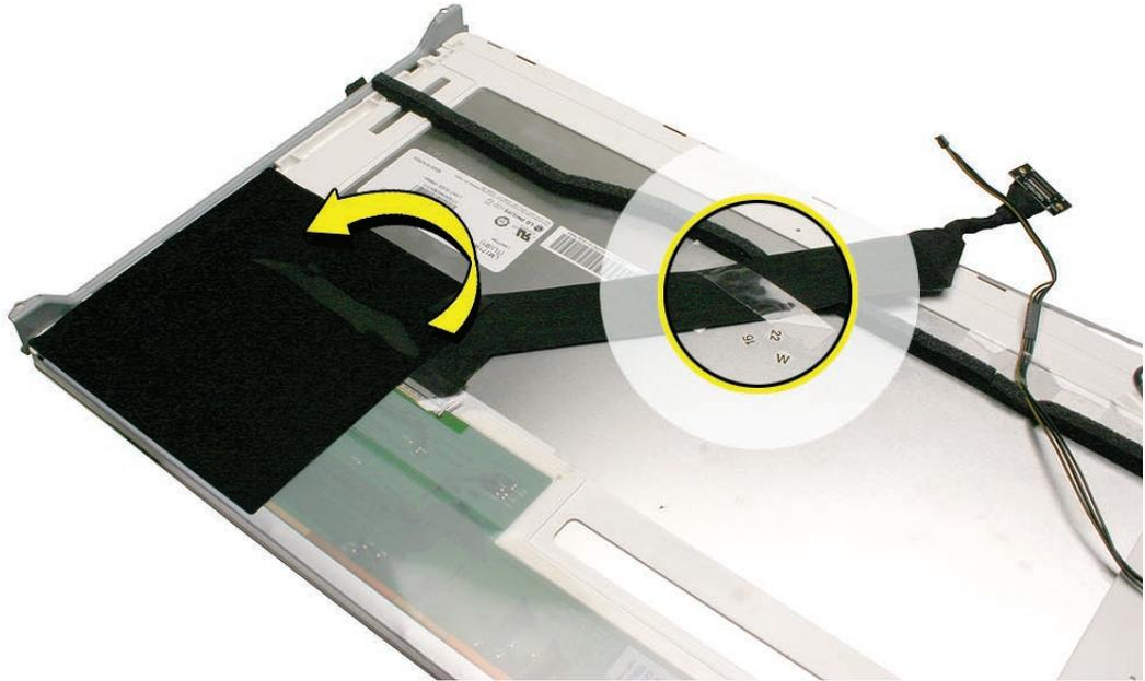
9. Remove the tape securing the LVDS connector to the panel connector.
