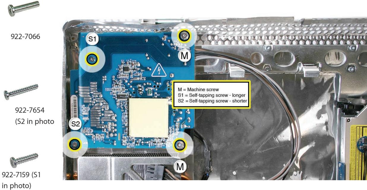
4. Remove the power supply from the enclosure.
