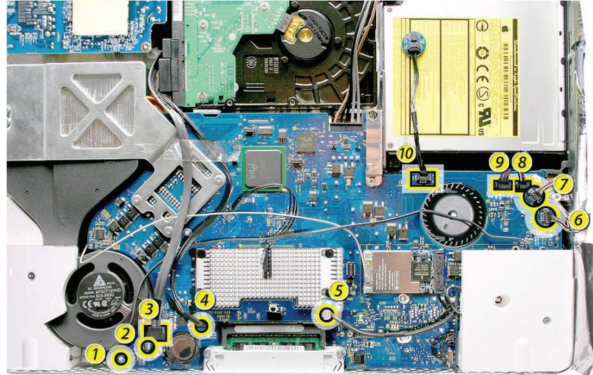
2. Using a T10 torx screwdriver, remove the screws from the logic board. Note the locations of the three self-tapping screws (marked by "S" in the photo). The rest of the screws are machine screws.
