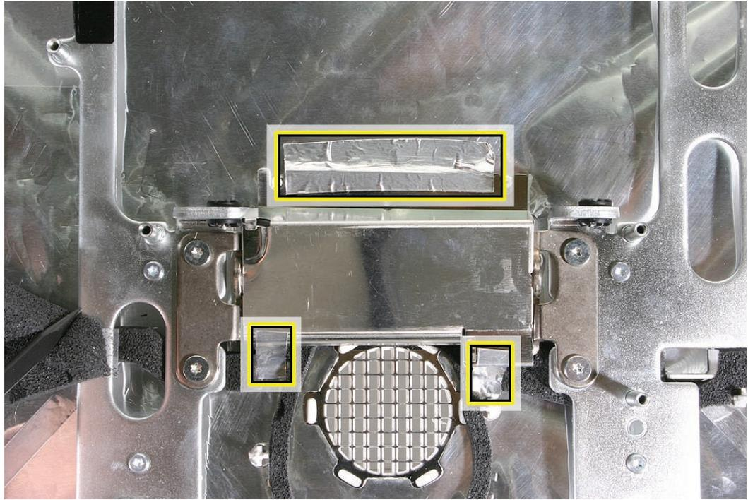
2. Remove the metal clutch cover.
