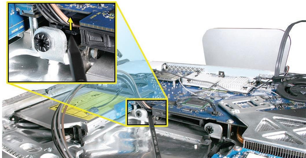
3. Using a T8 screwdriver, remove the two self-tapping screws on the left side of the power supply board and the two machine screws on the right side of the board. **Note:** Self-tapping screw labeled S1 is longer than self-tapping screw S2.
