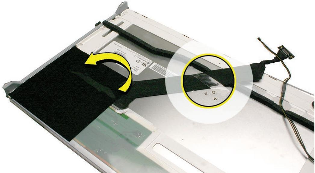
2. Remove the tape securing the LVDS connector to the panel connector.
