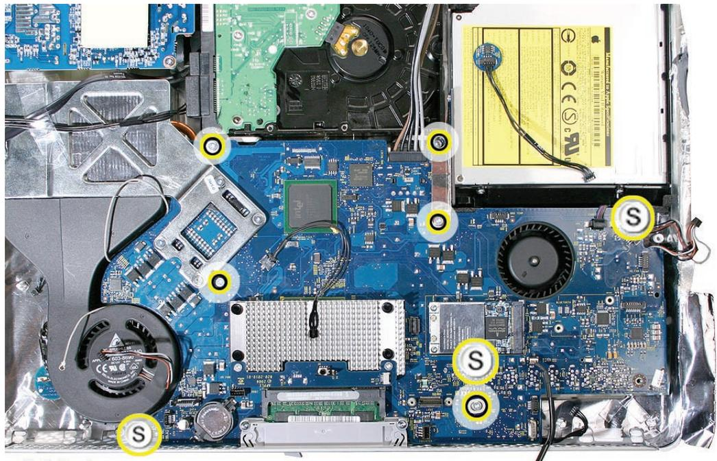
4. Connect all the cables. **Note:** The speaker cable is attached under the right speaker.
