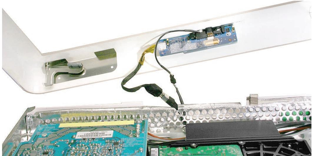
2. Route the camera cable around the hard drive and under the chassis (as shown). Connect the two cables to the connectors on the logic board.
