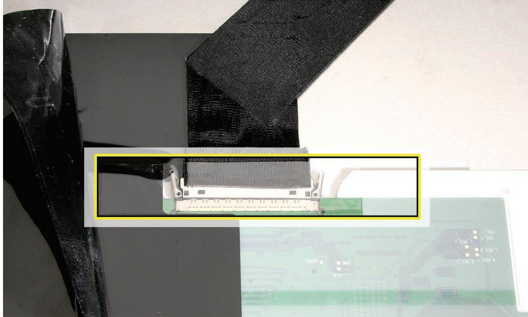
3. If you are replacing the display, a piece of black mylar is enclosed in the box with the display module. The dotted lines below show the correct placement of the mylar. **Note:** The LVDS locking lever (on one side) should be covered by the mylar when positioned correctly.
