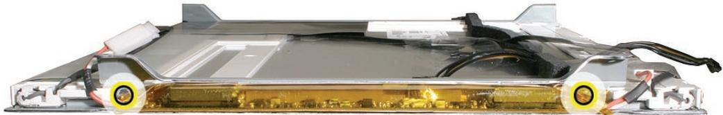
7. Peel back the tape where shown below, and disconnect the two white inverter-to-display cable connectors.
