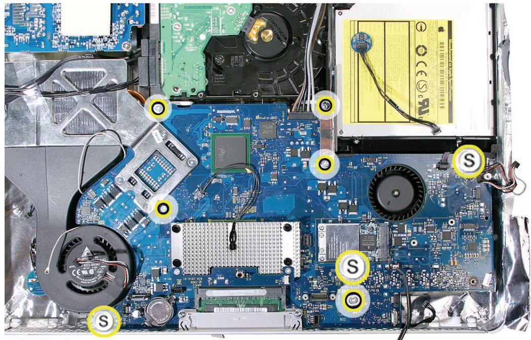
3. Rotate the unit so the power supply is in the bottom right corner and the optical drive is on your left. With a black stick, disconnect the power supply cable on the underside of the logic board.
