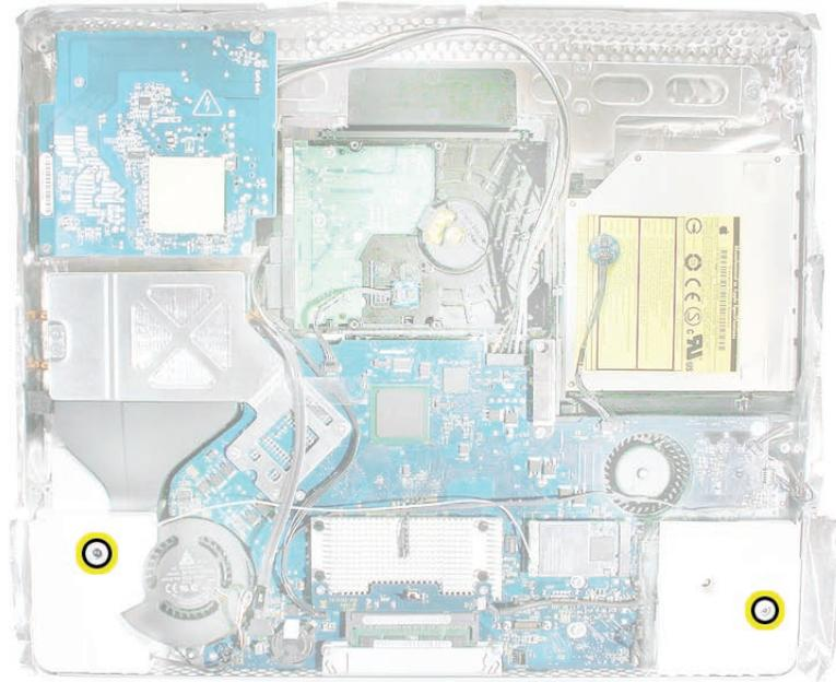
2. Lift the speakers straight up and disconnect the speaker cable under the right speaker.
