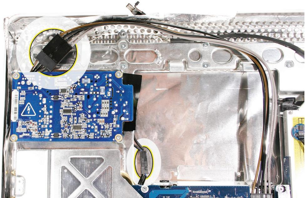
2. Using a T10 screwdriver, Remove the T10 AC power inlet ground-to-chassis screw.
