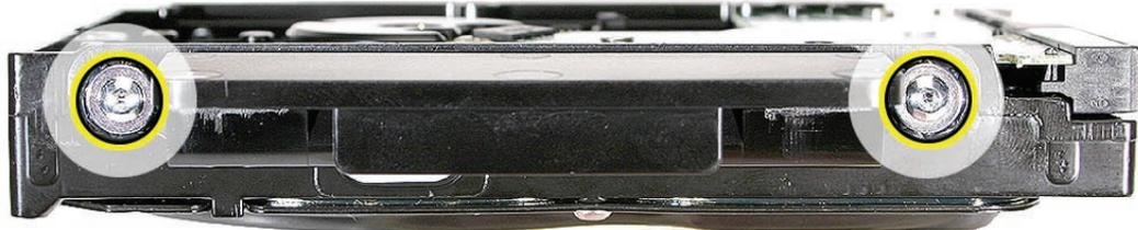
6. Using a T8 torx screwdriver, remove two mounting pins from the other side of the drive.
