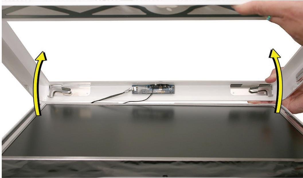
2. Disconnect the camera and microphone cables.
