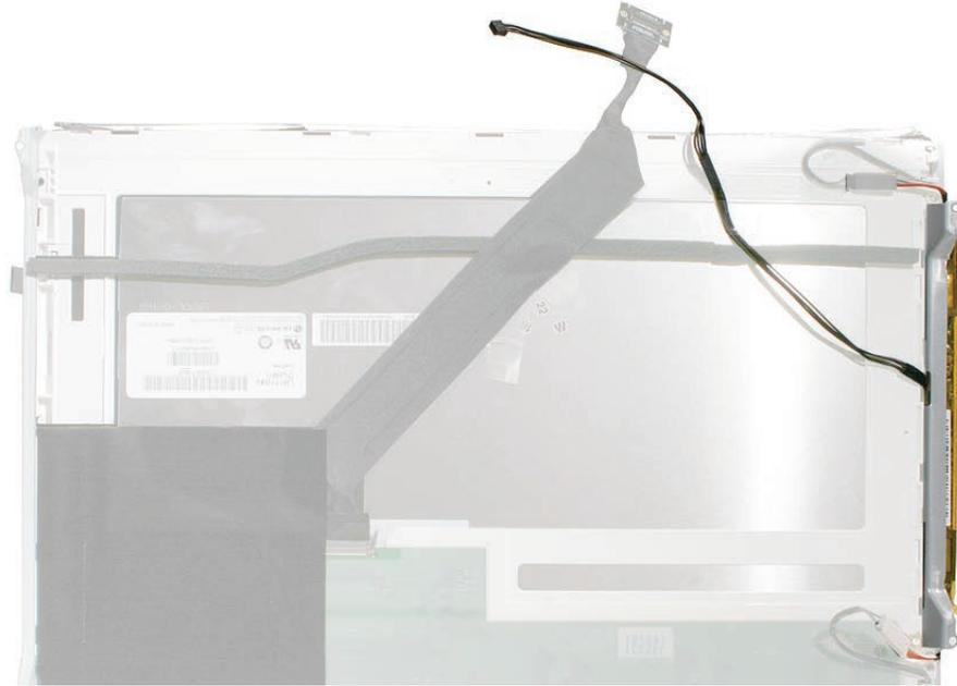
2. Connect the LVDS cable connector. When connected correctly the locking levers will secure the connector and it cannot be disconnected without depressing the levers.
