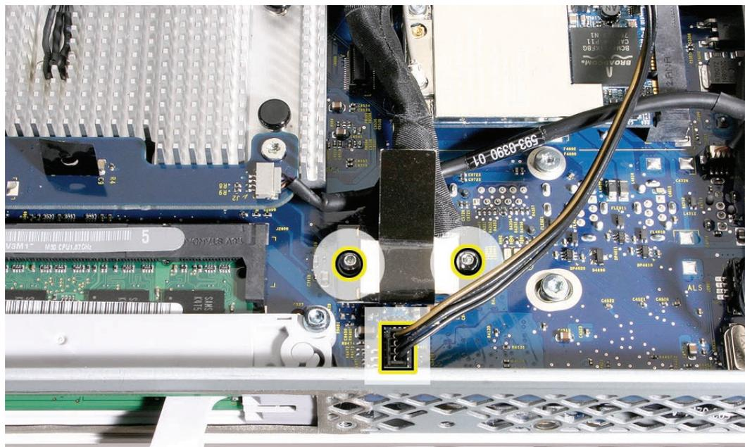
3. Peel the EMI tape away from each side of the panel. Using a Torx T10 screwdriver, remove the four panel mounting screws.
