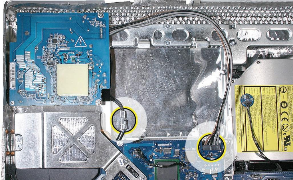
2. Rotate the computer so that the stand is away from you. Locate the power supply connector underneath the logic board. Use a black stick to release the connector.
