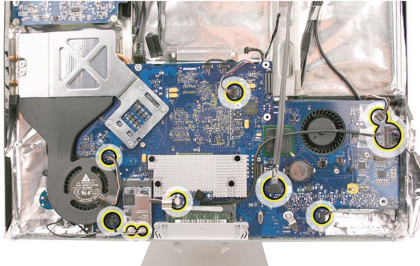
2. Using a T10 torx screwdriver, remove the screws from the logic board. The locations of the three self-tapping screws are marked by an “S” in the photo. The remaining three screws, are machine screws; they are marked with an “M.” **Note:** Transfer the small metal grounding (located two screws below the battery) clip to the replacement logic board.
