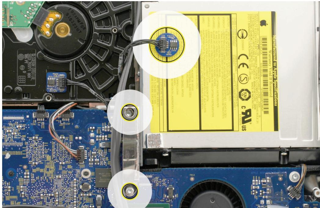
2. **Note:** Make sure to use a needlenose pliers with teeth to remove the optical drive. The pliers must have a textured surface to properly grasp the optical drive release tabs.
