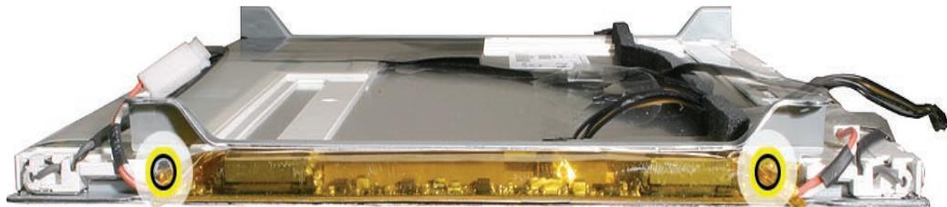
8. Peel back the clear tape and disconnect the two inverter-to-display cable connectors.
