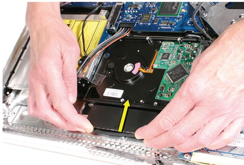
4. Disconnect the hard drive power and data cables. Set the hard drive aside.
