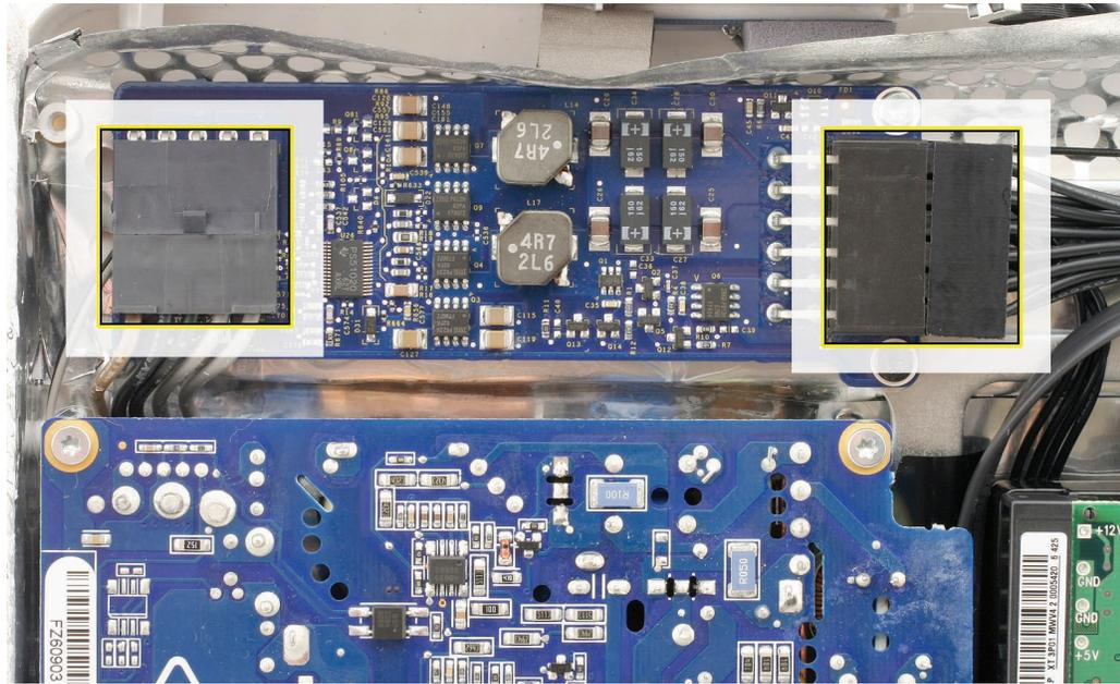
2. Using a T10 torx screwdriver, remove the two self-tapping screw from the bottom corners of the board and the machine screw in the top right corner.
