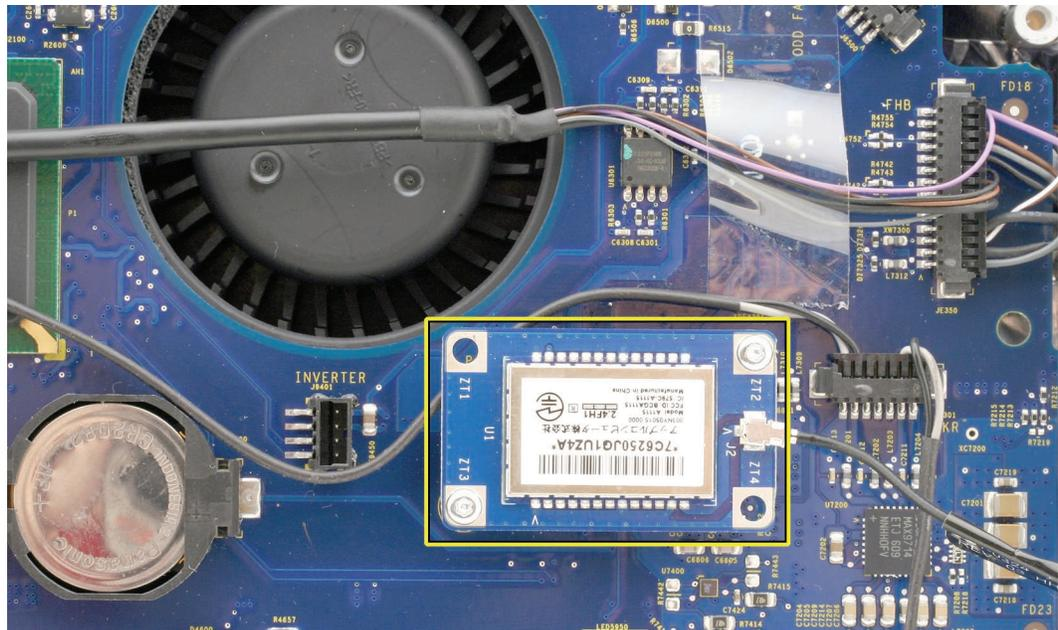
3. Disconnect the speaker cable located to the right of the Bluetooth board.
