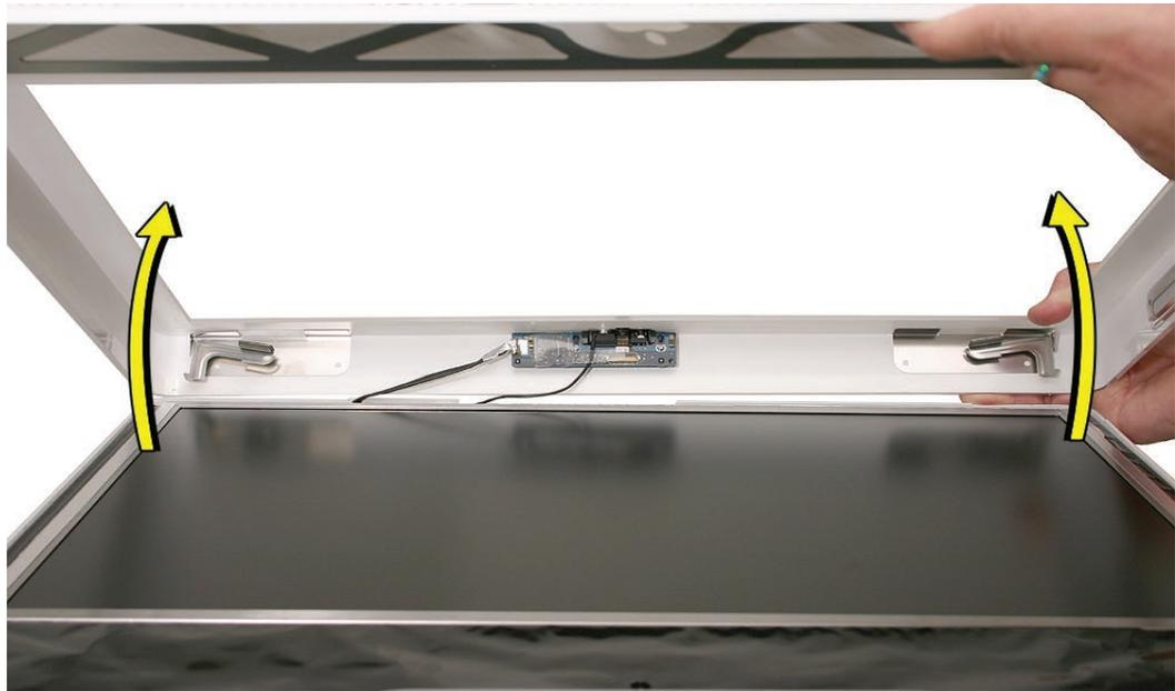
2. Remove any kapton tape wrapped around the cables. Disconnect the camera and microphone cables.
