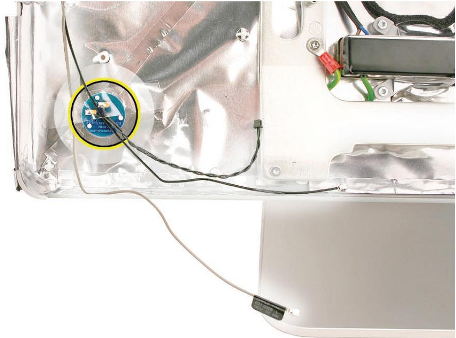
4. Pull the antenna cables through the access hole in the EMI shield at the top, near the antenna board.
