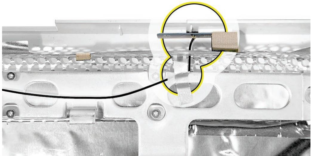
3. Remove any other tape that secures the antenna cables to the rear housing.
