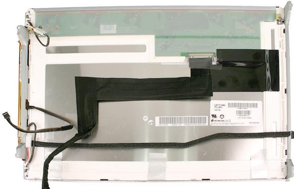
2. If you are replacing the display, a piece of black mylar is enclosed in the box with the display module. The dotted lines below show the correct placement of the clear tape and black mylar.
