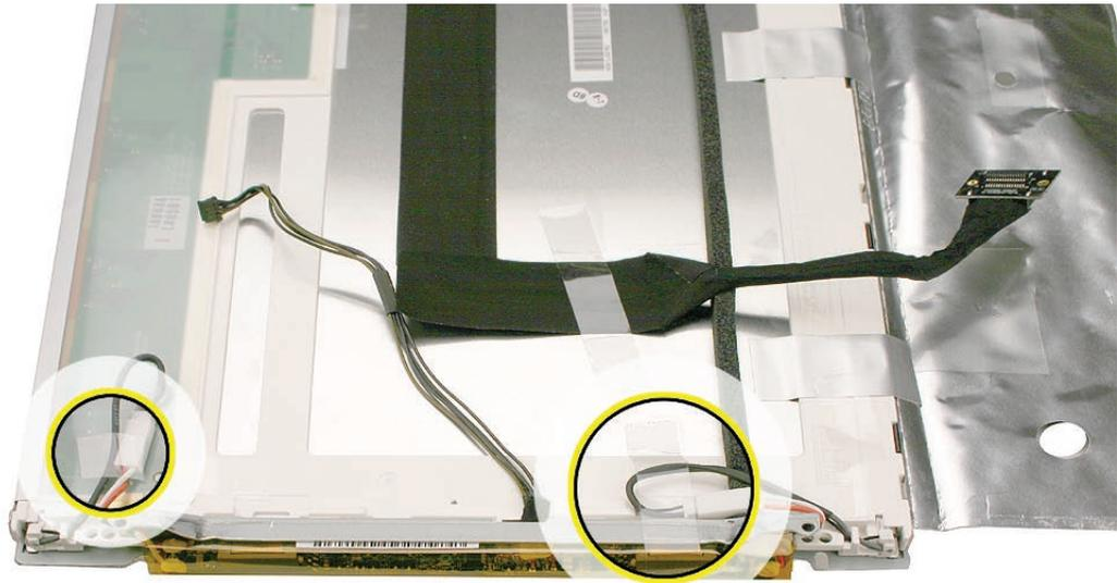
9. To access the LVDS cable connector, peel back the clear tape and the black mylar (if necessary). Pinch together the connector locking levers, and disconnect the LVDS cable connector.
