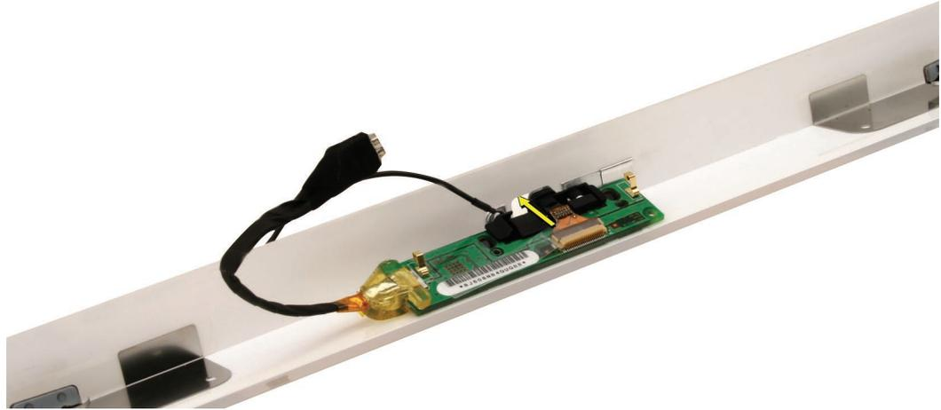
2. Install the camera board to the bezel with two T6 mounting screws.
