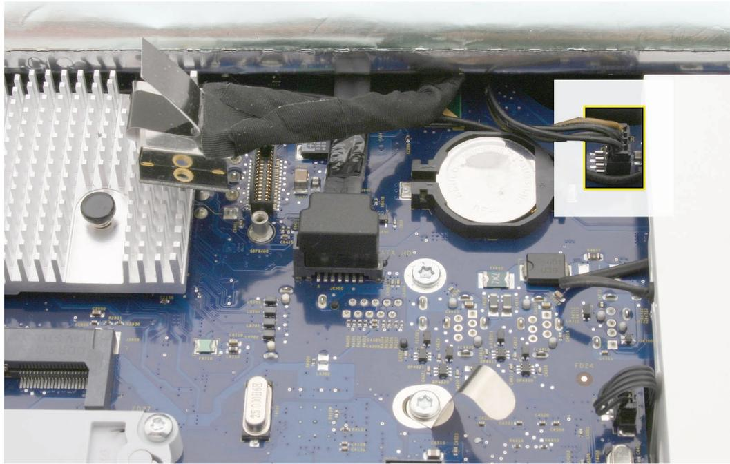
4. Using the access card or a black stick, peel the EMI tape away from each side of the panel. Remove the four panel mounting screws with a T10 screwdriver.
