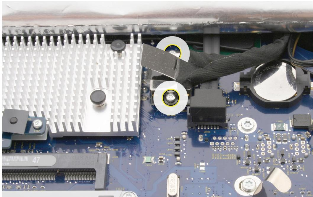
3. To the right of the battery is the inverter cable connector. Disconnect the inverter cable from the logic board.
