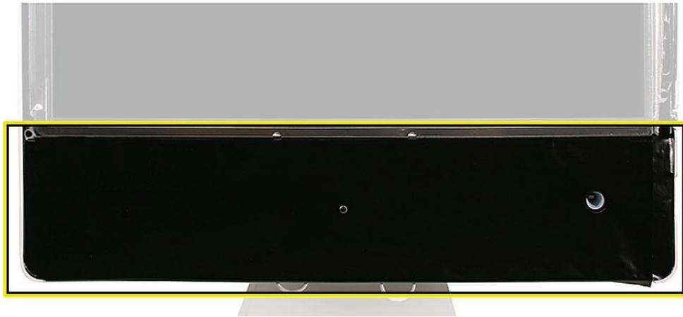
When properly repaired, all edges shown below will be wrapped by EMI tape, and the tape securely adhered to all edges. Use a black stick to flatten the EMI tape tightly and rub out air pockets and wrinkles.
