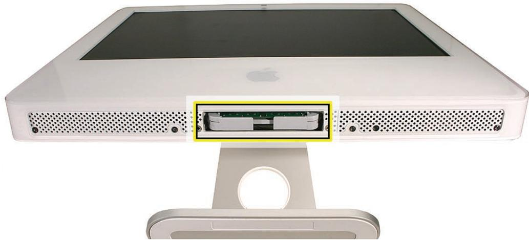
5. Continue to lower the front bezel down and press the top corners of the front bezel to connect the latches. **Note:** Check that the latches are connected by lifting the front bezel at each corner.
