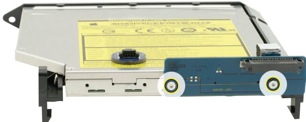
8. If replacing a bad optical drive the replacement drive will have a new sensor installed.
