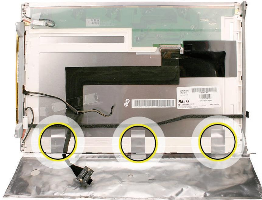
8. Position the panel into the rear housing. Make sure the inverter cable and the LVDS cable are accessible and not tucked under the panel.
