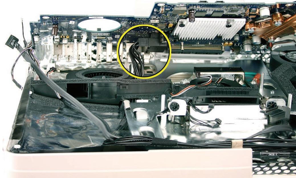
3. Check that the screw holes are aligned with the screw mounts in the chassis. **Replacement Note:** The logic board should rest on the screw mounts without any binding or bowing—if it doesn't, adjust any cables that are interfering with the logic board. Reconnect the ten logic board cables.
