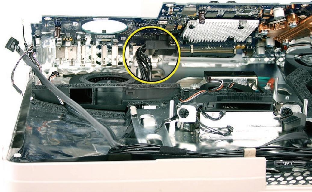
4. Pull the board toward you and gently lift the board up. **Note:** The I/O ports fit tightly into the port hole openings on the rear cover. You may have to wiggle with the board to free the ports from the rear cover.
