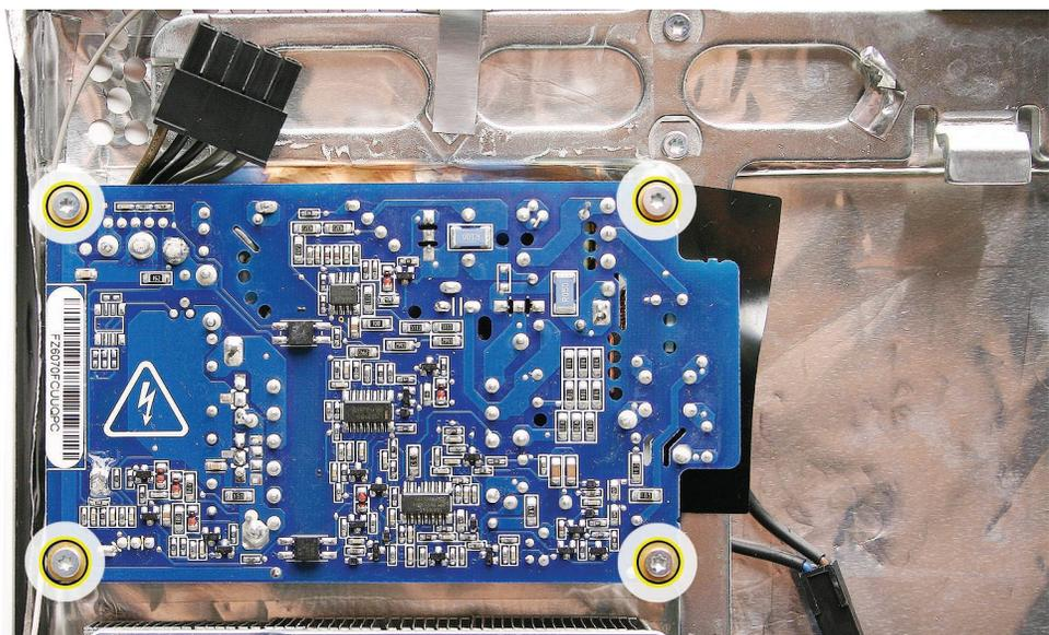
3. Remove the power supply from the enclosure.
