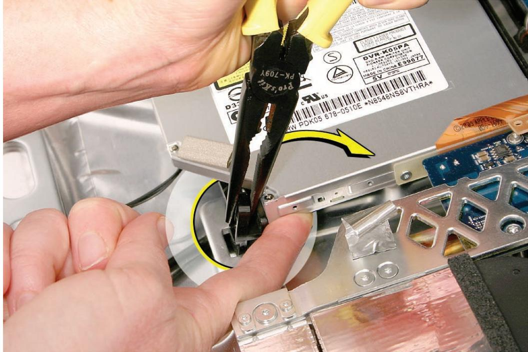
**Caution:** Never press down on or grasp the body (silver) of the optical drive when removing or installing it. Depressing the body of the optical drive could damage the mechanism. Grasp the optical drive by its mounting bracket only.
