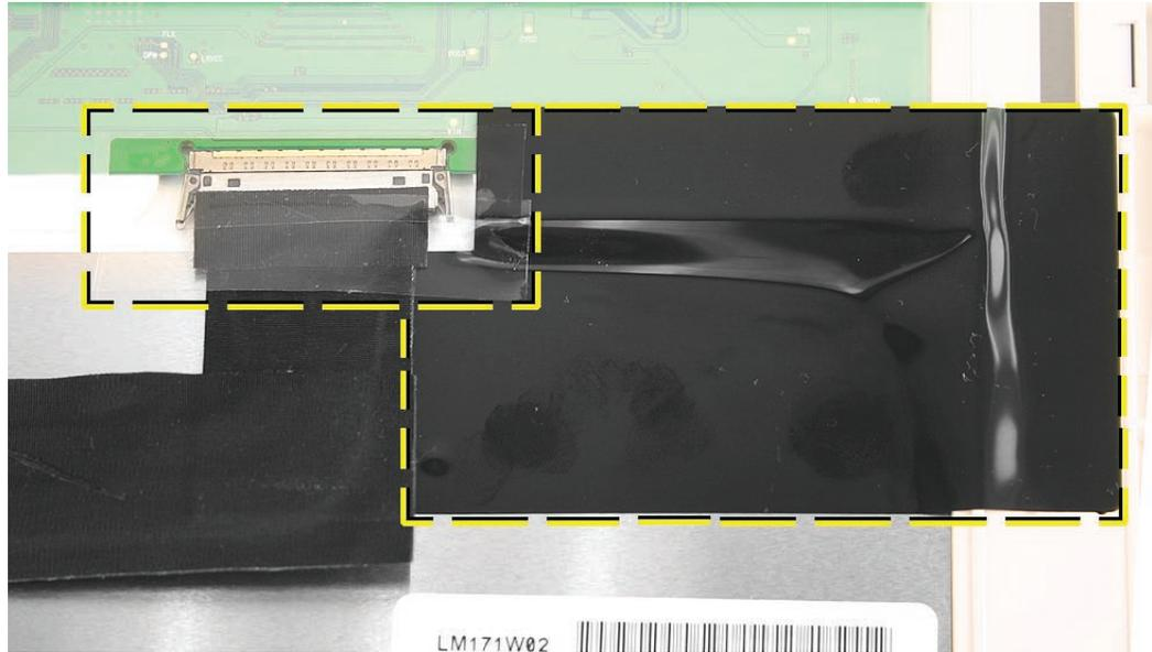
2. Pinch together the connector locking levers, and disconnect the LVDS cable connector.
