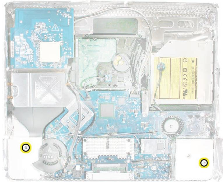
2. Lift up the right speaker. The speaker cable routes under the Bluetooth board. Remove the two T6 screws on the Bluetooth board. Lift the Bluetooth board to access the speaker cable.
