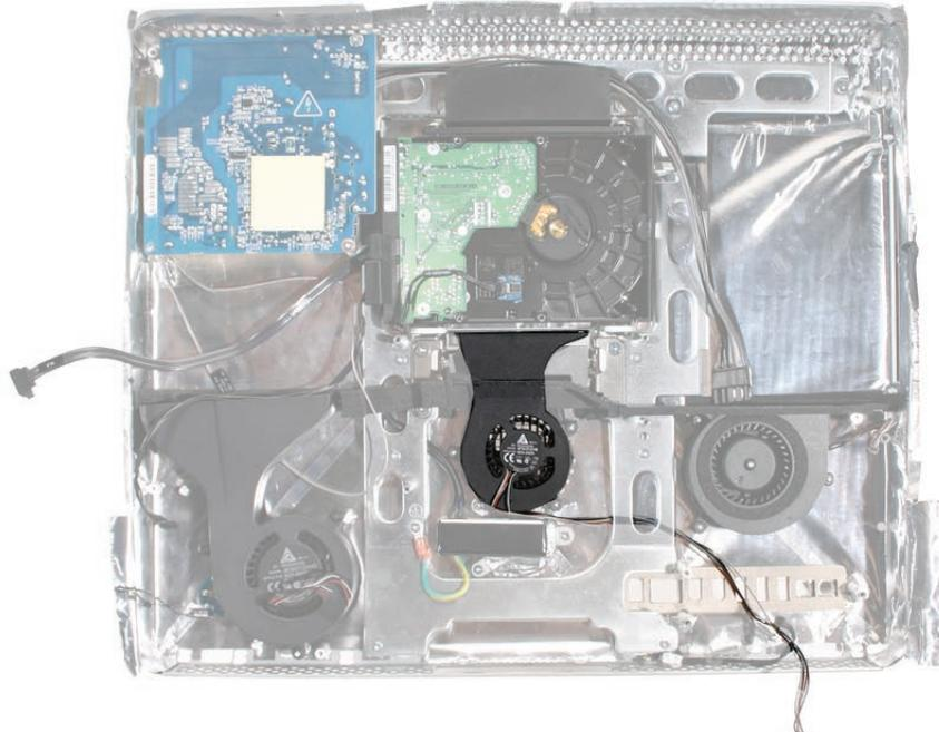
**Note:** This hard drive fan photo is of the iMac (17-inch Mid 2006), however the hard drive fan is in the same location on the iMac (17-inch Late 2006). The hard drive fan cable is routed differently on the iMac (17-inch Late 2006) model. Refer to the next page for a photograph.
