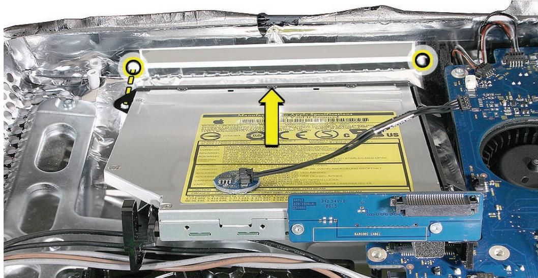
Push down on the black mounting bracket to lock the optical drive securely into place on the chassis.
