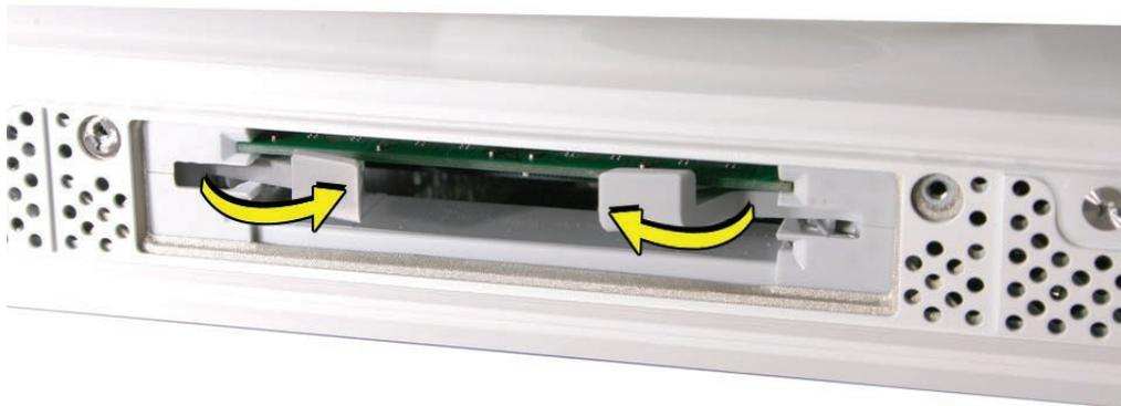
4. Replace the access door on the memory compartment.
