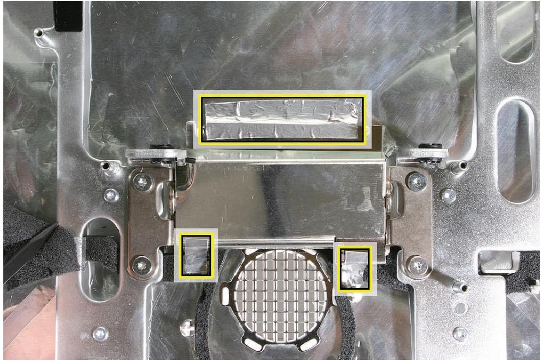
2. Remove the metal clutch cover.
