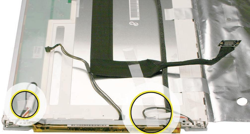
2. Using a flat-blade screwdriver as shown, pry up the inverter to remove it from inside the display panel mounting bracket.
