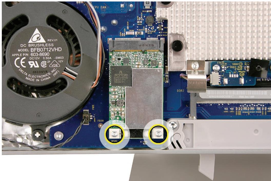
3. The card will spring up when the screws are removed. Grab the card from the connector end and pull the card from the socket on the logic board.
