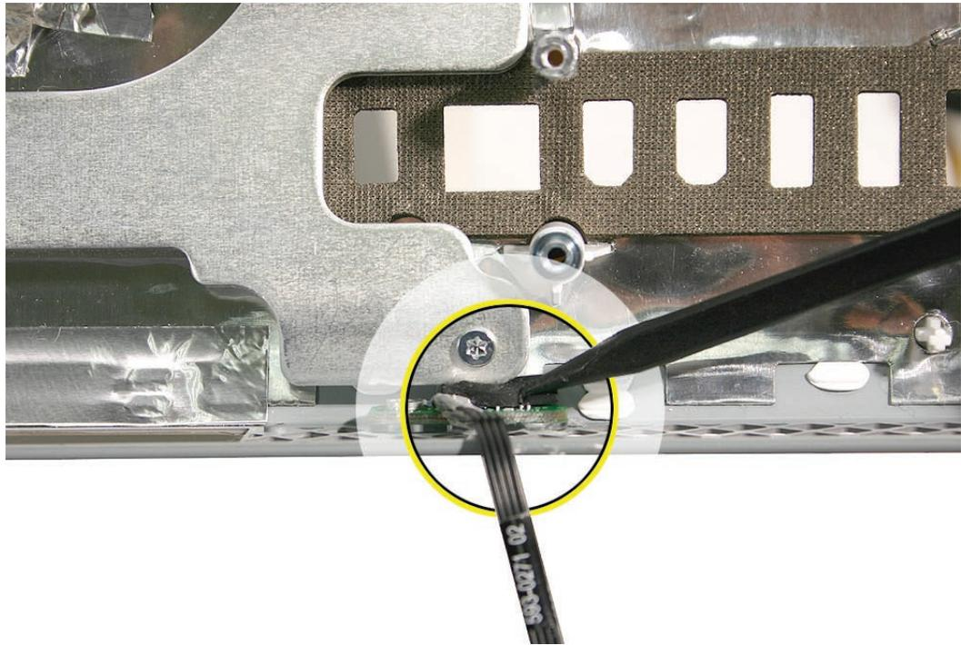
2. With a black stick, pry the ambient light sensor board from the frame.
