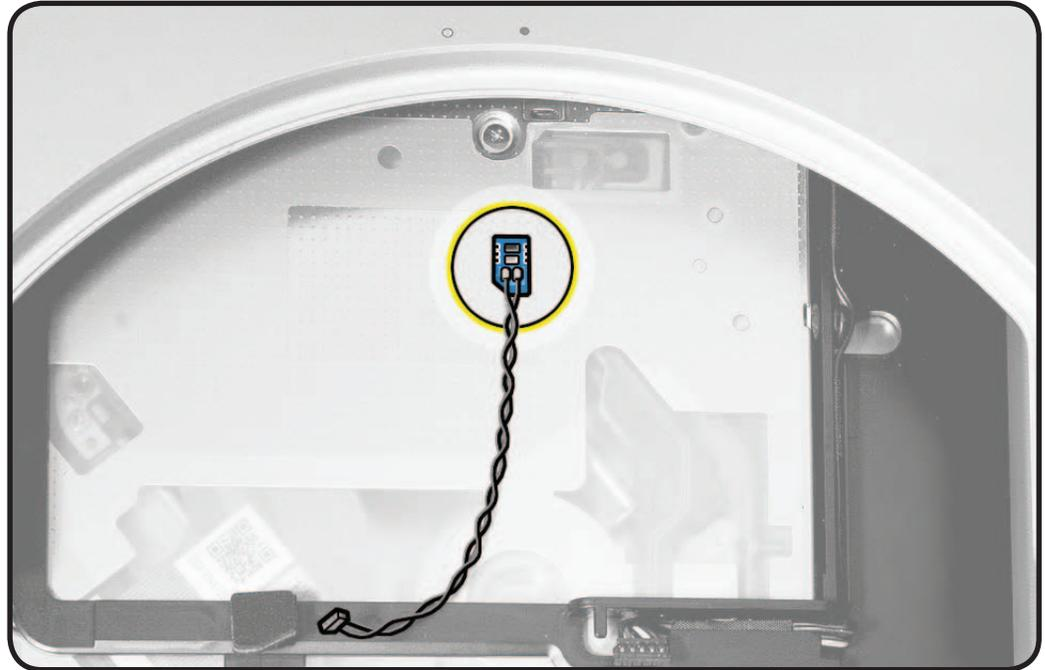
2. Secure the sensor and cable with tape, as shown here.
