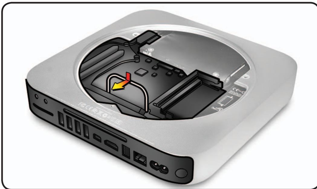
**9** Disconnect the power cable. Wiggle it out from its logic board socket. Tweezers may be helpful.
