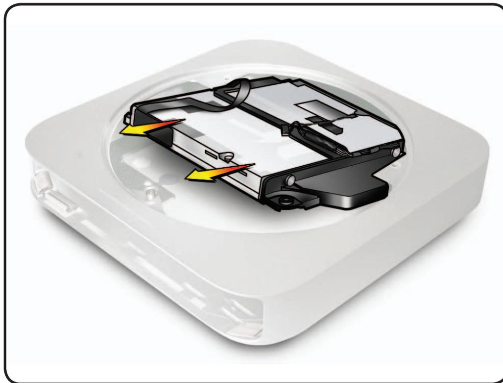
**3** Remove 4 T8 screws in the drive carrier:
