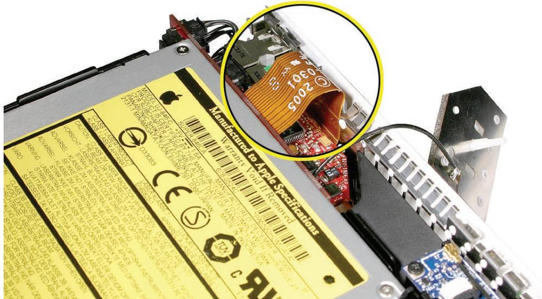
2. Disconnect the Bluetooth antenna from the Bluetooth board.
