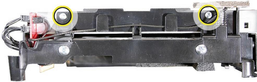
2. Remove the other two optical drive screws.
