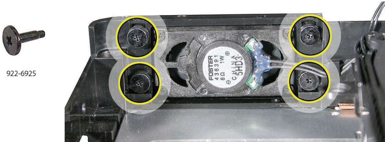
2. Route the speaker cable along the cable channel. Connect the 2-pin speaker cable to the 2-pin connector on the hidden side (see the next photo) of interconnect board.
