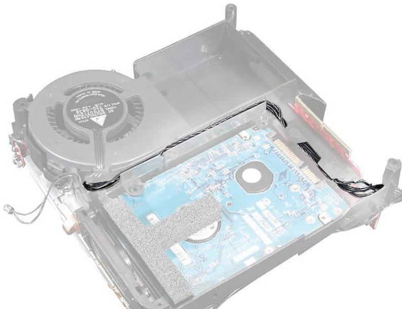
3. Flip the internal frame over and route the cable through the internal frame as shown below. Replace the screw on the IR board.
