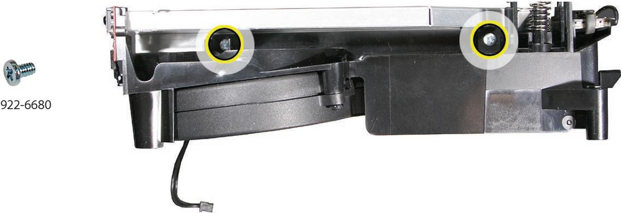
5. Replace the two remaining optical drive screws.
