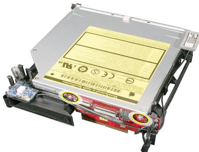
4. Replace the optical drive screws on one side, then rotate the internal frame 180 degrees.
