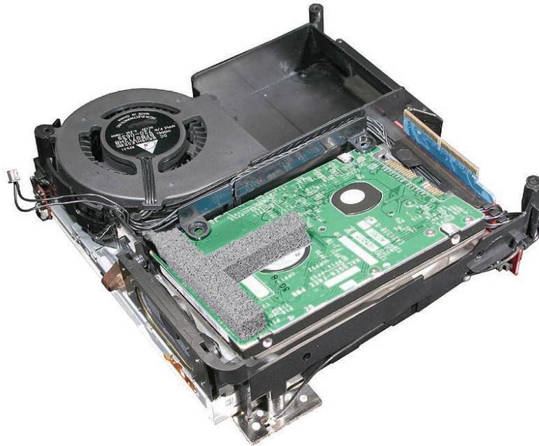
2. Replace the four hard drive screws.
