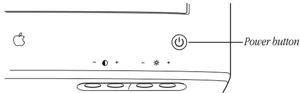
The monitor's green power indicator light goes on. (It may turn amber until your computer comes on.) If the green light does not go on, press the monitor's power button again. If this doesn't work, shut down and unplug your computer and make sure you've connected the monitor to your computer properly (see "Connecting the Display to Your Computer" on page 9).
