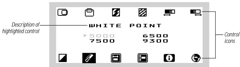
**Note:** The On-Screen Display disappears after approximately 10 seconds if you haven't pressed the OSD navigation buttons or OSD adjustment buttons.
