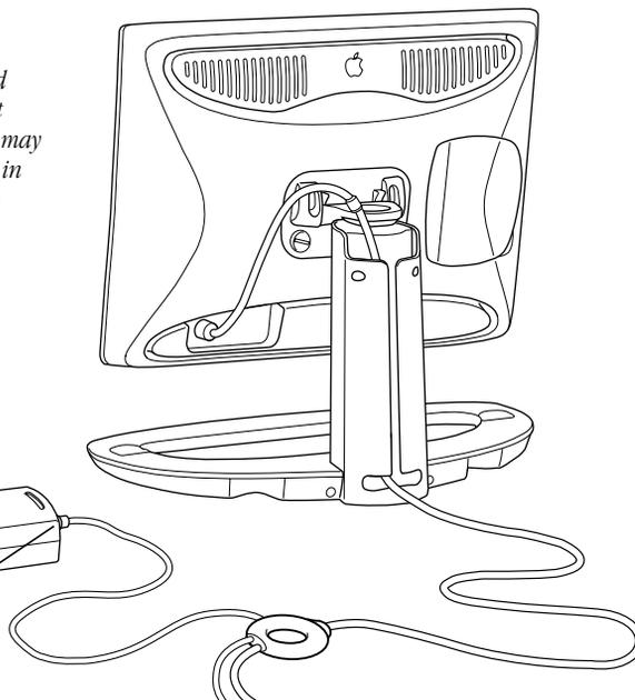
**Step 3: Plug In the display's DVI and USB connectors.**
