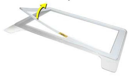
**Replacement Note:** When reassembling the bezel and inner bezel, make sure to snap each bezel clip together.
