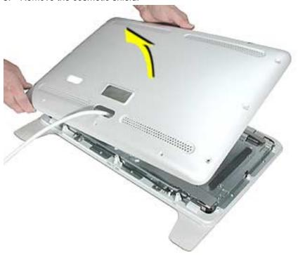
**Replacement Note:** Verify that the rear cosmetic shield and the clear plastic rear cover are free of dust, fingerprints and foreign matter before reassembling.
