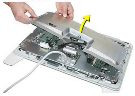
**Replacement Note:** Verify that the EMI gaskets are on the replacement shield. If not, transfer them to the replacement shield from the shield being replaced.
