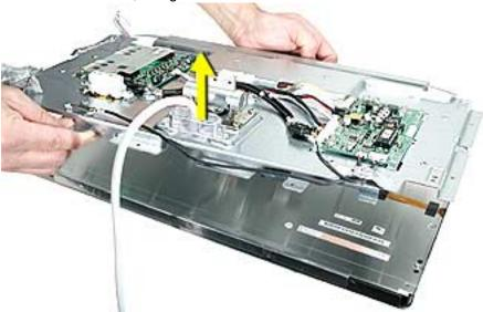
Replacement Note: Be careful not to catch or pinch the backlight bulb wires.
