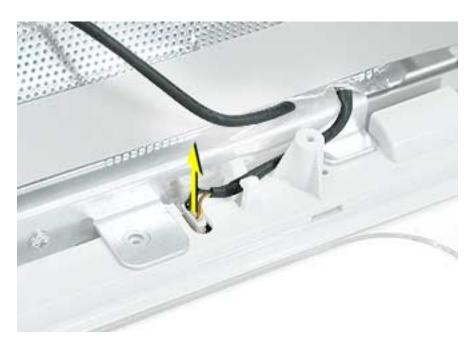
3. Carefully separate the wire clips enough to remove the wires.
