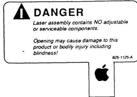
**Safety Labels:** (Scanner unit) Warn against direct exposure to laser beam.
