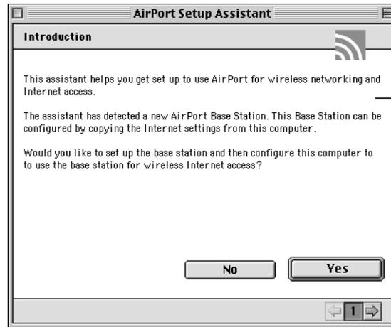
*The AirPort Setup Assistant screen that appears if a new AirPort Base Station is detected and the computer has never been set up to use AirPort. A different screen will appear if there are other networks in range or the computer has already been set up to use AirPort.*
