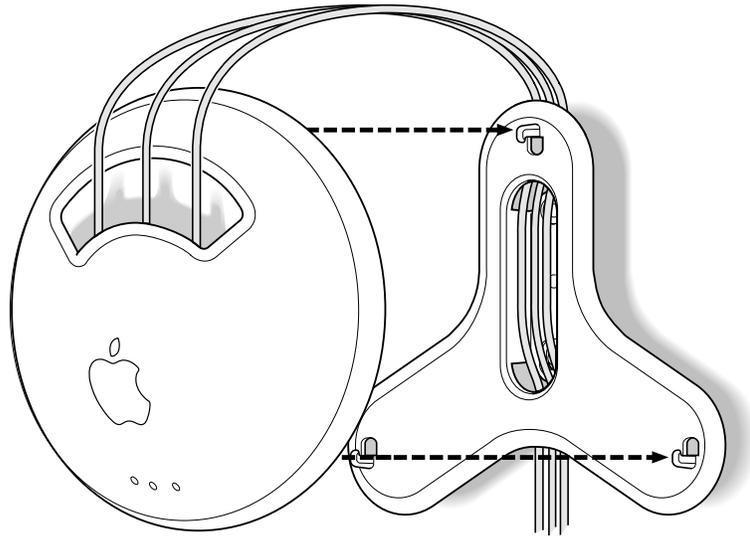
**Note:** The mounting bracket has enough space so that three cables (power, phone, and Ethernet) can be routed through it as shown in the illustration above, even though in most cases only two cables are used.
